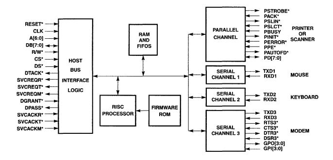
Figure 1-1. Workstation: Printer, Keyboard, Mouse, and Modem Ports
