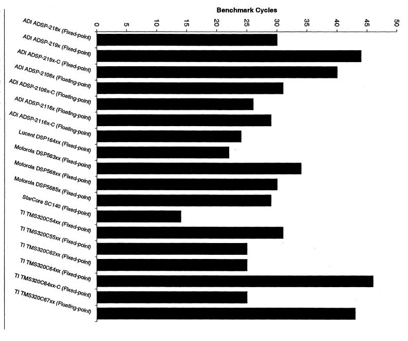
Figure 8.1-3. Total Cycles for Complex Block FIR
