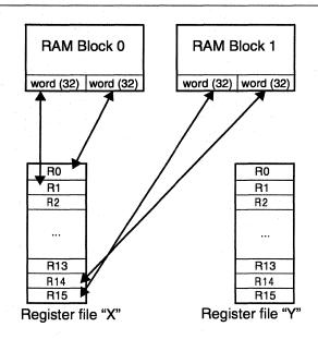
a. SISD mode, addressing a 64-bit long word in each of the two RAM blocks and specifying R0 and R14 as sources or destinations.
