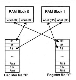
b. SIMD mode, addressing a 32-bit word in each of the two RAM blocks and specifying R0 and R2 as sources or destinations.
