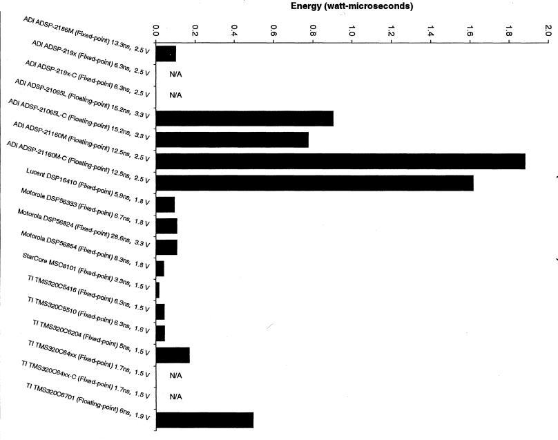
Figure 8.4-5. Energy Consumption for Two-Biquad IIR (Lower is Better)
