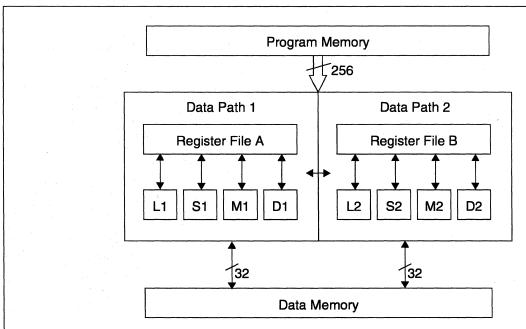
FIGURE 7.15-2. TMS320C62xx data paths. Each data path includes four execution units (L, S, M, and D), described in the text. The arrow between the data paths denotes the cross paths that allow each data path to access the register file of the other data path.
