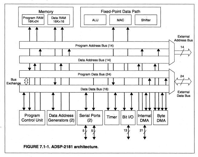
The single accumulator is a limitation of the ADSP-21xx data path. It makes the processor poorly suited for arithmetic using complex numbers, for example. While the shadow register set provides a second accumulator, accessing it requires exchanging all arithmetic registers with their shadow registers. Thus, the shadow registers are more useful for context switching than as additional arithmetic registers for use within a single algorithm.
