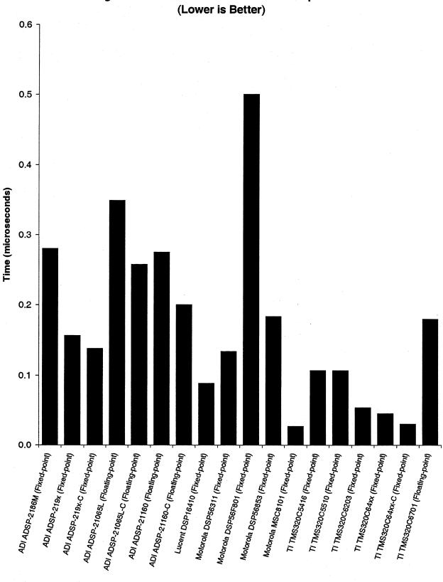
Figure 8.2-5. Execution Time for Two-Biquad IIR
