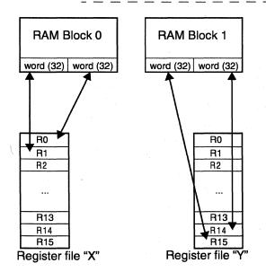
c. SIMD mode, addressing a 64-bit long word in each of the two RAM blocks and specifying R0 in register file "X" and R14 in register file "Y" as sources or destinations.
