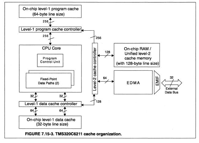
twice the width of the bus between the level-1 data cache and the level-2 cache, two copy operations are required between the level-2 and level-1 data cache. Each copy operation takes 2 cycles to complete. Hence, a latency of four cycles is required to update an entire level-1 data cache line.
