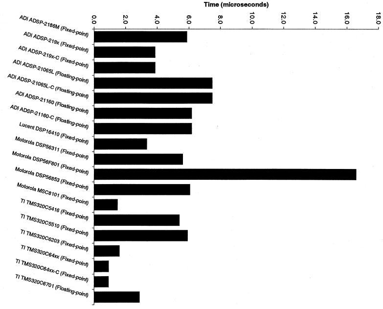
Figure 8.2-10. Execution Time for 256-Point FFT (Lower is Better)
