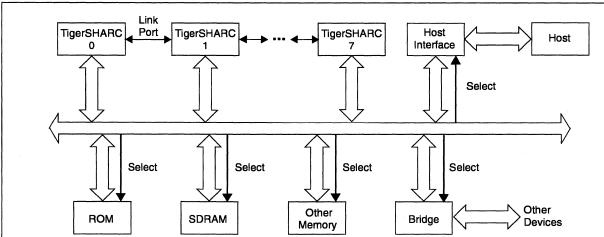
FIGURE 7.5-2. ADSP-TS0xx multiprocessing configuration. The link ports may connect TigerSHARCs 0 through 7 in any configuration, not just the simple configuration shown here.
