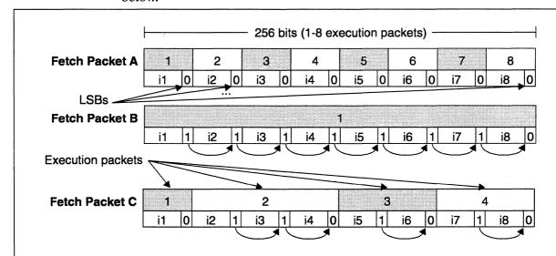
FIGURE 7.15-4. Example fetch packets A, B, and C. Fetch packet A consists of eight instructions (i1-i8), each forming its own execution packet indicated by the LSB of each instruction. Fetch packet B contains one execution packet consisting of eight instructions. Fetch packet C contains four execution packets, each consisting of one to three instructions. Execution times for fetch packets A, B, and C are eight, one, and four cycles, respectively.
