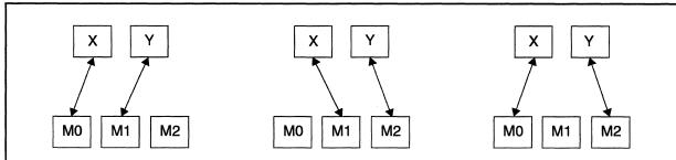
FIGURE 7.5-3. SIMD transfers between fixed/floating-point data path registers and on-chip memory. M0, M1, and M2 are the three internal memory banks shown in Figure 7.5-1.
