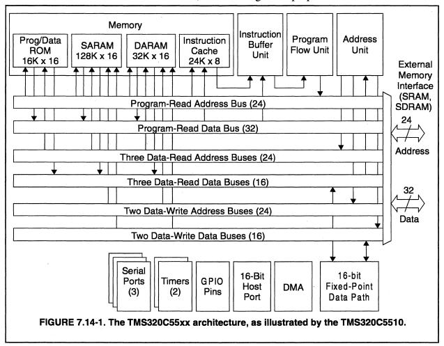
pendent from the processor's three address generators and can be used in parallel with the main data path. The TMS320C55xx (like the TMS320C54xx) includes eight 16-bit "auxiliary registers," AR0-AR7. These registers are primarily used (with 7-bit extension registers) as address registers but, unlike on the TMS320C54xx, they can also be used as general-purpose registers in some cases.
