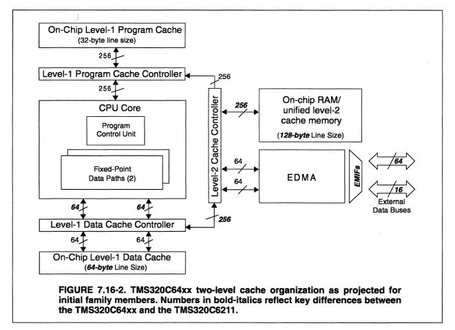
gle-ported 256-bit wide memory bank. The line size of the TMS320C64xx level-1 instruction cache is 32 bytes (it holds an entire fetch packet). The level-1 instruction cache of the initial TMS320C64xx can store up to 4K 32-bit instructions.
