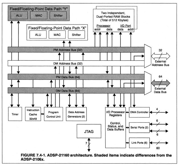
cutes instructions in a fashion similar to an ADSP-2106x processor. The SIMD mode enables data path "Y," which then executes the same instruction as data path "X," but on the register file associated with data path "Y".
