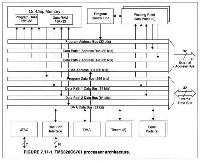
32-bit single-precision and 64-bit double-precision floating-point arithmetic. Since TMS320C67xx general-purpose registers are 32 bits wide, 64-bit floating-point values are supported by pairing an even-numbered register with the next higher odd-numbered register. For example, registers A2 and A3 can be paired to hold a single 64-bit floating-point value.
