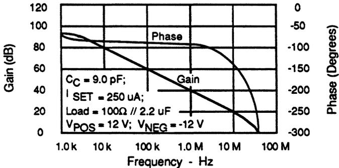
Figure 9. Open Loop Gain and Phase vs Frequency
