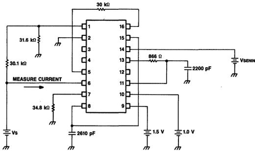
Figure 1. Power Supply Current Test Circuit
