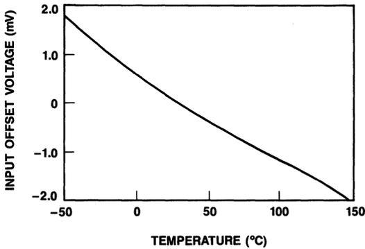
Figure 17. Typical Darlington Input Offset Voltage vs. Temperature
