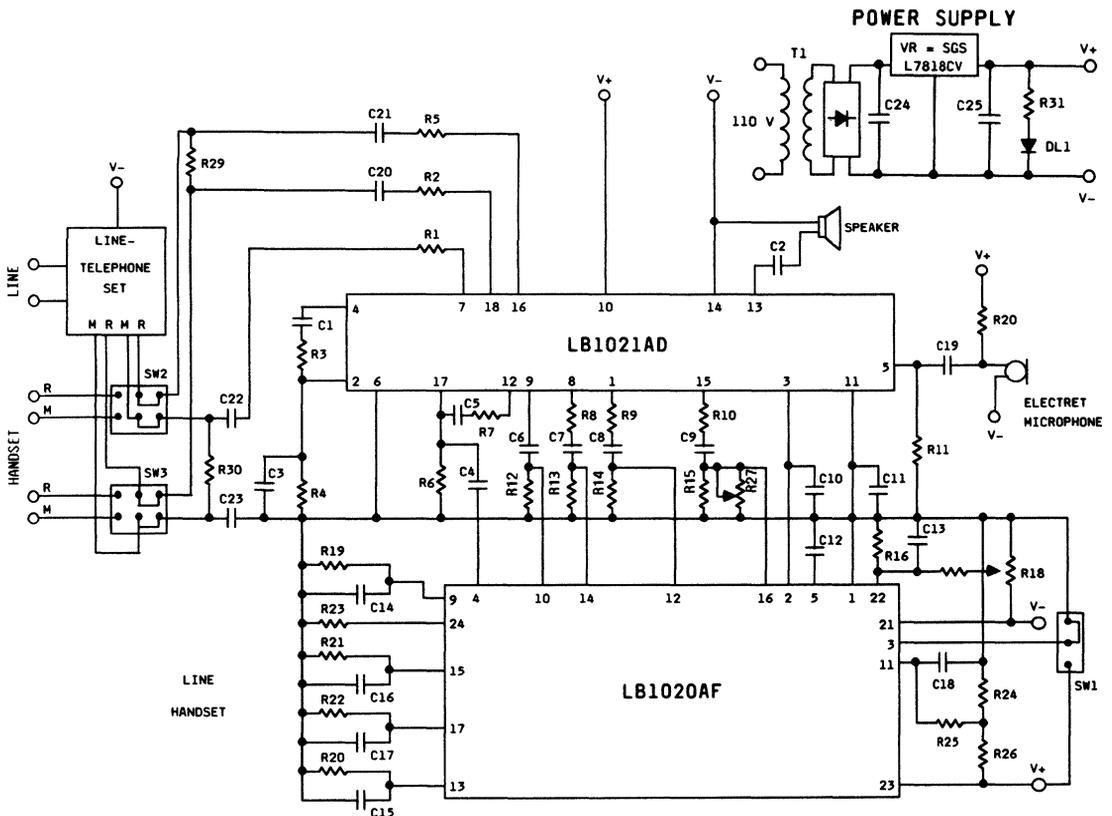
**Figure 43. Typical Speakerphone Telephone-Coupled Application**
