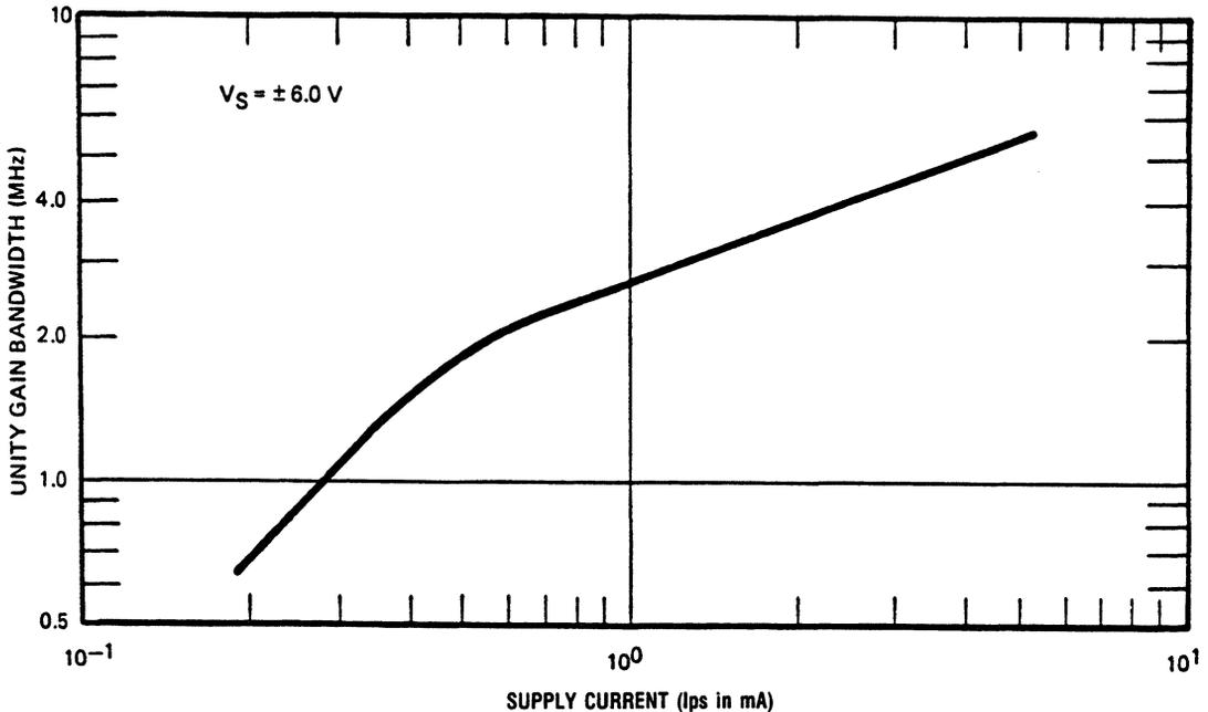
Figure 14. Supply Current/Unity Bandwidth Characteristic
