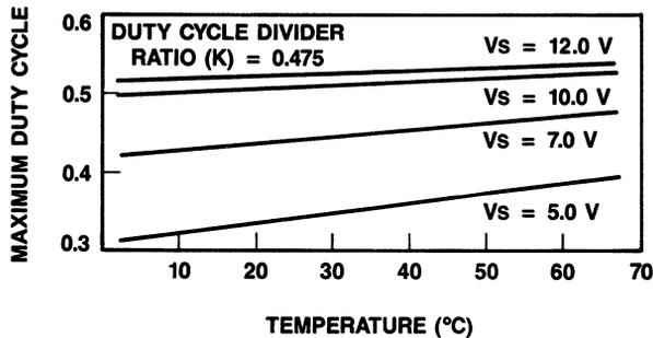
Figure 8. Maximum Duty Cycle as a Function of Temperature for Various Supply Voltages
