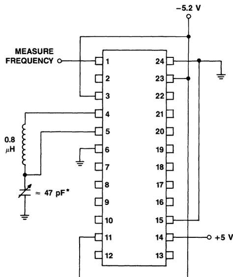
\* Capacitor should be adjusted so the resonant frequency of the tank circuit (including Lead length, etc.) is nominally 20 MHz.
