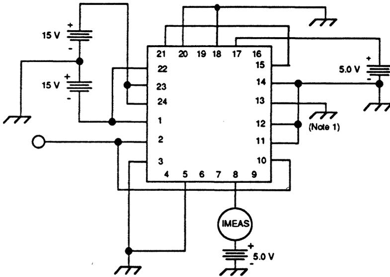
Figure 10. Logic Input Current Test Circuit
