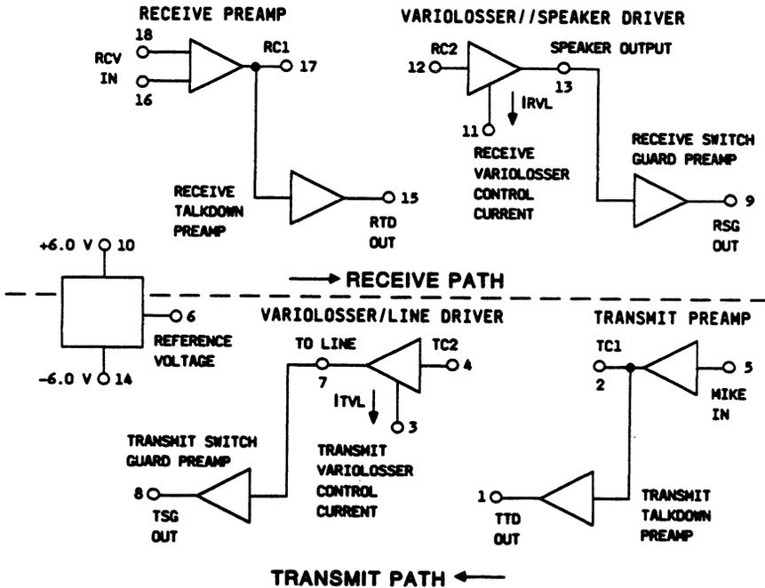
Figure 5. LB1021AD Power Conditioner—Amplifier Block Diagram
