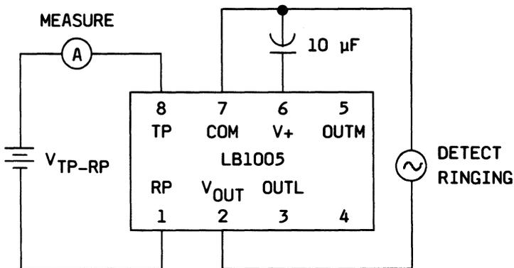
Figure 2. Test Circuit (TP and RP Currents, No Load)
