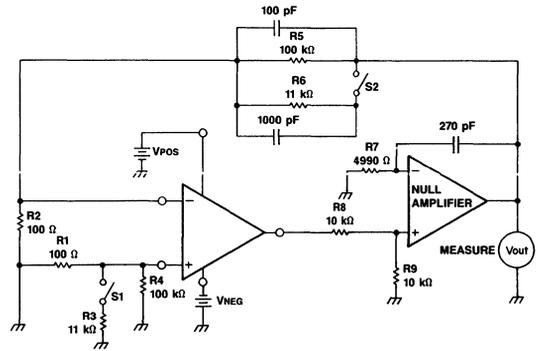
Figure 2. Input Offset Voltage ( $V_{io}$ ), Input Bias Current ( $I_{ib}$ ), and Input Offset Current ( $I_{io}$ ) Test Circuit
