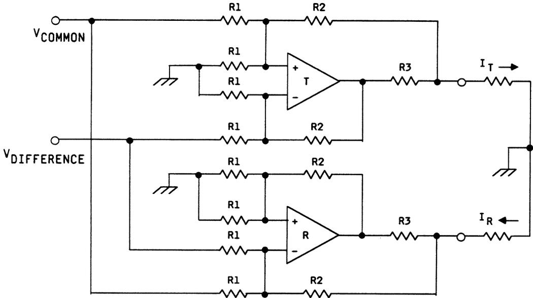
Figure 7. Simplified Line Feed Operation (Power-Supply Connections Not Shown)
