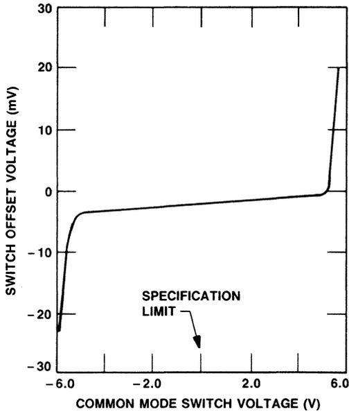
Figure 7. Typical Offset Voltage vs. Common-mode Voltage
