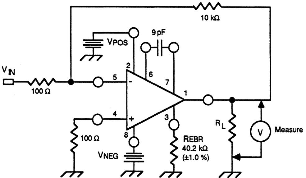
Figure 4. Output Voltage Swing Test Circuit
