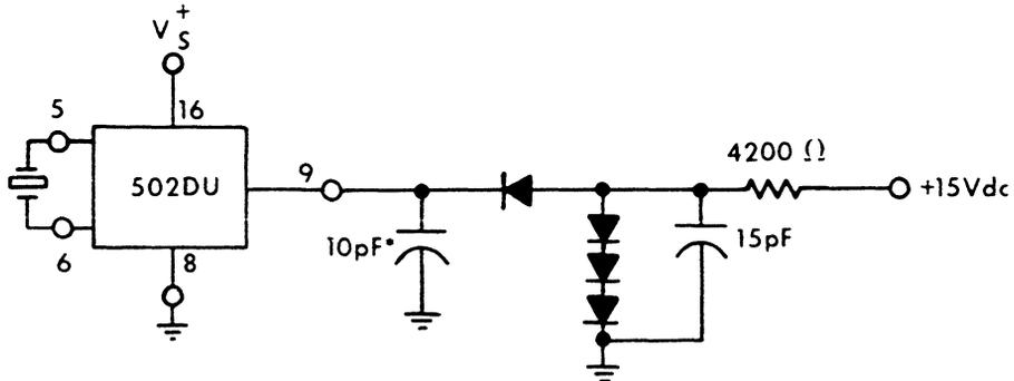
\*Includes probe, trigger circuit, and fixture capacitance. All diodes shall be 458E or equivalent.
