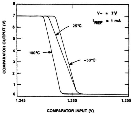
Figure 10. Typical Comparator DC Transfer Characteristics vs Temperature
