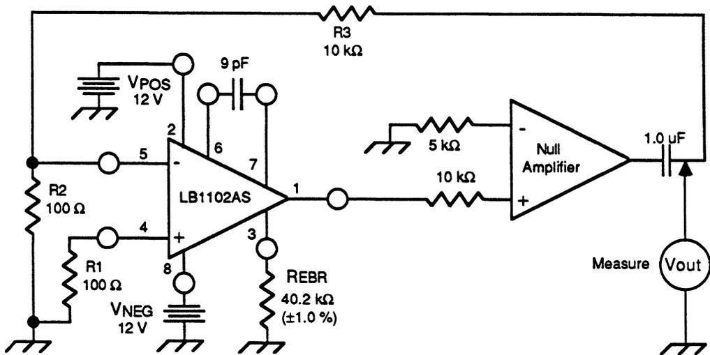
$$\text{Input Offset Voltage} = \frac{V_{\text{out}}}{K}; \text{ where } K = \frac{R_2 + R_3}{R_2};$$
