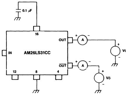
Figure 5. Output Current (Power OFF)
