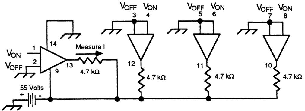
Figure 5. Fail-Safe Output Leakage Current Test Circuit
