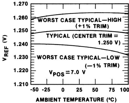
Figure 3. Precision Low-Voltage Reference Temperature Characteristics
