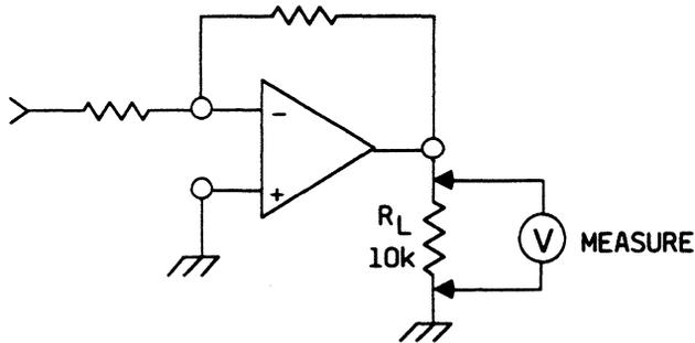
Figure 1. Test Circuit, Output Voltage Swing
