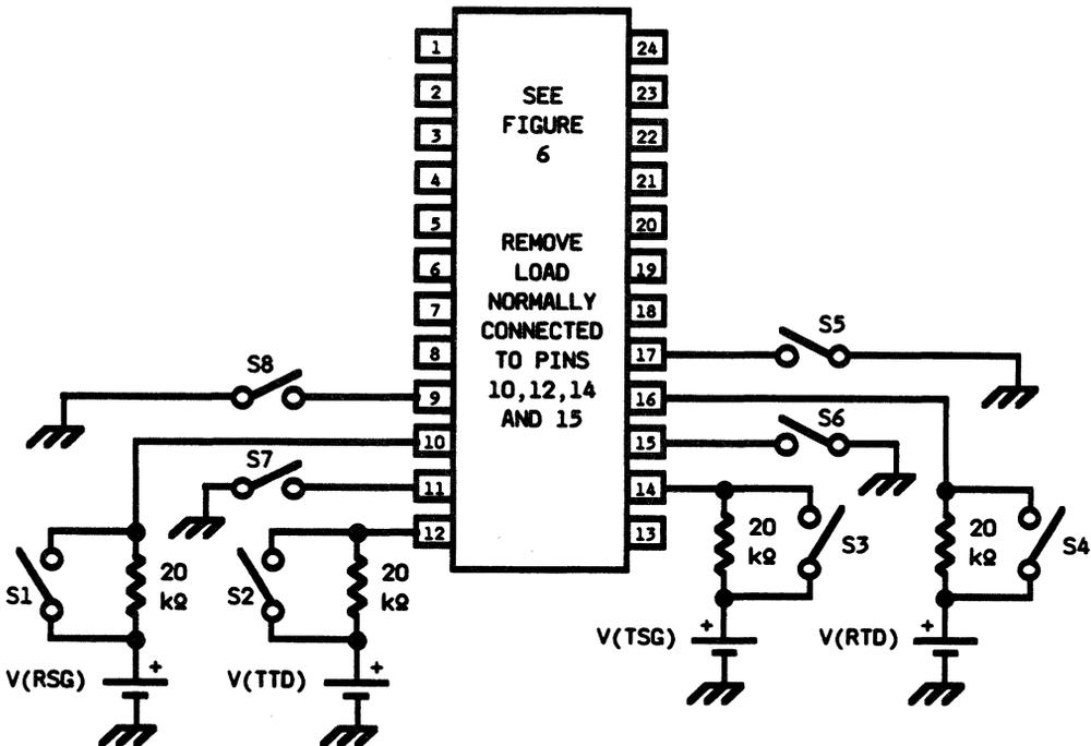
Figure 17. LB1020AF Test Circuit
