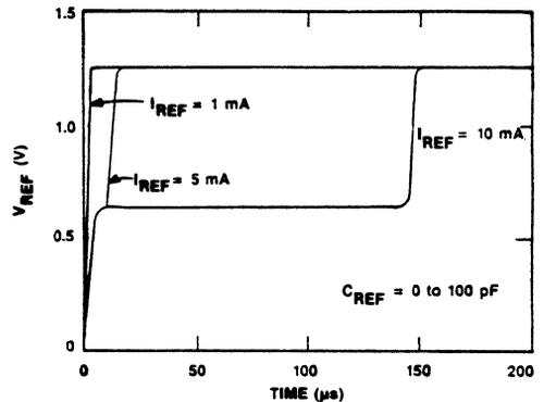
Figure 6. Precision Low-Voltage Reference Transient Start-Up Time
