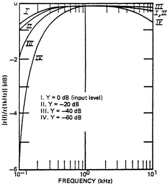
Figure 12. Frequency Response of the Compressor
