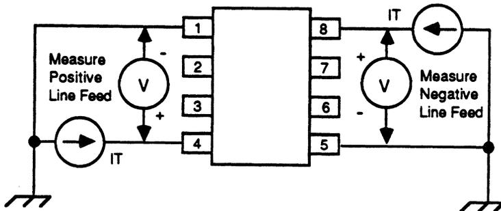
Figure 7. Line/Supply Voltage, Test Circuit
