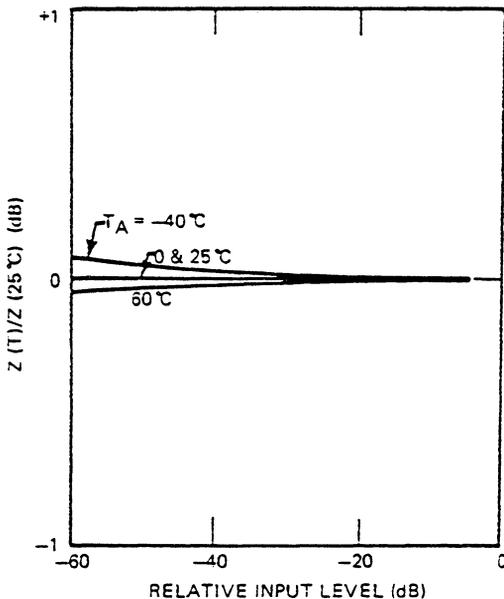
Figure 10. Temperature Stability of the Compressor
