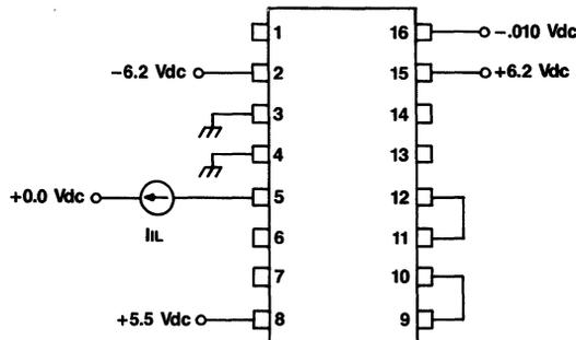
Figure 6. Input Forward Current,  $V(4) = 0$
