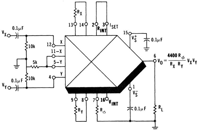
**Figure 4. Internal Reference with Internal Resistor**
