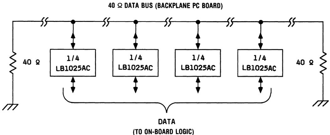
Figure 7. LB1025AC Quad Bus Transceiver Application Diagram
