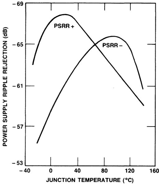
Figure 11. Typical Power Supply Ripple Rejection vs. Temperature
