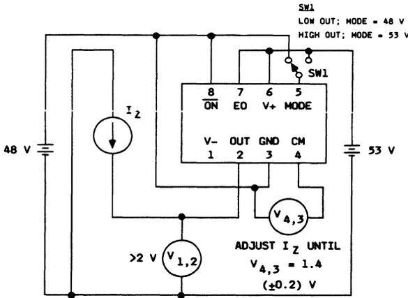
Figure 8. Output Current Threshold Test
