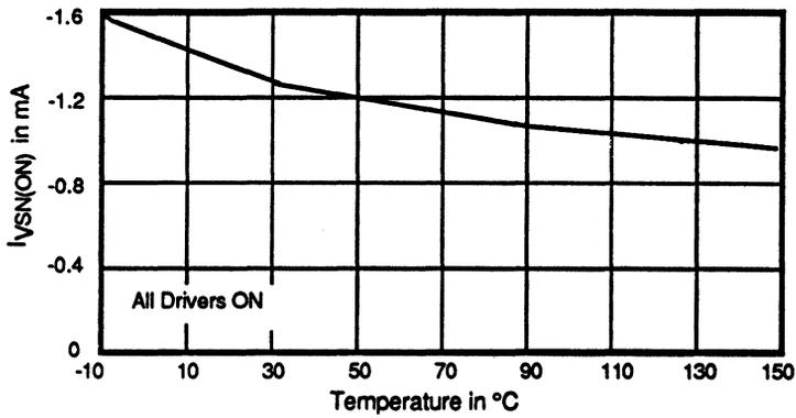
Figure 13. Typical Supply Current (I<sub>VSN(ON)</sub>) vs Temperature
