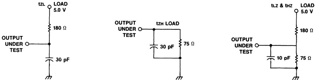
Figure 13. Associated ENABLE,  $\overline{\text{ENABLE}}$  Loading Diagrams
