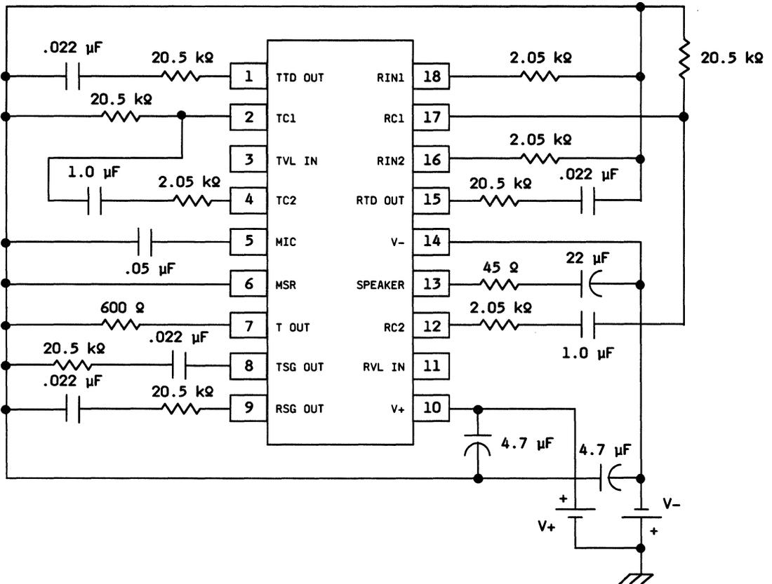
Figure 21. LB1021AD Test Circuit
