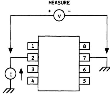
Figure 4. On/Forward Voltage Tests
