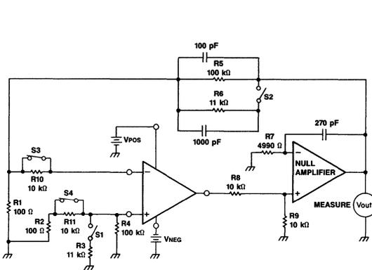
Figure 3. Input Bias and Input Offset Current Test Circuit
