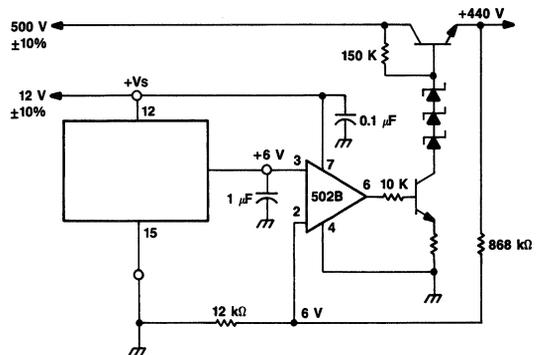
**Figure 11. High-Voltage Application Using the LB1081CC 6 V Reference**
