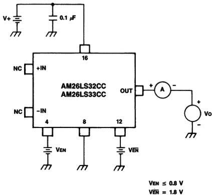
Figure 7. Off-State Output Current (High Z)
