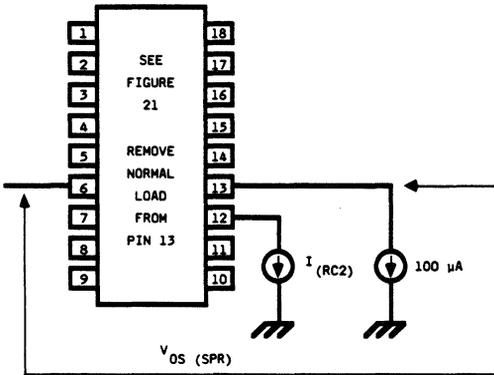
Figure 28. LB1021AD Test Circuit
