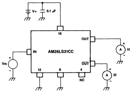
Figure 6. Output Current (Short Circuit)
