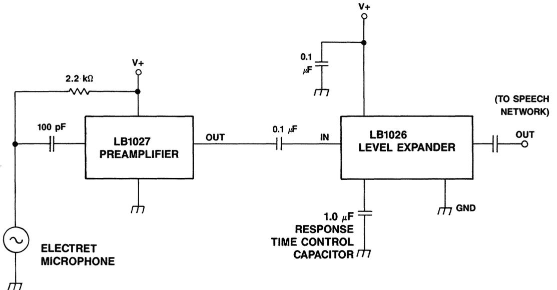
Figure 3. LB1026AA/AB Level Expander Application Diagram
