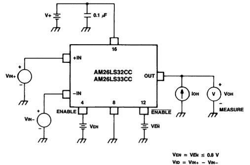
Figure 5. High-Level Output Voltage & Low-Level Output Voltage
