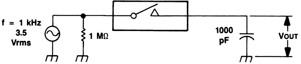
Figure 4. Switch Off Isolation Test Method
