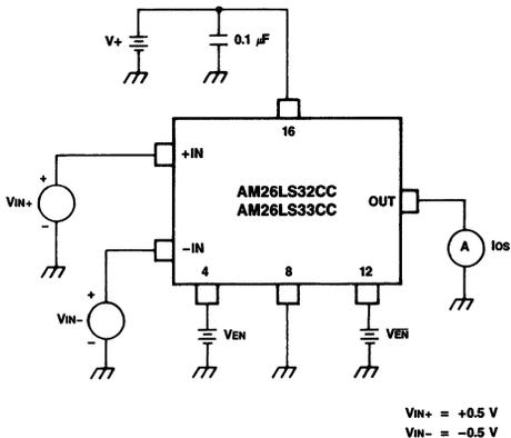
Figure 6. Output Current, Short Circuit
