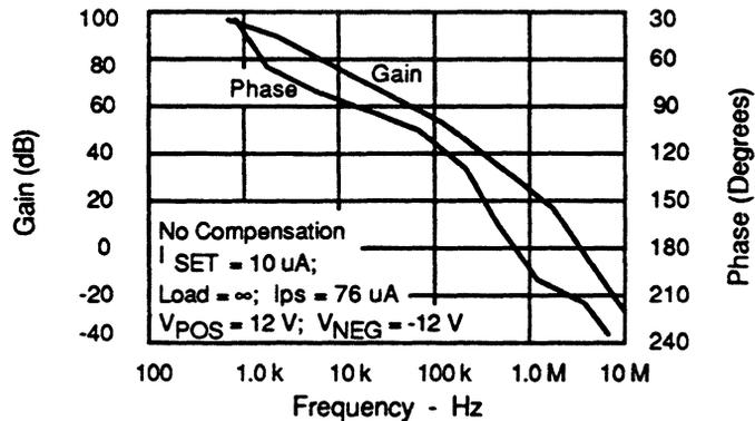
Figure 12. Open Loop Gain and Phase vs Frequency
