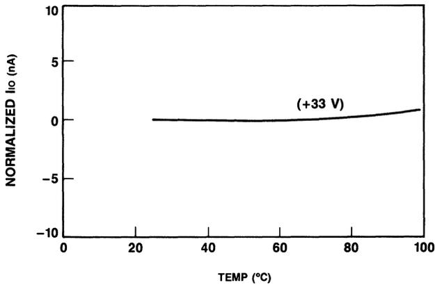
Figure 14. Temperature vs. Input Offset Current (Normalized) at Various Supply Voltages
