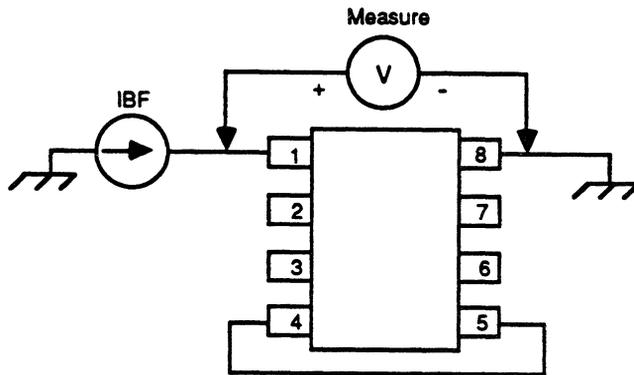
Figure 6. Battery Feed Total Voltage, Test Circuit
