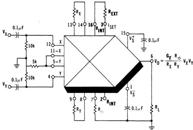
**Figure 5. Internal Reference with External Resistor**
