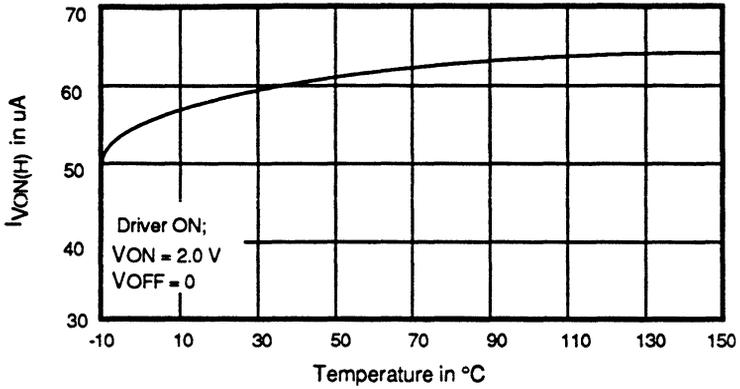
Figure 16. Typical Driver V<sub>ON</sub> Input Current (I<sub>VON(H)</sub>) vs Temperature
