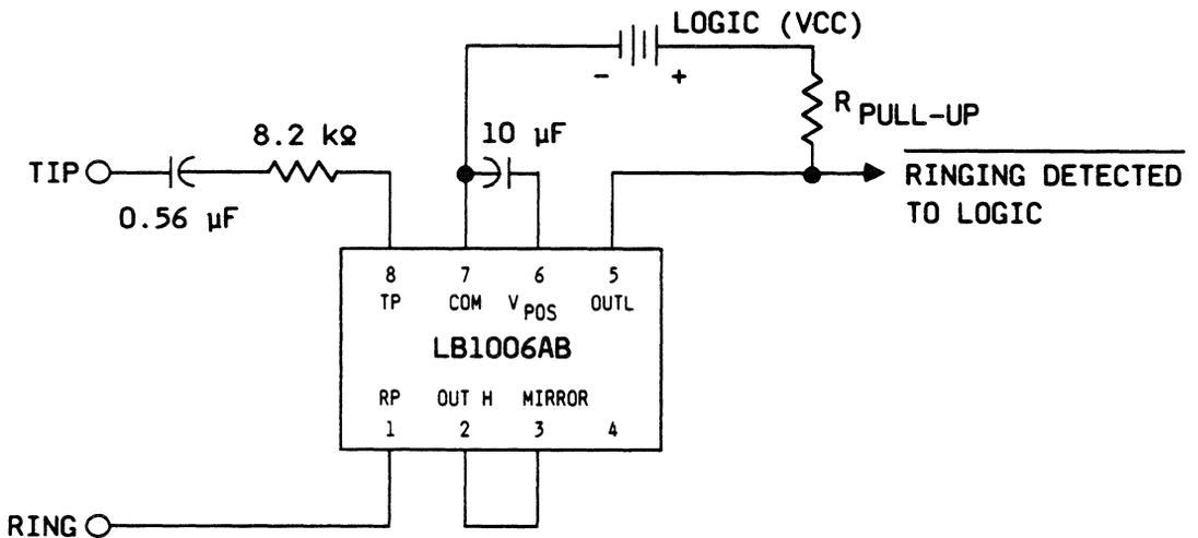
**CAUTION:** Care must be taken when interfacing to a load which is referenced to earth ground (see APPLICATIONS text for further details).
