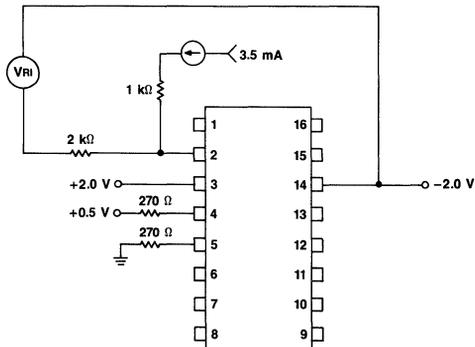
Figure 5. Low-Level Output Voltage (+Vs = +2 V and -Vs = -2 V)
