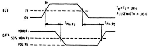
Figure 4. Receiver Timing Waveform
