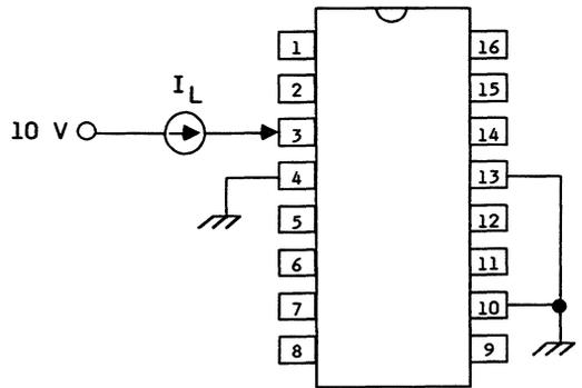
Figure 5. Leakage Current Test Circuit
