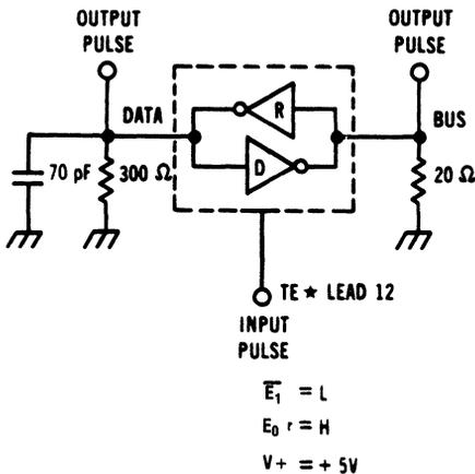
Figure 5.  $\overline{TE}$  to Driver and Receiver Test Circuit
