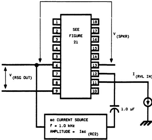
Figure 30. LB1021AD Test Circuit
