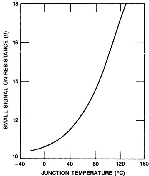
Figure 19. Typical ON Resistance vs. Temperature
