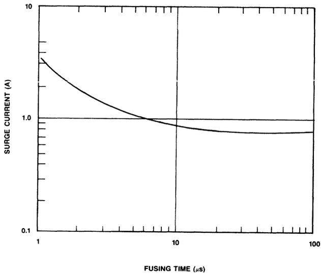
Figure 3. Typical Fusing Characteristics
