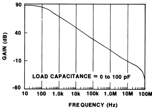
Figure 5. Op-Amp Open-Loop Gain
