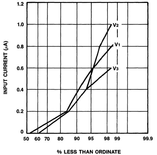
Figure 6. Typical Input Current Distributions
