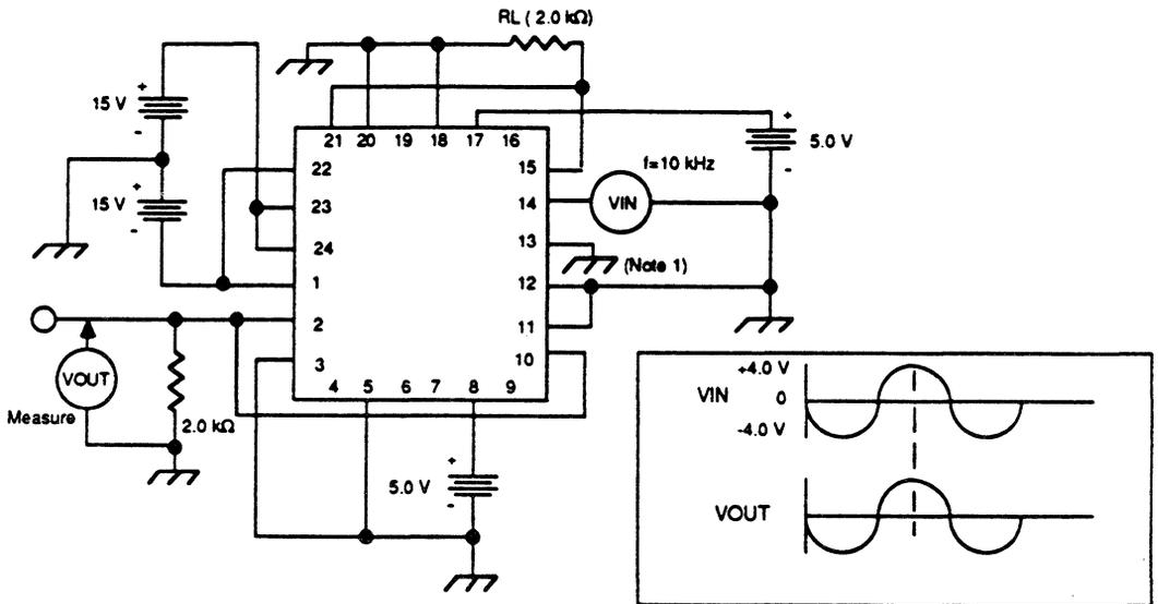
Figure 13. Crosstalk Test Circuit
