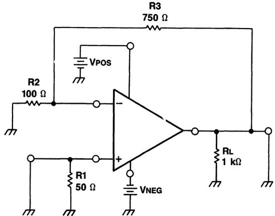
Figure 8. Slew Rate Test Circuit
