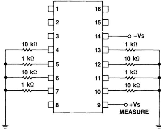
Figure 7. Power Supply Current
