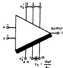
**Figure 13. 1031AC No Offset Null External Compensation**
