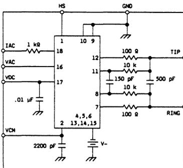
Figure 2. Basic Test Circuit
