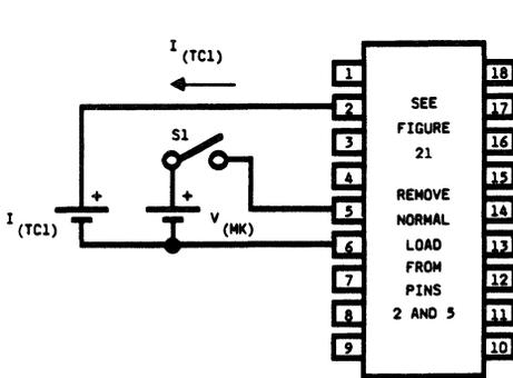
Figure 34. LB1021AD Test Circuit
