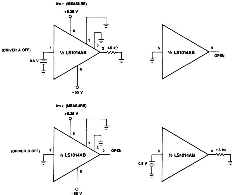
Figure 2. Power Supply, Current Off
