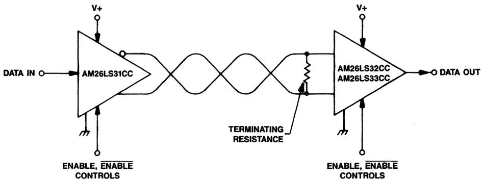
Figure 14. AM26LS31CC Quad Line Driver Application Diagram
