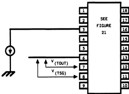
Figure 32. LB1021AD Test Circuit
