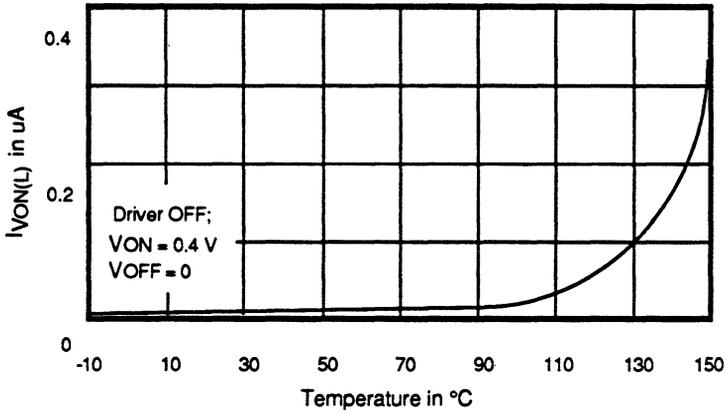
Figure 17. Typical Driver V<sub>ON</sub> Input Current (I<sub>VON(L)</sub>) vs Temperature
