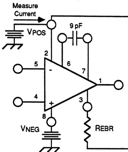
Figure 2. Power Supply Leakage Current
