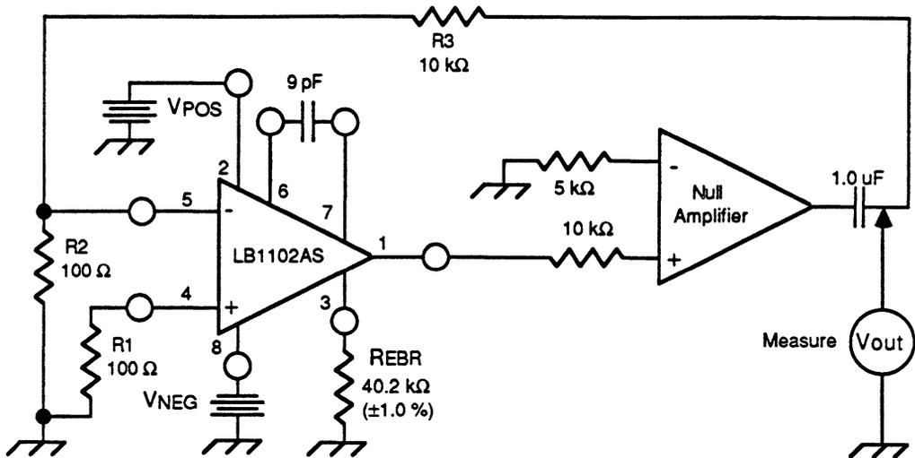
$$\text{PSRR (dB)} = 20 \left[ \text{Log} \frac{\Delta V_{\text{out}}}{K(\Delta V_{\text{supply}})} \right]; \text{ where } K = \frac{R_2 + R_3}{R_2}; \quad \Delta V_{\text{supply}} = 5.0 \text{ volts (Positive and Negative power supplies are simultaneously varied from 12 volts to 7.0 volts.)}$$
