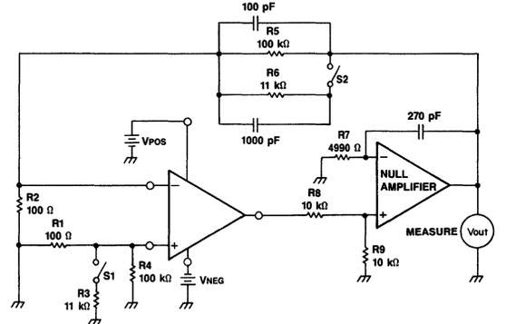
Figure 6. Power Supply Rejection Ratio Test Circuit
