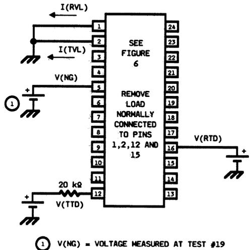
① V(NG) = VOLTAGE MEASURED AT TEST #19
