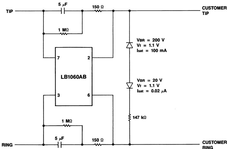
Figure 8. Typical Application Diagram for LB1060AB in Maintenance Termination Unit (MTU)
