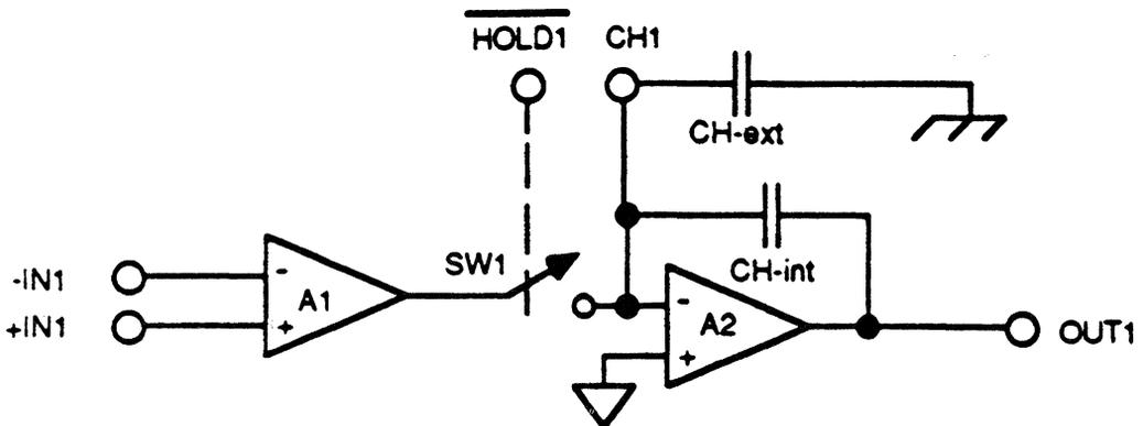
Figure 14. Simplified Functional Operation
