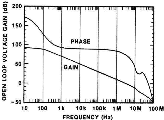
Figure 5. LB1108AD Open-Loop Frequency and Phase Response
