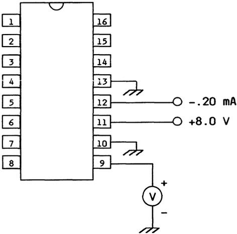
Figure 1. Cutoff Voltage and Collector-Emitter Saturation Voltage Test Circuit
