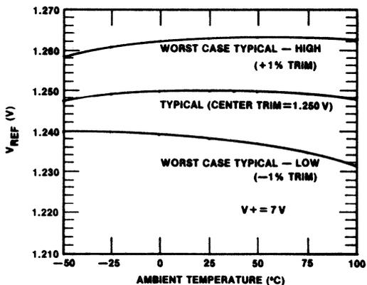
Figure 7. Precision Low-Voltage Reference Temperature Characteristics
