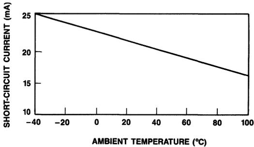
Figure 6. Typical Short-Circuit Current vs. Temperature
