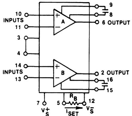
Figure 8. Both Amplifiers Operating, External Bias Resistor, External Frequency Compensation
