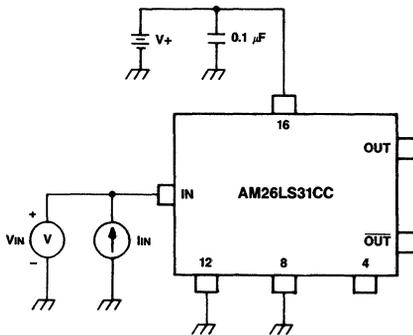
Figure 2. Input Clamp Voltage
