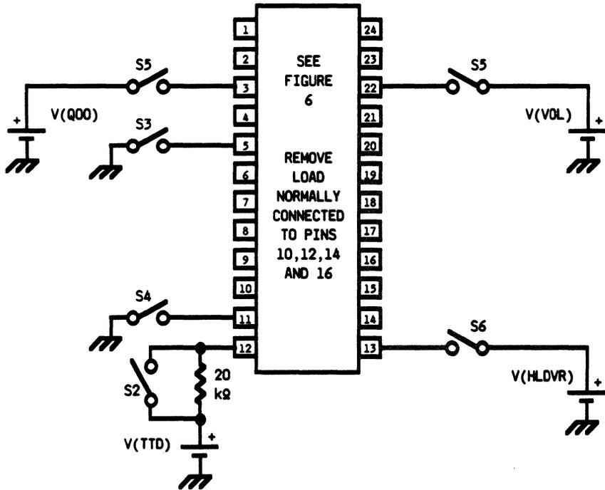
Figure 18. LB1020AF Test Circuit
