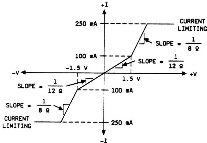
Figure 1. LH1061AB Typical ON Characteristics
