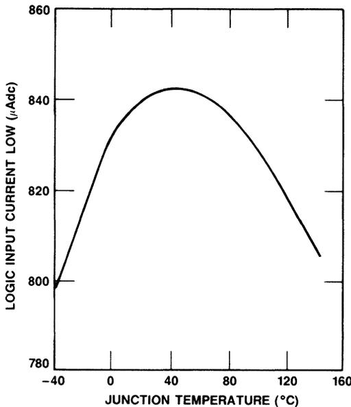
Figure 13. Typical Input Logic Current Low vs. Temperature
