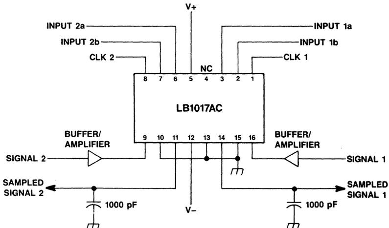
Figure 20. LB1017AC High-Speed Dual Analog Switch Sampling Application
