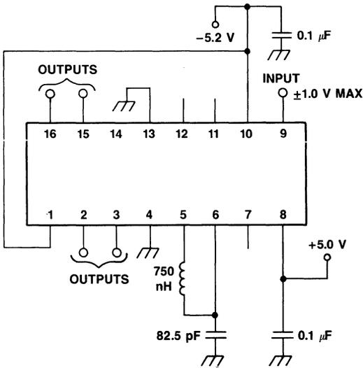
Figure 6. Typical VCO Configuration for Operation at 20 MHz
