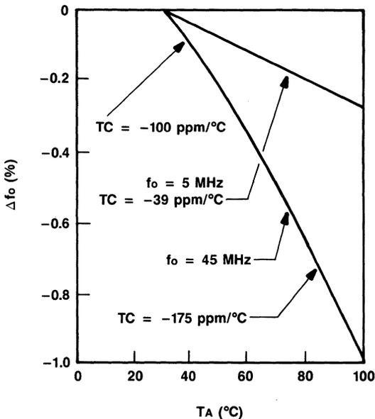
Figure 4. Typical Temperature Coefficient
