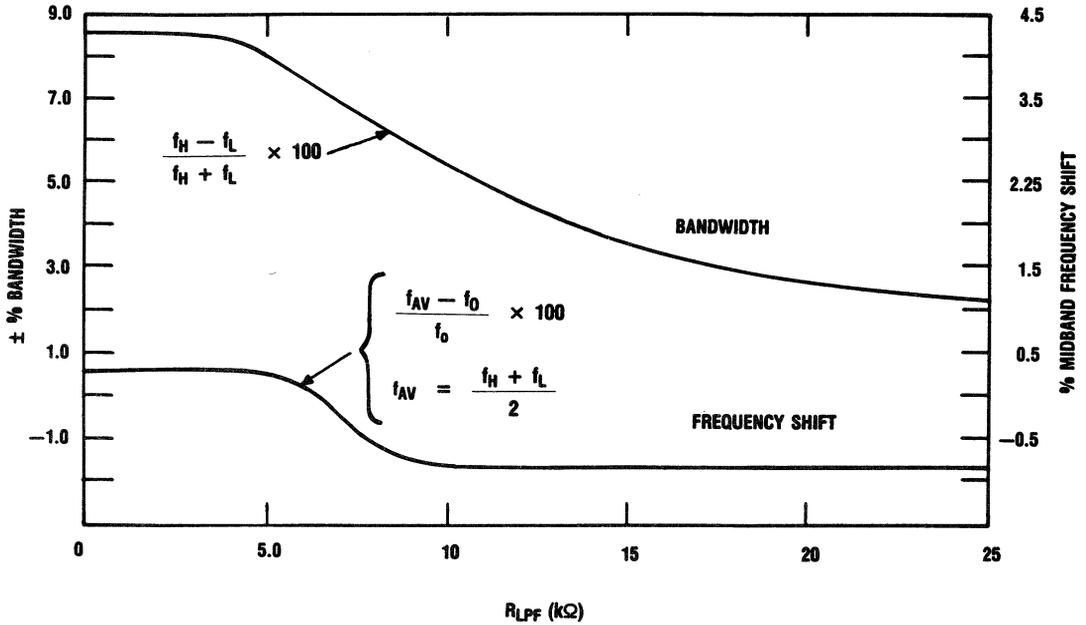
Figure 1. Bandwidth and Midband Frequency Shift vs  $R_{LPF}$
