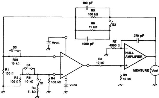
Figure 3. Input Bias and Input Offset Current Test Circuit
