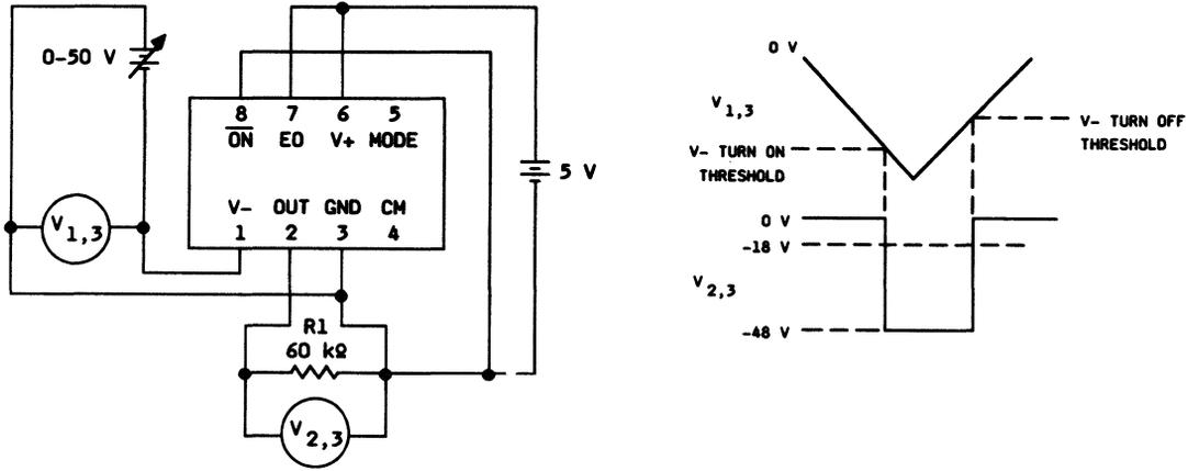
Figure 5. V-Threshold Tests
