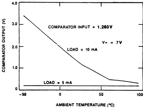
Figure 11. Typical Temperature Characteristics
