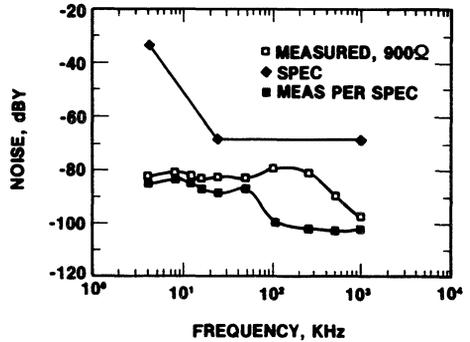
Figure 20(b). Typical Longitudinal Out-of-Band Noise
