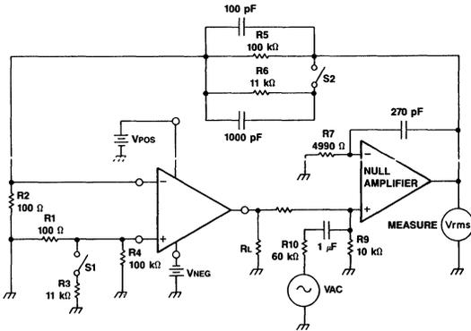
Figure 1. Open Loop Gain Test Circuit
