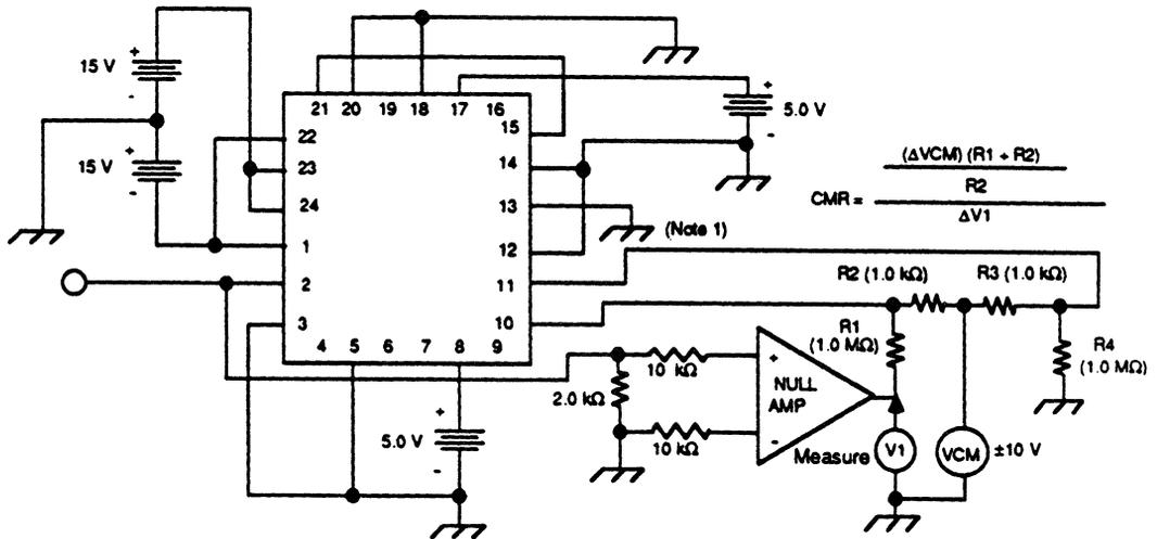
Figure 4. Common Mode Rejection Test Circuit
