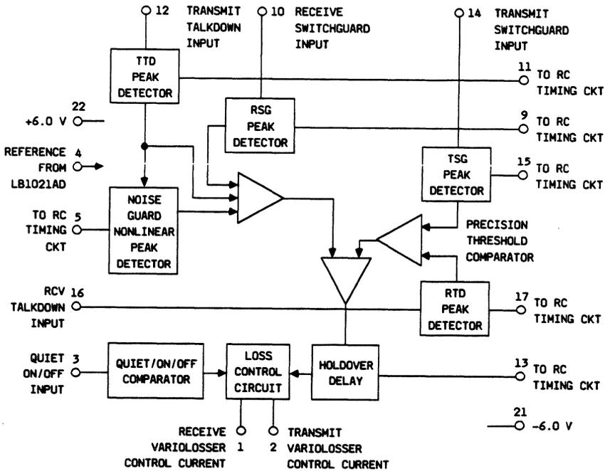
Figure 4. LB1020AF Voice Path Switch Block Diagram
