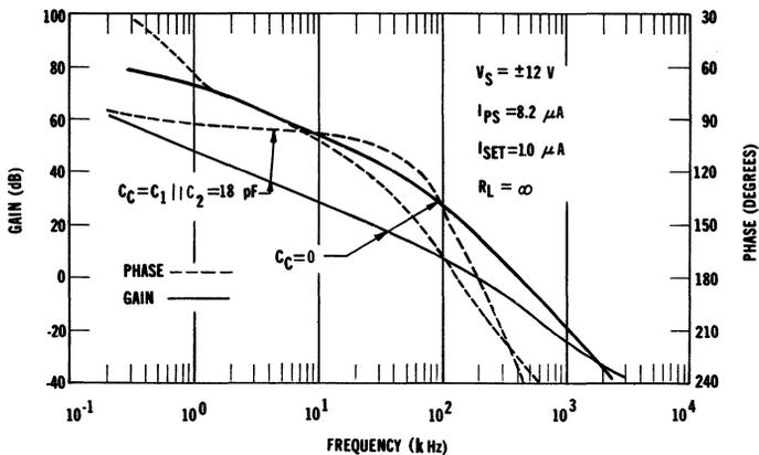
Figure 12. Open-Loop Gain and Phase vs. Frequency
