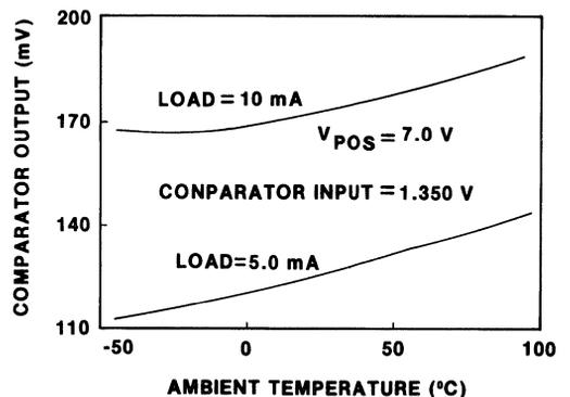
Figure 8. Typical Temperature Characteristics Comparator Output Voltage vs. Comparator Input Overdrive of 100 mV
