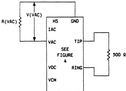
Figure 13. Test Circuit
