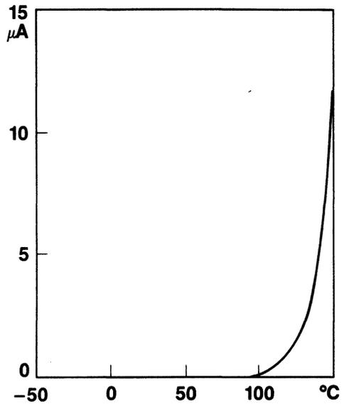
Figure 11. Output Leakage Current vs. Temperature
