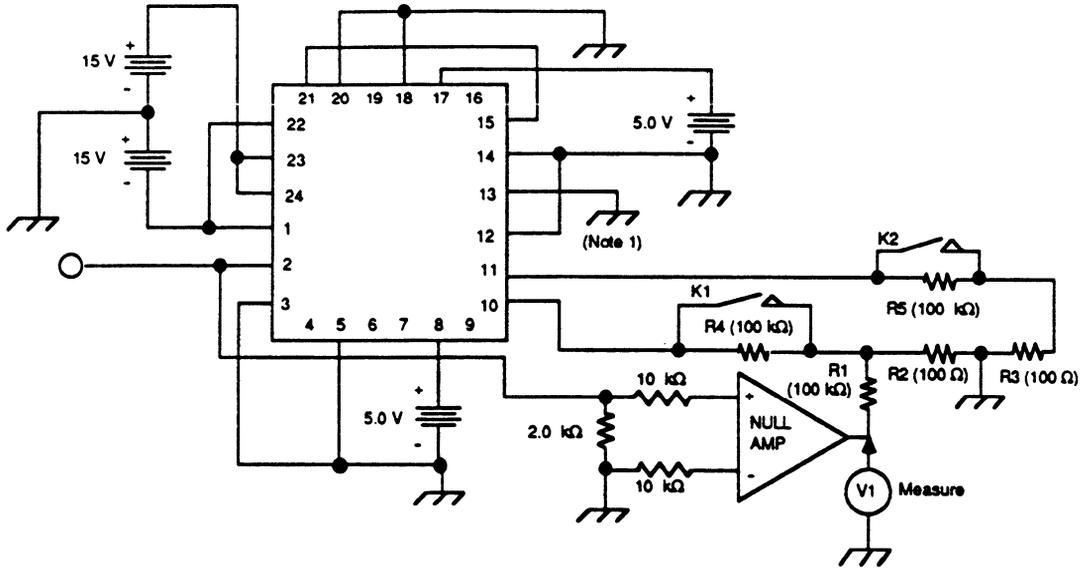
Test Condition      V1 Measurement
