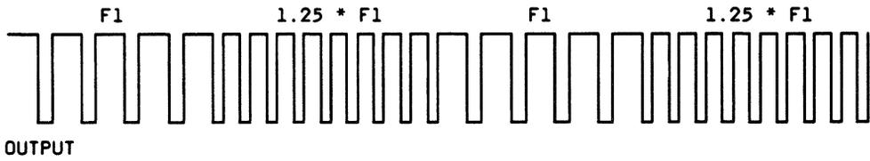
Figure 7. Tone Ringer Output Waveform (Approximately)
