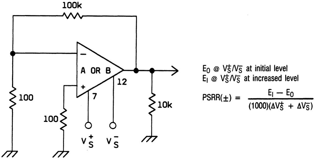
Figure 3. Test Circuit, Power-Supply Rejection Ratio<sup>Ⓢ</sup>
