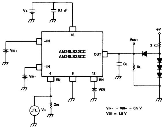
Figure 10. Propagation Delay Times ( $t_{PLZ}$ ,  $t_{PHZ}$ ,  $t_{PZL}$ ,  $t_{PZH}$ )
