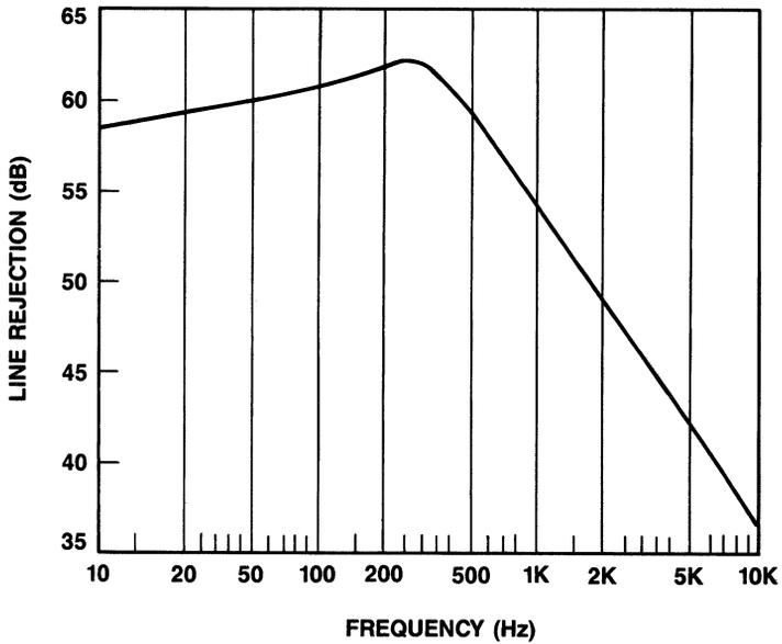
Figure 3. Typical Line Rejection vs. Frequency
