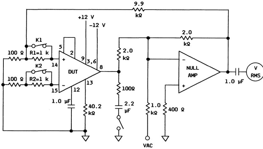
Figure 7. Input Offset Voltage ( $V_{IO}$ ), Input Bias Current ( $I_{IB}$ ), Input Offset Current ( $I_{IO}$ ) and Power-Supply Rejection Ratio (PSRR) Test Circuit
