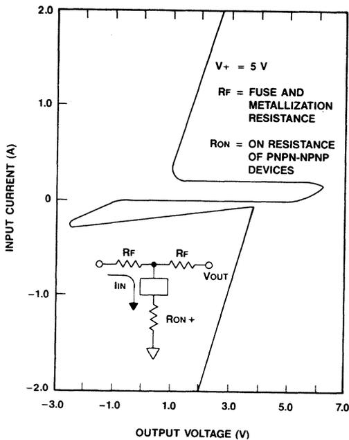
Figure 4. Typical Operating Characteristic
