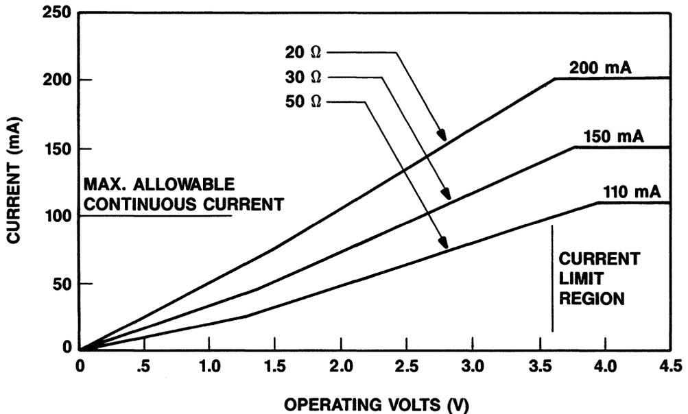
Figure 3. Output I/V Characteristics for Various RON @ 25°C
