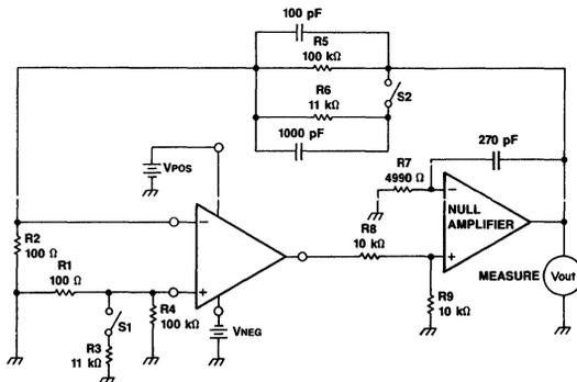
Figure 2. Input Offset Voltage ( $V_{io}$ ), Input Bias Current ( $I_{IB}$ ), and Input Offset Current ( $I_{io}$ ) Test Circuit
