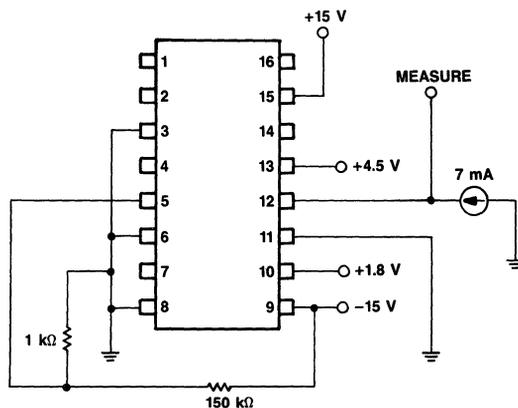
Figure 7. Low-Voltage Output ( $V_{OL}$ ), ( $I_{12} = -7 \text{ mA}$ )
