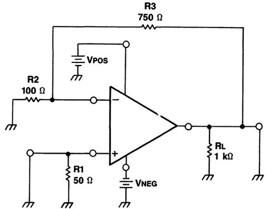
Figure 8. Slew Rate Test Circuit
