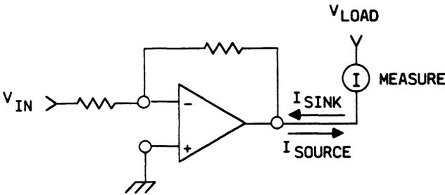
Figure 3. Test Circuit, Output Current
