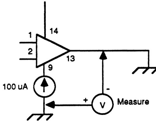
Figure 10. Forward Voltage, Output Diode D2 Test Circuit
