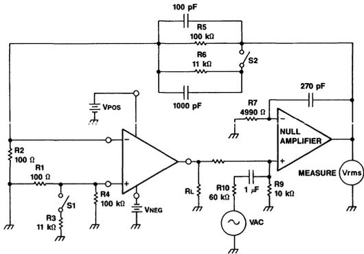
Figure 1. Open Loop Gain Test Circuit
