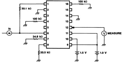
Figure 2. Bandgap Output Voltage Test Circuit
