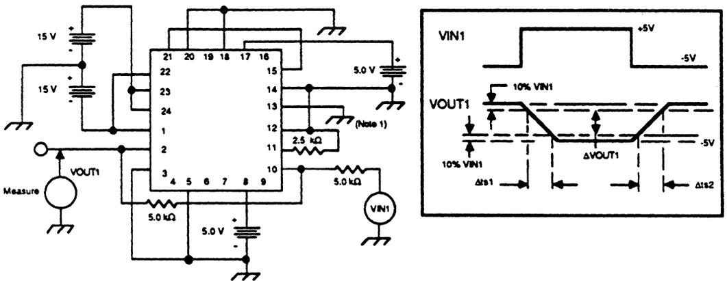
Figure 6. Slew Rate Test Circuit
