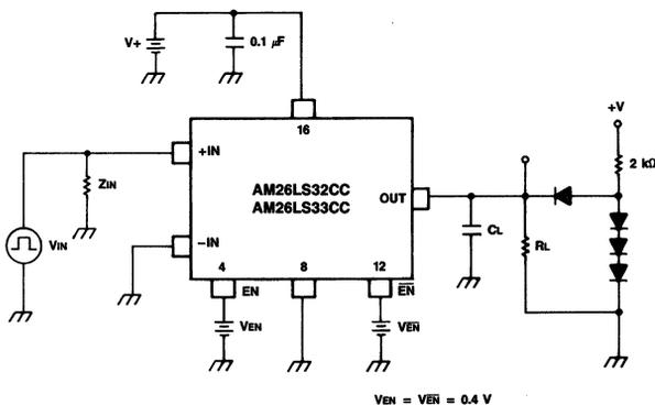
Figure 9. Propagation Delay Times ( $t_{PLH}$ ,  $t_{PHL}$ )
