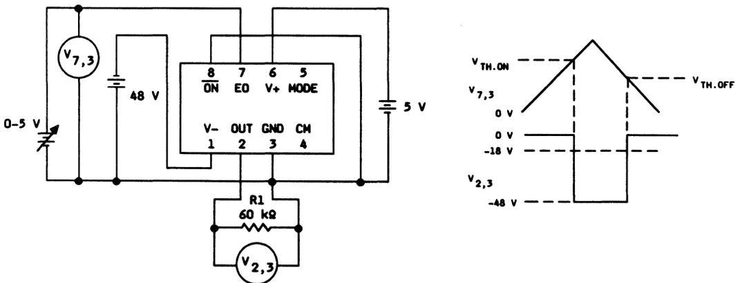
Figure 7. EO Threshold Tests
