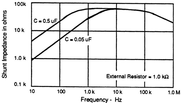
Figure 10. Typical Shunt Impedance vs Frequency
