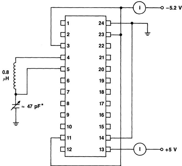
\* Capacitor should be adjusted so the resonant frequency of the tank circuit (including lead length, etc.) is nominally 20 MHz.
