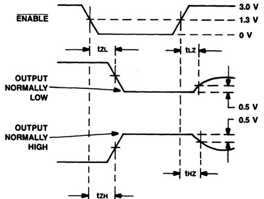
Figure 12.  $\overline{\text{ENABLE}}$  and Output Waveforms
