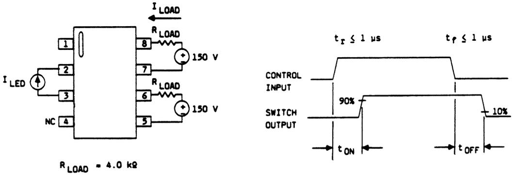
Figure 4.  $t_{ON}/t_{OFF}$  Test Circuit and Waveform
