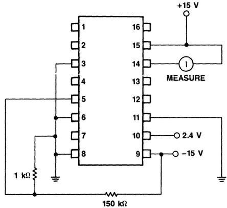
Figure 4. Logic Supply Current ( $I_{14}$ )
