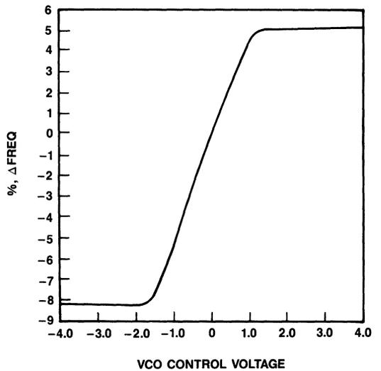
Figure 5. VCO Control Voltage\* vs. Percent Change in Frequency
