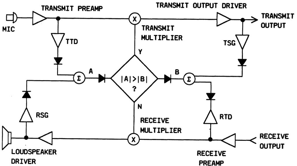
Figure 1. Simplified Speakerphone Circuit
