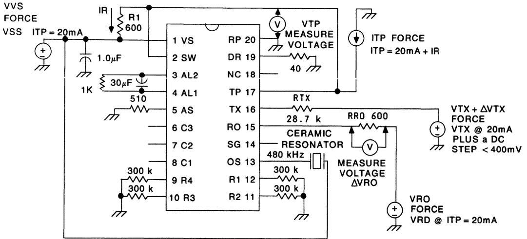
DETERMINE THE VALUE OF IR AND RECORD VRO VOLTAGE: Force 20 mA into RP (Pin 17) with TX (Pin 16) open and R1 disconnected. Measure VVS voltage (Pin 1), VTP voltage (Pin 17) and VRO voltage (Figure 18). Then,  $IR \text{ (mA)} = [(VTP - VSS)/600] \text{ times } 1000$ .
