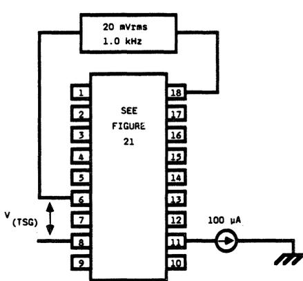
Figure 39. LB1021AD Test Circuit
