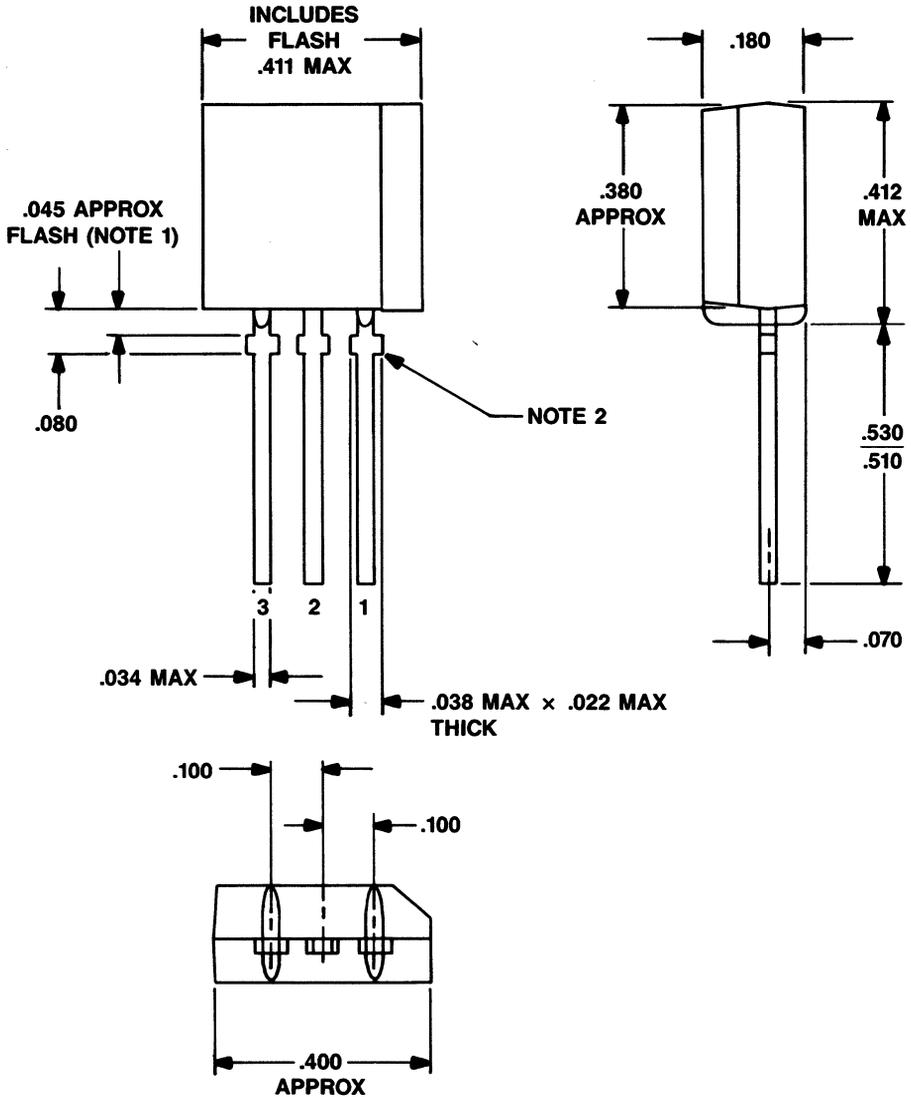
**Note 1.** Flash permissible in this area along with lead length not to exceed the .038" max. wide X .022" max thickness of the leads.
