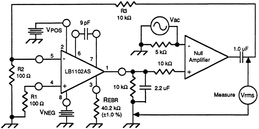
$$\text{GAIN (dB)} = 20 \left[ \text{Lo} \left( K \frac{V_{\text{rms}}}{V_{\text{ac}}} \right) \right]; \text{ where } K = \frac{R_2 + R_3}{R_2}$$
