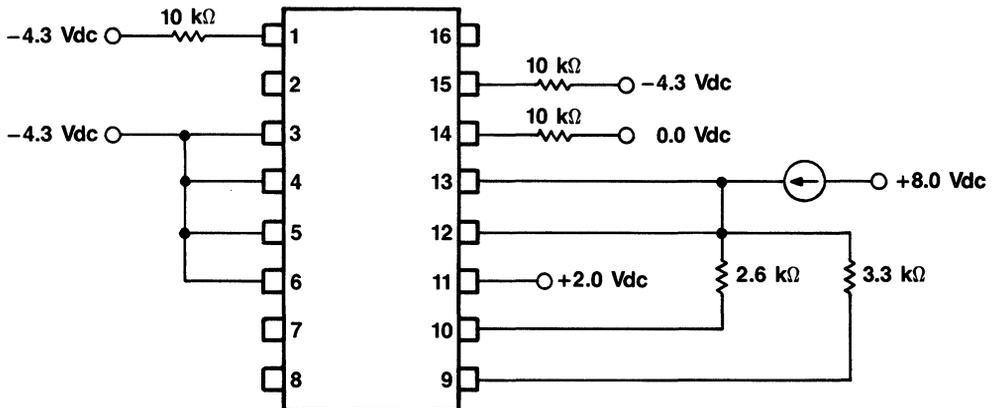
Figure 1. Current Supply (I<sub>S</sub>)
