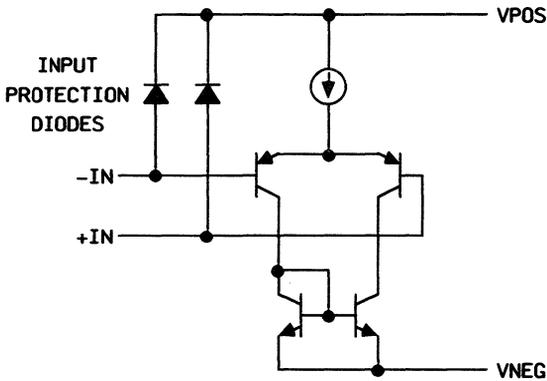
Figure 1. Simplified Input Diagram
