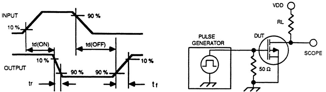
**Figure 1. Switching Waveforms and Simplified Test Circuit**
