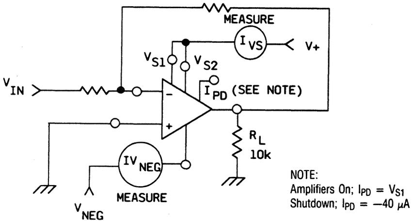
Figure 2. Test Circuit, Power-Supply Current
