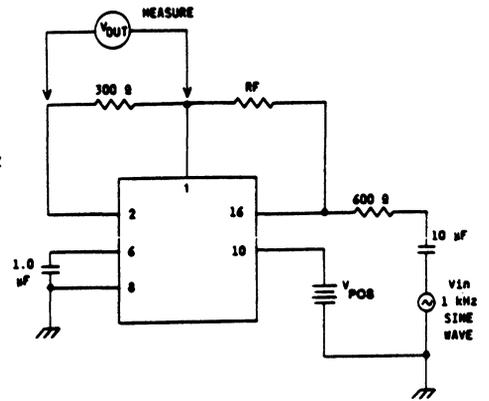
Figure 6. Receive Amplifier, Output and Gain
