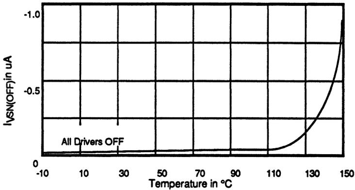
Figure 14. Typical Supply Current (I<sub>VSN(OFF)</sub>) vs Temperature
