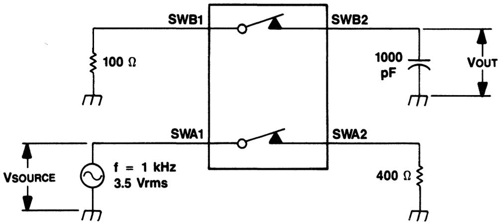
$$\text{CROSSTALK} = 20 \text{ LOG } \frac{V_{\text{OUT}}}{V_{\text{SOURCE}}}$$
