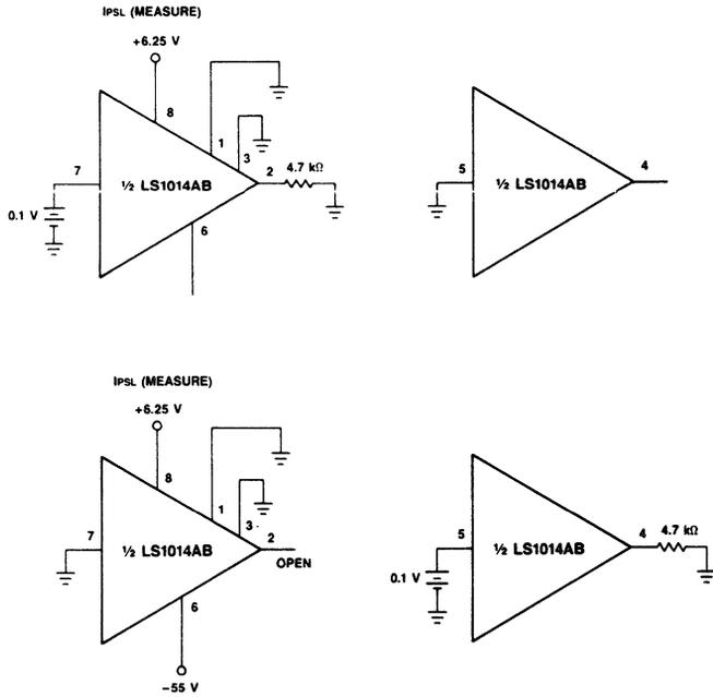
Figure 5. Logic Supply, Current Off
