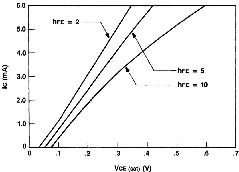
Current vs. Voltage Characteristics (NPN 1X)
