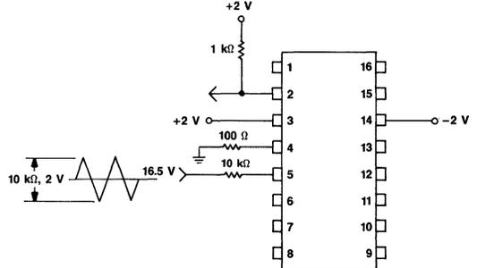
Figure 2. Input Offset Voltage; Input Bias Current; Input Offset Current (+Vs = 2 V and -Vs = -2 V)
