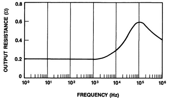
Figure 7. Typical Output Resistance vs. Frequency
