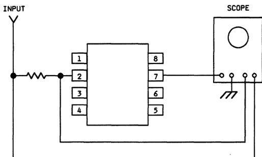
**Figure 2. Hold Current and Breakover Voltage Tests**
