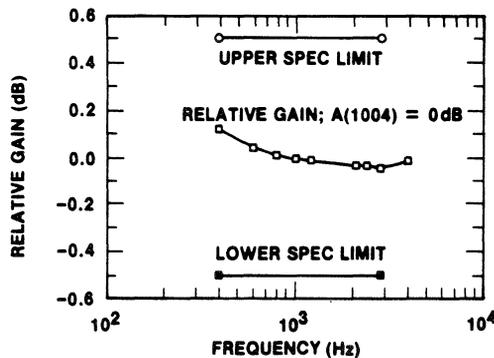
Figure 18(a). LB1012AA/AD Typical Gain vs Frequency Response
