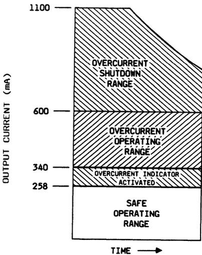
Figure 1 is an output diagram of a typical LB1019AB at room temperature as a function of load current.
