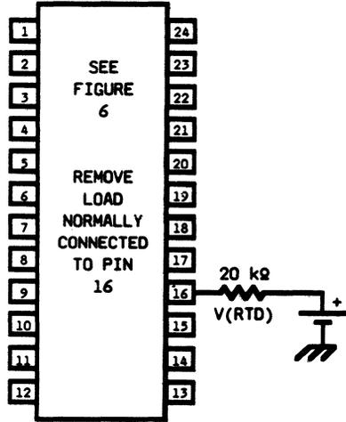
Figure 8. LB1020AF Test Circuit
