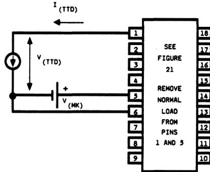
Figure 35. LB1021AD Test Circuit
