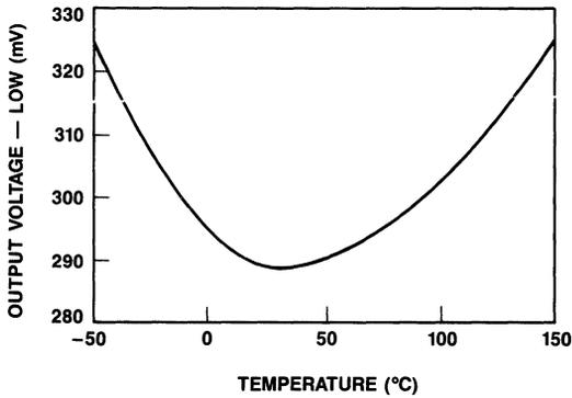
Figure 11. Typical Low-Level Output Voltage vs. Temperature
