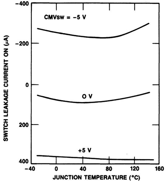
Figure 16. Typical ON Leakage Current vs. Temperature
