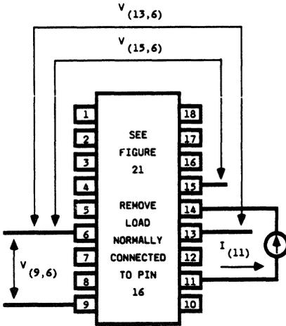
Figure 22. LB1021AD Test Circuit
