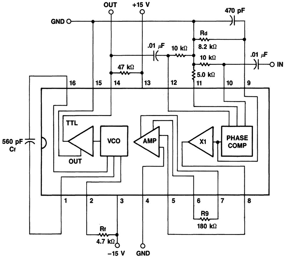
Figure 5. 200 kHz Synchronizer Application
