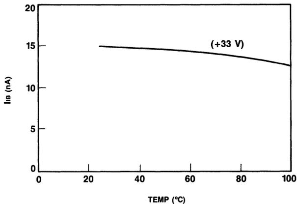
Figure 15. Temperature vs. Input Bias Current at Various Supply Voltages
