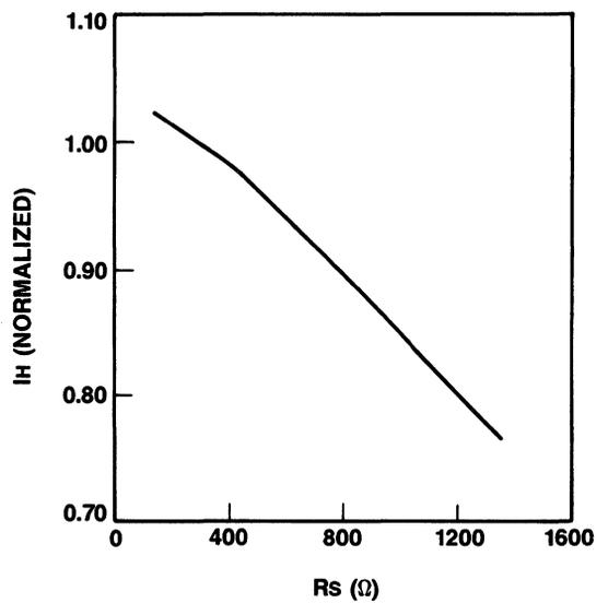
Figure 4. Holding Current vs Series Resistance
