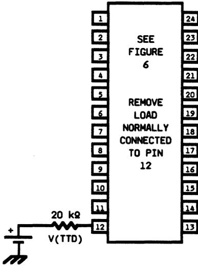
Figure 7. LB1020AF Test Circuit
