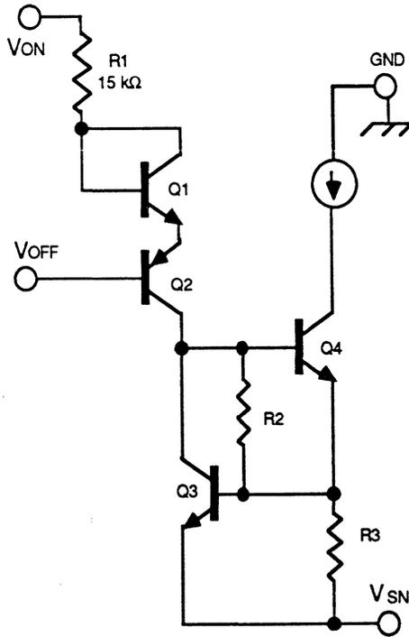
Figure 1. LS1098AAF Simplified Input Diagram
