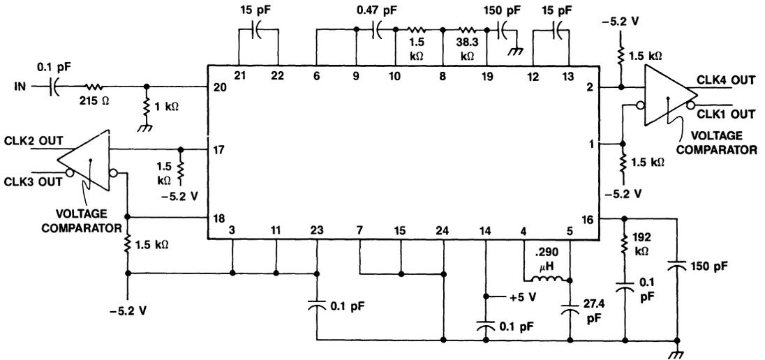
Figure 6. Sample Application Timing Recovery\* in a Synchronous Digital Communication System Operating at 50 MHz
