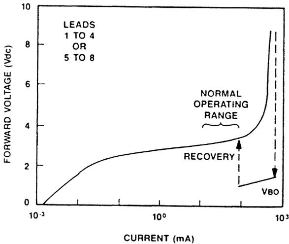
Figure 12. Typical Voltage vs Current (PNPN Composite Device)
