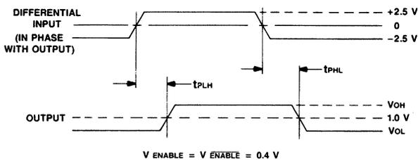
Figure 11. Signal Propagation Delay Time
