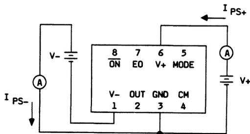
**Figure 3. Power-Supply Current**
