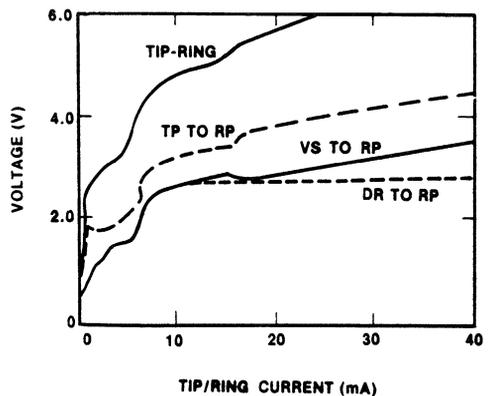
Figure 2. Typical V-1 Characteristics (Speech Mode)
