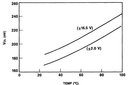
Figure 12. Temperature vs. Output Voltage (Low) at Various Supply Voltages
