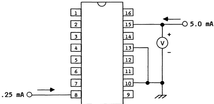
Figure 3. Saturation Voltage ( $V_{CE}$ ) Test Circuit
