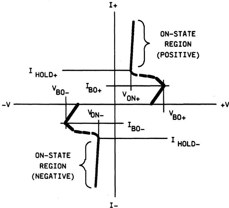
Figure 1. Symbology for Test Characteristics (Not to Scale)
