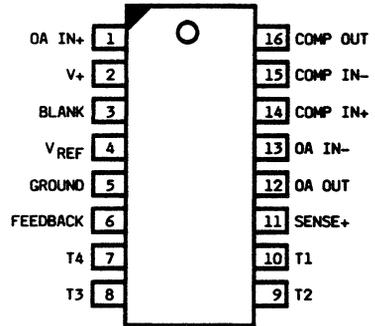
Figure 2. 16-Pin Plastic DIP
