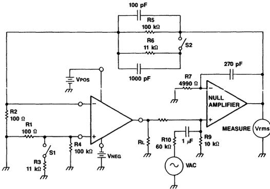
Figure 1. Open Loop Gain Test Circuit
