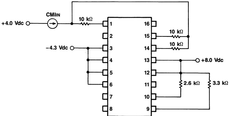
Figure 3. Common Mode Input Current ( $CMI_{IN}$ )
