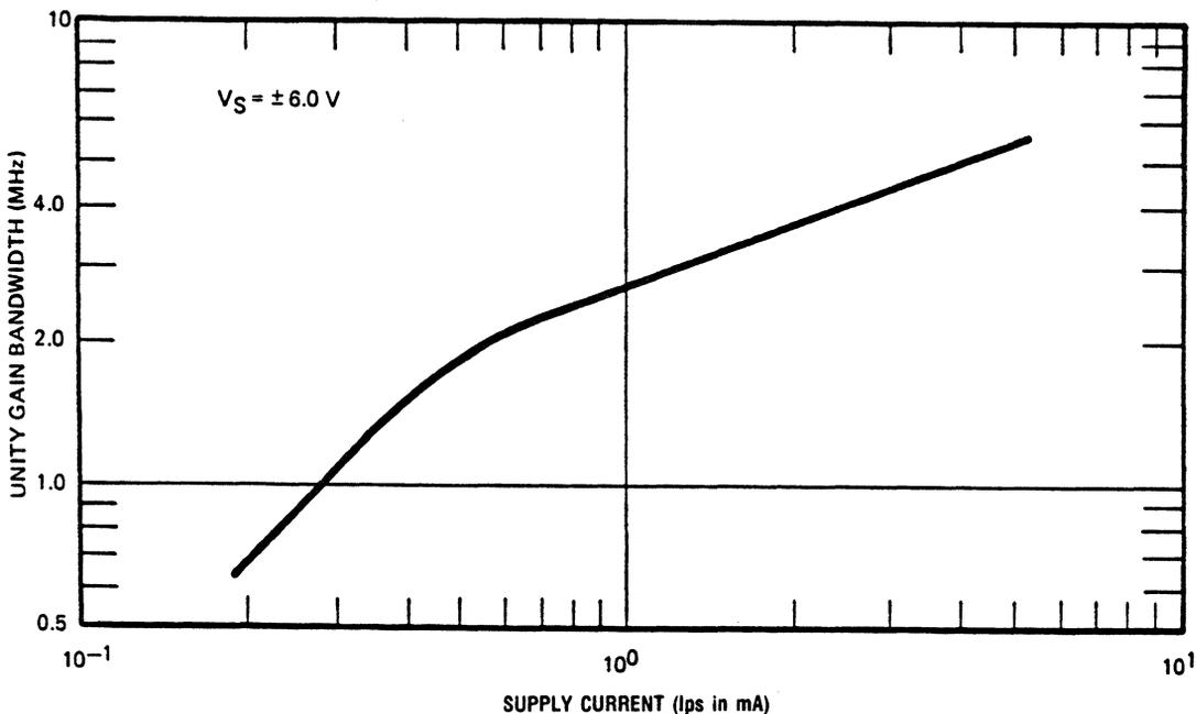
Figure 15. Supply Current/Unity Bandwidth Characteristic
