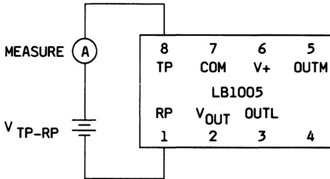
Figure 4. Test Circuit (TP and RP Current, Low Voltage)
