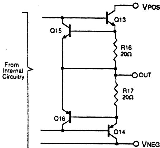
Figure 1. Sample-And-Hold Op-Amp Outputs (Simplified)
