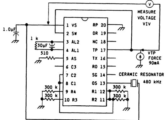
Figure 9. Voltage (TP-to-VS), Dial
