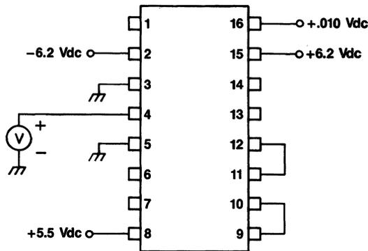
Figure 5. Input Forward Current,  $V(s) = 0$
