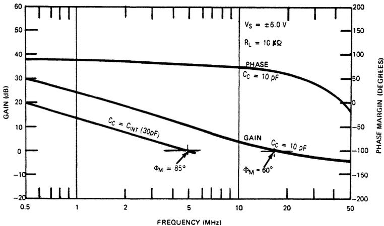
Figure 17. Open-Loop Gain and Phase vs. Frequency
