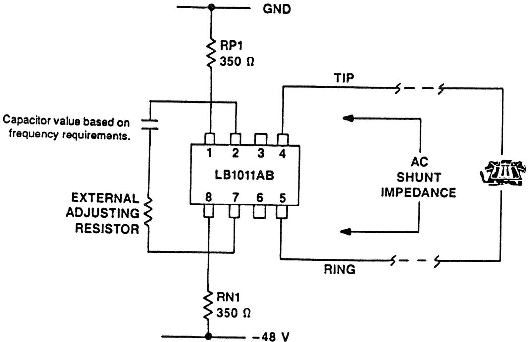
Figure 13. Battery Feed Application (Balanced Configuration)
