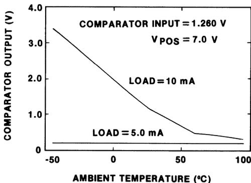
Figure 7. Typical Temperature Characteristics Comparator Output Voltage vs. Comparator Input Overdrive of 10 mV
