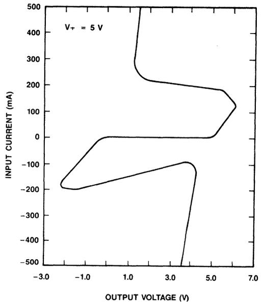
Figure 5. Typical Operating Characteristic
