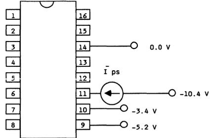
Figure 3. Power-Supply Current (- Ips) Test Circuit
