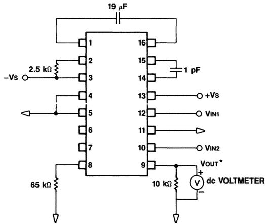
Measure  $V_{OUT}$  under the following conditions
