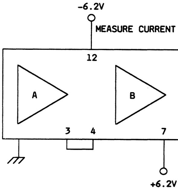
Figure 4. Test Circuit, Power-Supply Current<sup>Ⓢ</sup>
