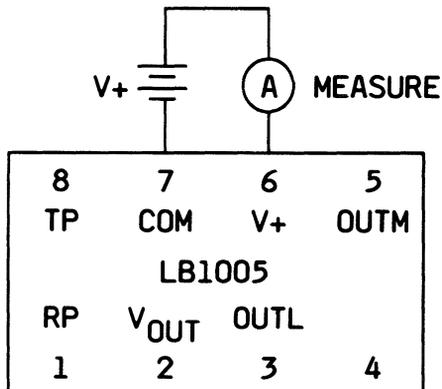
Figure 1. Test Circuit (Power Supply Current)
