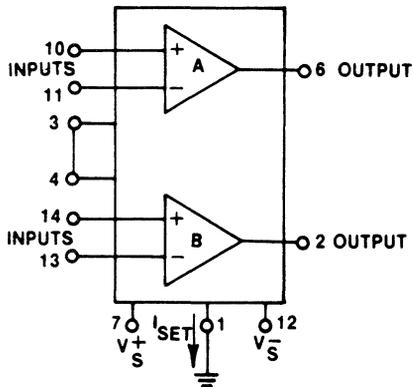
Figure 7. Both Amplifiers Operating, Internal Bias Resistor, Internal Frequency Compensation
