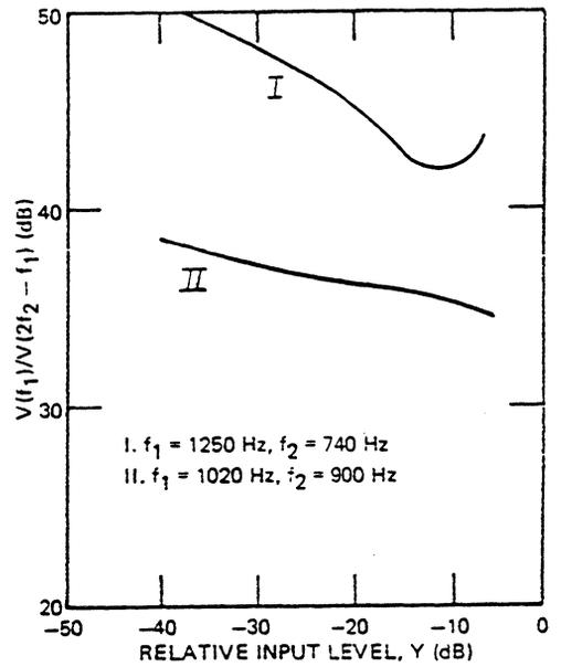
Figure 17. Intermodulation Product ( $2f_2 - f_1$ ) of the Compressor
