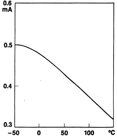
Figure 13. Logic Supply Current vs. Temperature
