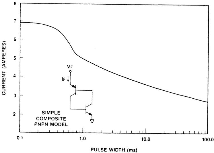
Figure 11. Maximum Applied Forward Surge Limits (PNPN Composite Device)
