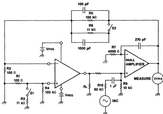
Figure 1. Open Loop Gain Test Circuit
