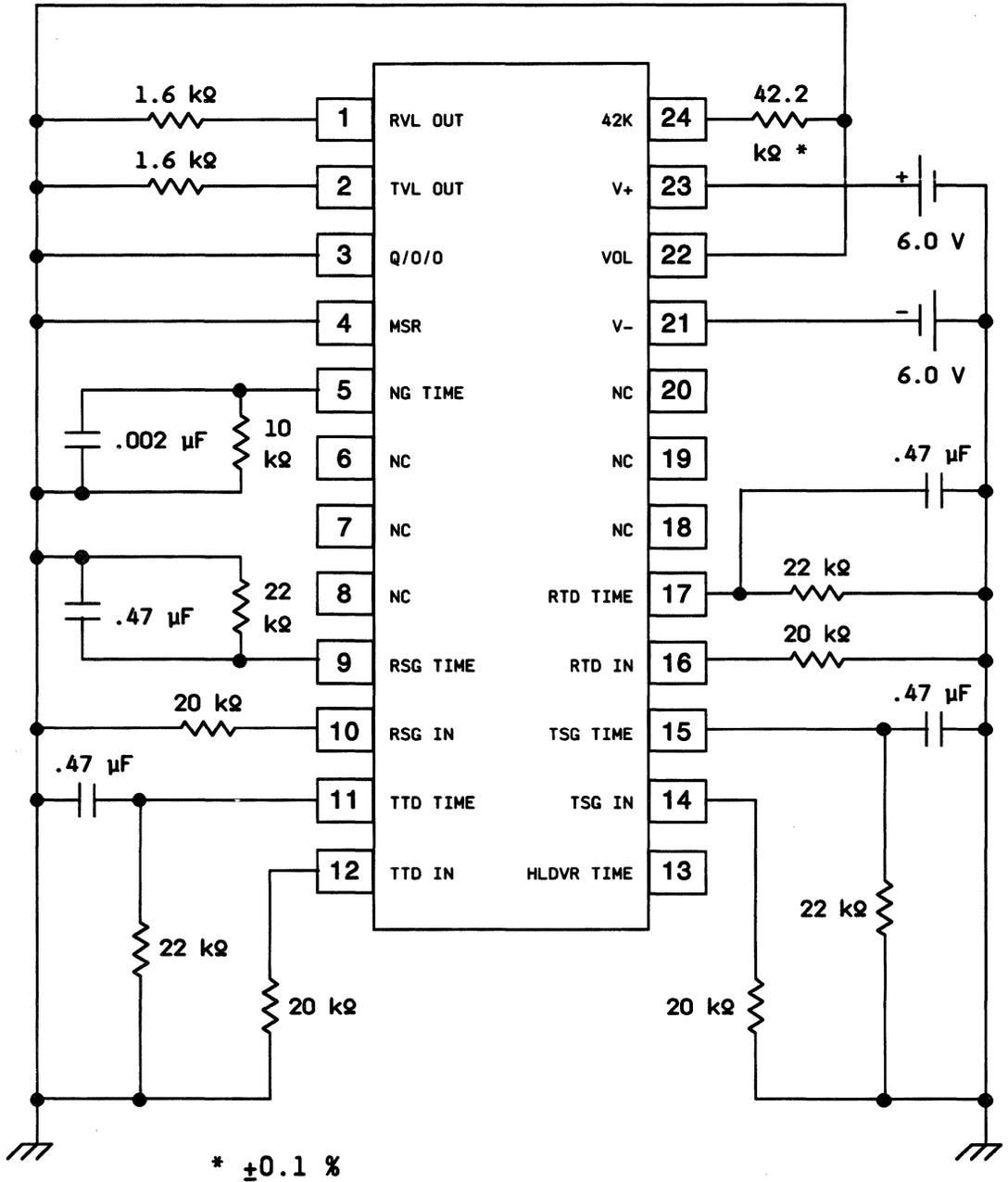
Figure 6. LB1020AF Default Test Circuit
