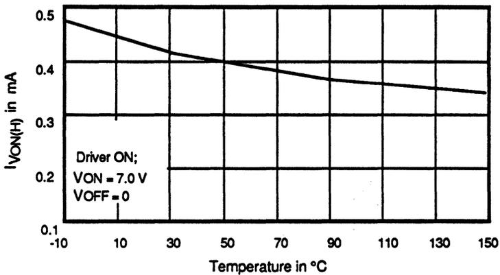
Figure 15. Typical Driver Von Input Current (I<sub>VON(H)</sub>) vs Temperature
