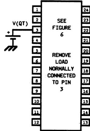
Figure 12. LB1020AF Test Circuit
