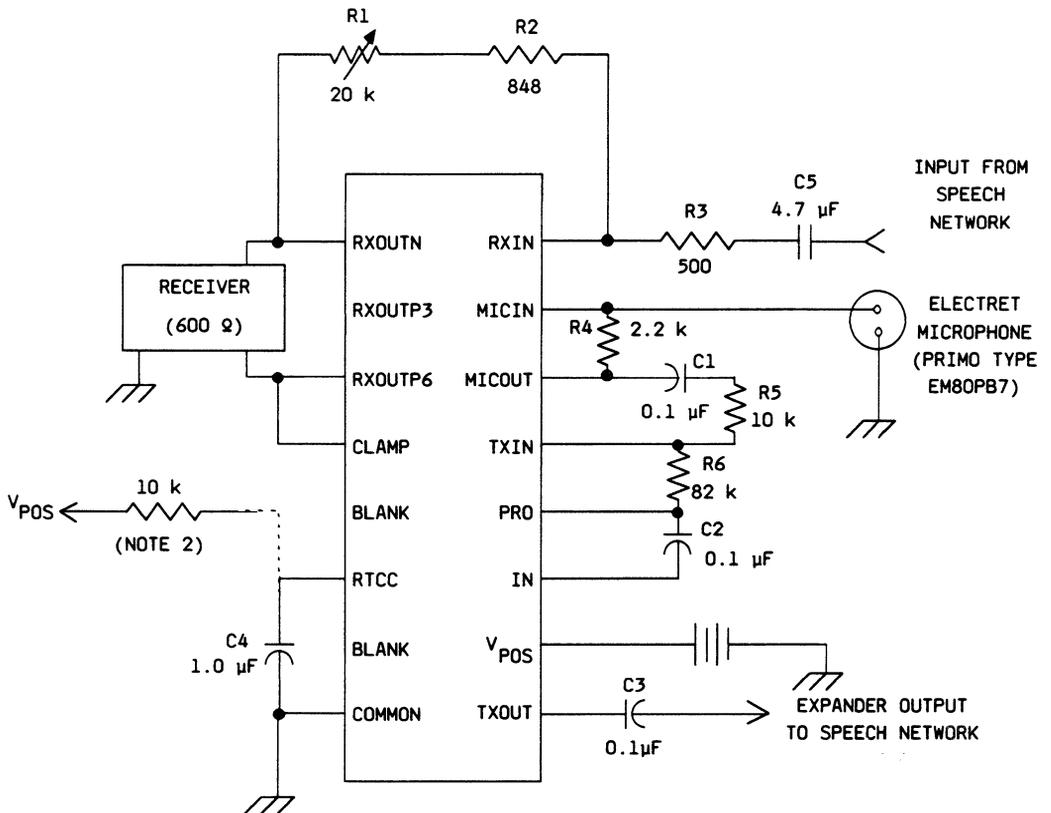
**Note 2:** The RTCC pin may be connected to V<sub>POS</sub> through a 10 kΩ resistor to eliminate the expander function.
