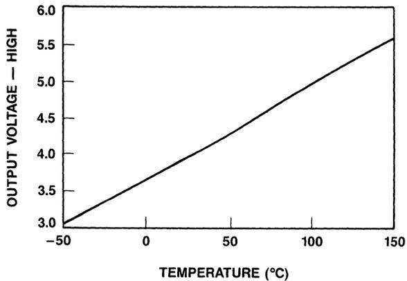
Figure 10. Typical High-Level Output Voltage vs. Temperature
