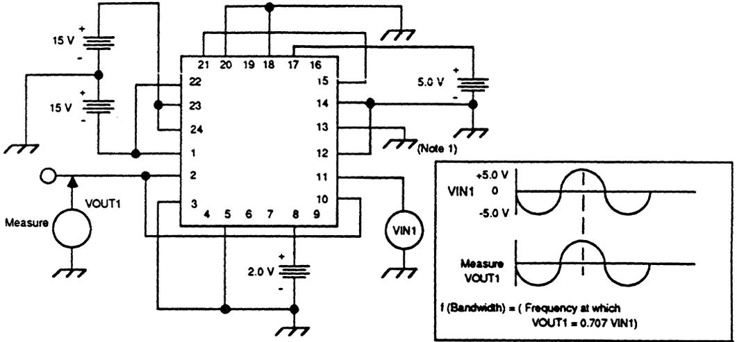
Figure 5. Full-Power Bandwidth Test Circuit
