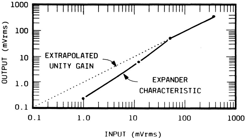
Figure 10. Typical Expander Characteristics
