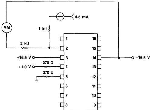
Figure 3. Low-Level Output Voltage (+Vs = +16.5 V and -Vs = -16.5 V)
