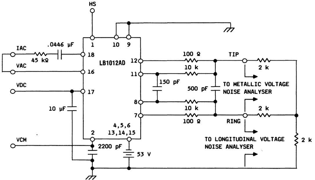
Figure 20(c). LB1012AD Noise Test Circuit
