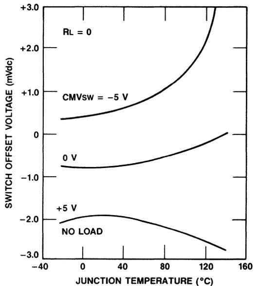
Figure 14. Typical Switch Offset Voltage vs. Temperature
