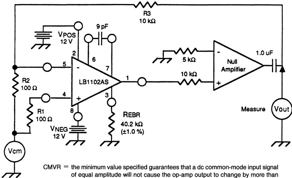
CMVR = the minimum value specified guarantees that a dc common-mode input signal of equal amplitude will not cause the op-amp output to change by more than  $\pm 2$  mV.
