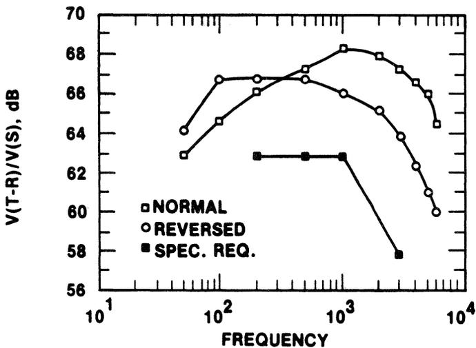
Figure 19(a). LB1012AA/AD Typical Longitudinal Balance vs Frequency
