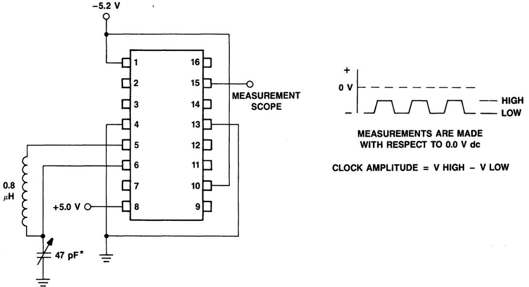
\* Capacitor should be adjusted so the resonant frequency of the tank circuit (including lead length, etc.) is nominally 20 MHz.
