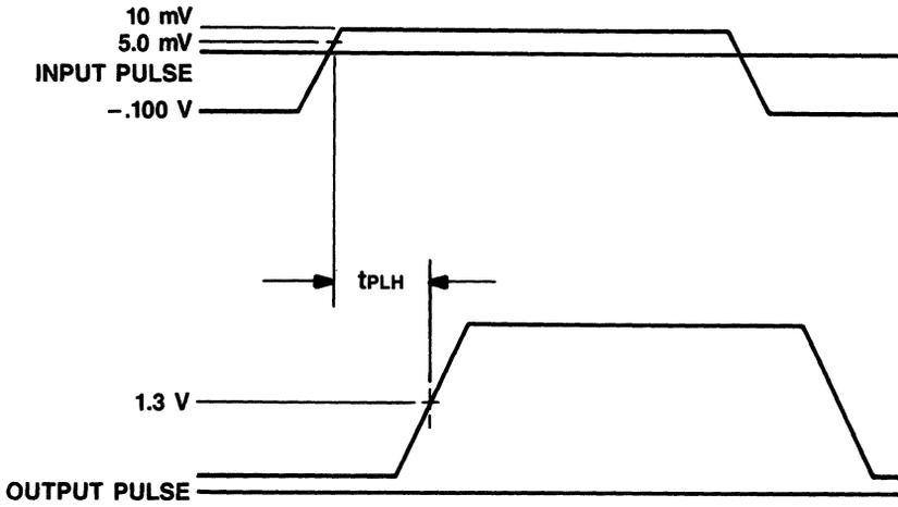
Figure 1. Positive Input and Output Waveforms
