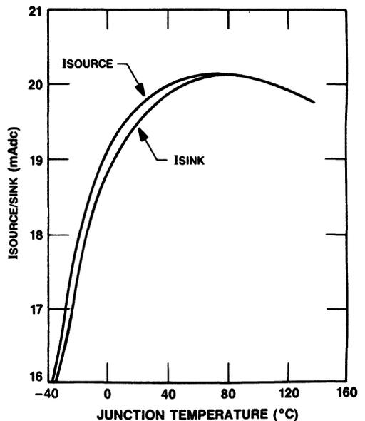
Figure 18. Typical Source and Sink Current vs. Temperature
