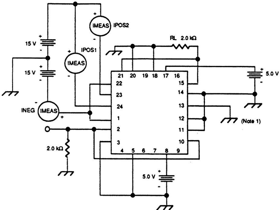
Figure 11. Power Supply Current Test Circuit
