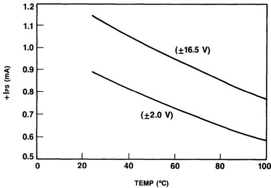
Figure 9. Temperature vs. Power Supply Current at Various Supply Voltages
