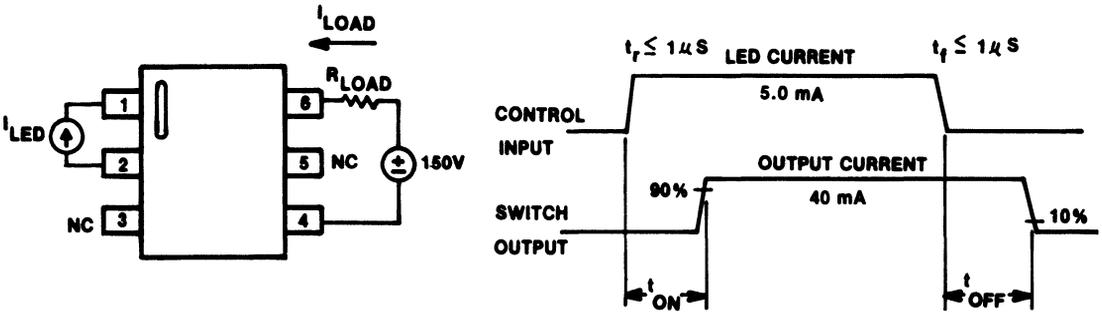
Figure 2. ton/toff Test Circuit and Waveform
