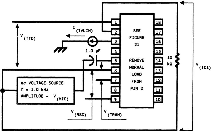
Figure 38. LB1021AD Test Circuit
