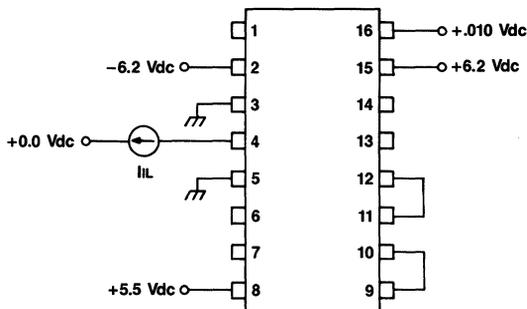
Figure 4. Logic Supply Current ( $I_{psL}$ )
