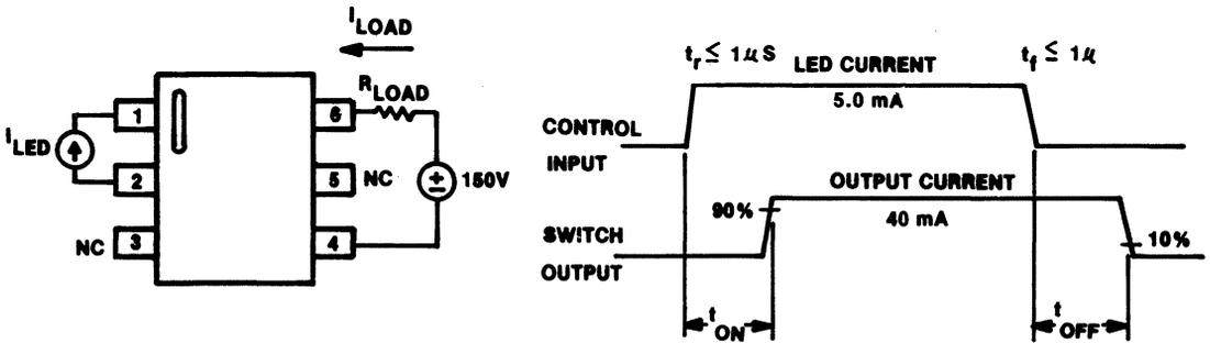
Figure 6.  $t_{ON}/t_{OFF}$  Test Circuit and Waveform
