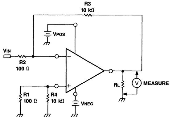
Figure 4. Output Voltage Swing Test Circuit
