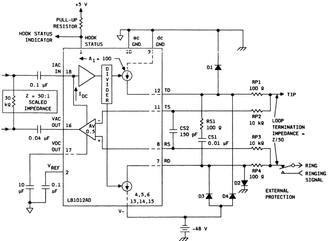
Figure 22. LB1012AD Battery Feed Application Diagram
