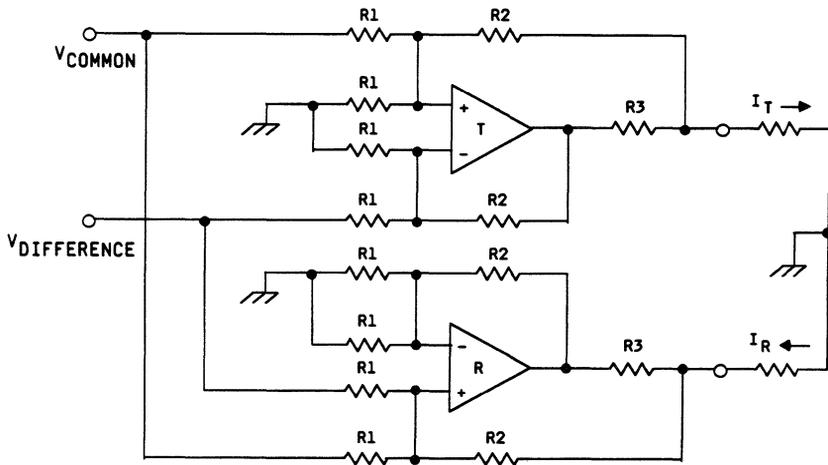
**Figure 6. Simplified Line Feed Operation (Power-Supply Connections Not Shown)**
