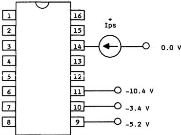
Figure 2. Power-Supply Current (+ Ips) Test Circuit
