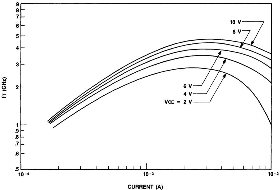
Current vs. Breakdown Voltage (NPN 1X)
