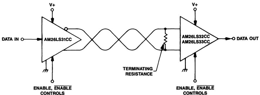
Figure 13. AM26LS32CC, AM26LS33CC Quad Line Receiver Application Diagram
