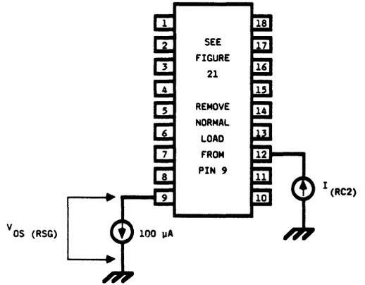
Figure 27. LB1021AD Test Circuit
