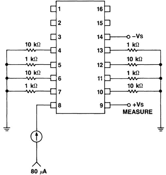
Figure 8. Power Supply Current (Disabled)
