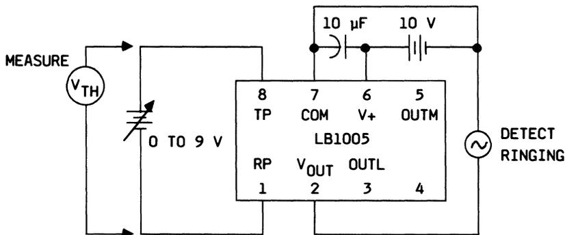
Figure 3. Test Circuit (Input Threshold Voltage)
