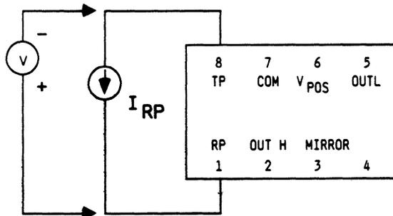
Figure 11. Clamp Voltage ( $I_{RP}$ )
