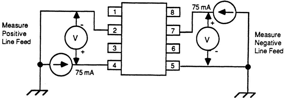
Figure 8. Line/Cross Coupling Voltage, Test Circuit
