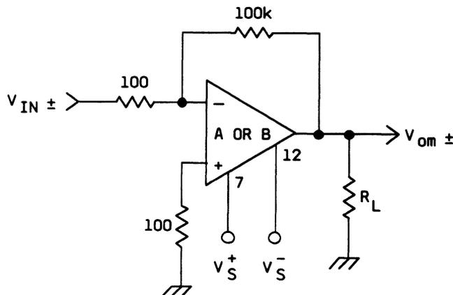
Figure 2. Test Circuit, Output Voltage Swing<sup>Ⓢ</sup>
