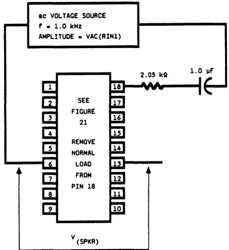
Figure 33. LB1021AD Test Circuit
