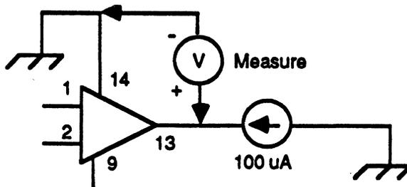
Figure 9. Forward Voltage, Output Diode D1 Test Circuit
