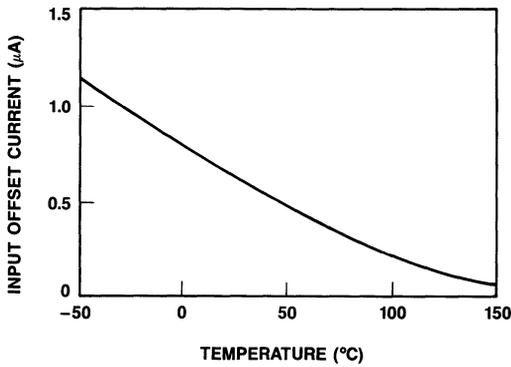
Figure 13. Typical Input Offset Current vs. Temperature
