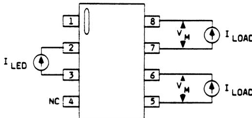
Figure 2. Test Circuit for  $R_{ON}$ , ON Voltage and Breakdown Voltage
