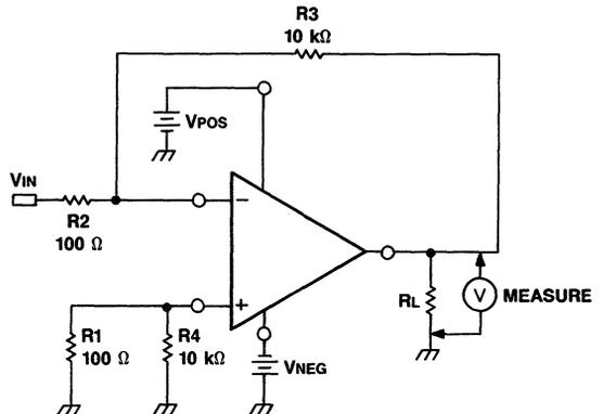
Figure 4. Output Voltage Swing Test Circuit
