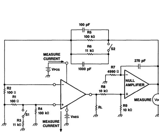
Figure 7. Power Supply Quiescent Current Test Circuit
