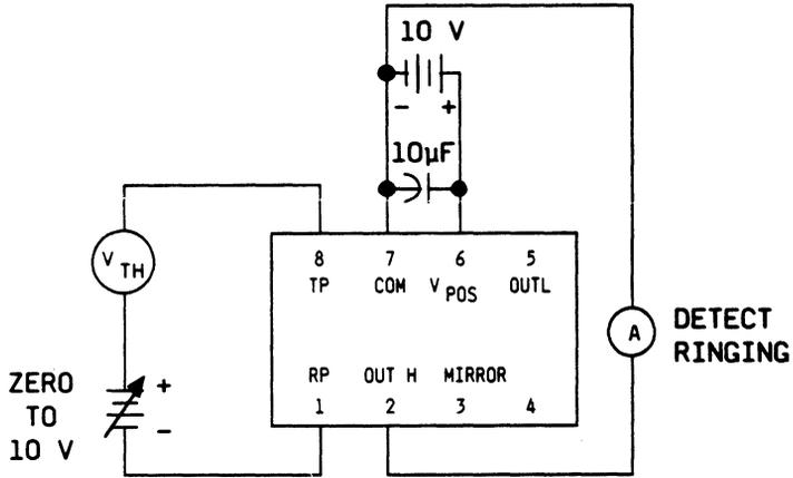
Threshold voltage is the voltage between TP and RP when ringing has been detected ("OUT H" sources current when ringing has been detected). This voltage is increased in the positive direction until the ringing condition occurs.
