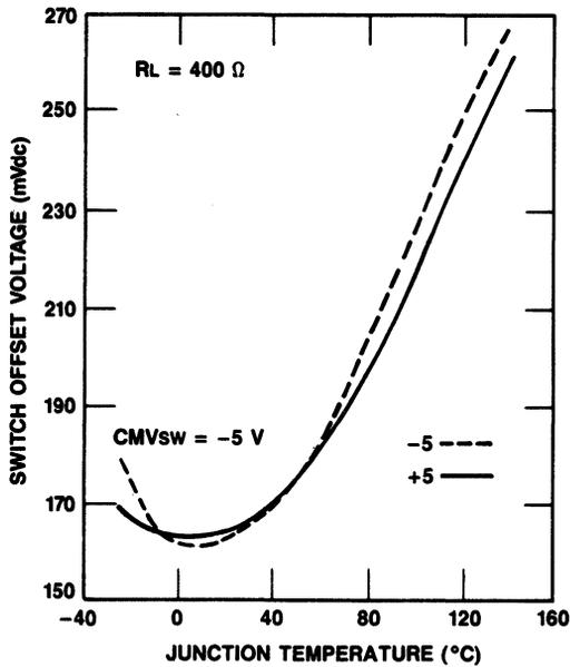
Figure 15. Typical Switch Offset Voltage vs. Temperature
