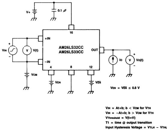
Figure 2. Differential Input Threshold Voltage
