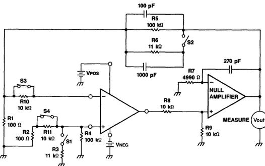
Figure 3. Input Bias and Input Offset Current Test Circuit
