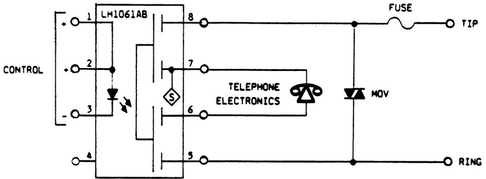
Figure 5. Balanced Switchhook Application
