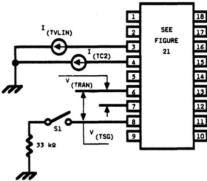
Figure 36. LB1021AD Test Circuit
