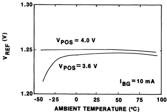
Figure 1. Precision Low-Voltage Reference Start-Up Characteristics
