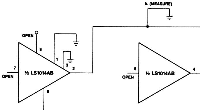
Figure 3. Output Leakage Current
