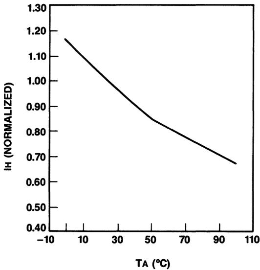
Figure 3. Holding Current vs Temperature
