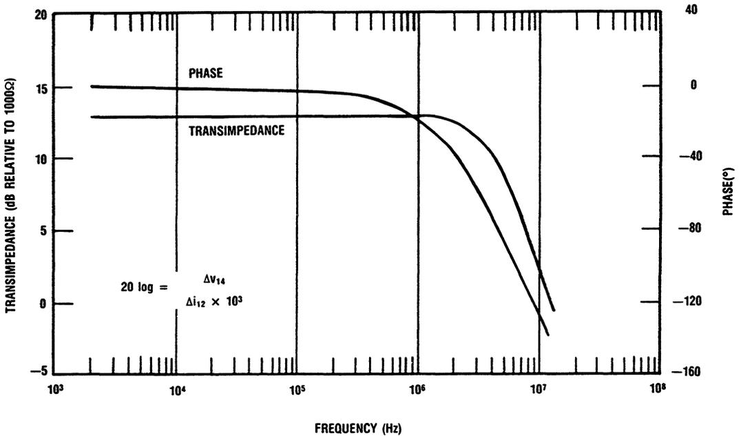
Figure 8. Typical Transimpedance and Phase vs Frequency
