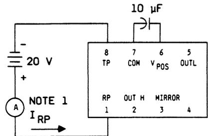
Figure 8. RP Current, No Load
