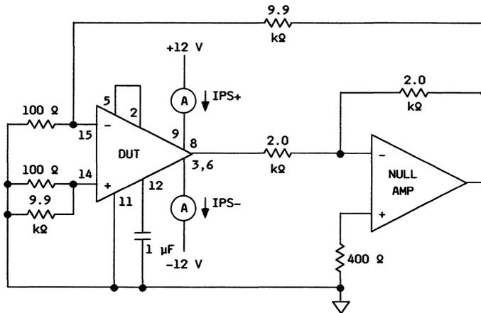
Figure 8. Power-Supply Current Test Circuit
