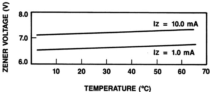
Figure 9. Zener Voltage vs. Temperature at 1 mA and 10 mA
