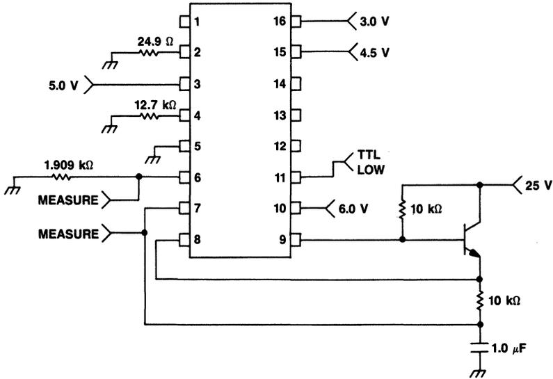
Figure 4A. Driver Output Test
