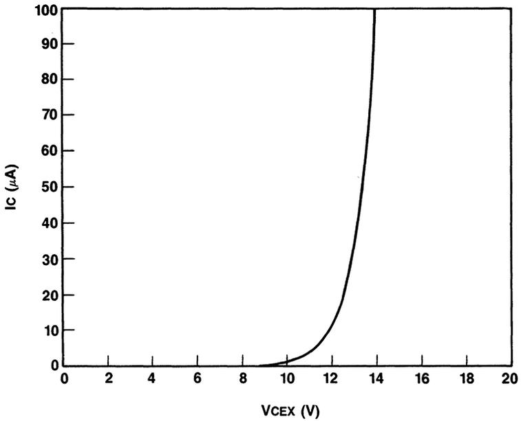
Current vs. Saturation Voltage (NPN)
