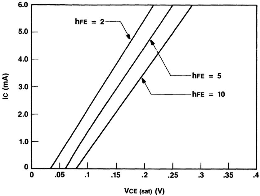
Current vs. Saturation Voltage (PNP)
