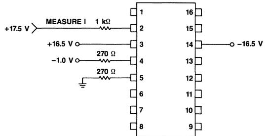
Figure 4. Output Leakage Current (+Vs = +16.5 V and -Vs = -16.5 V)
