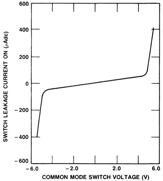
Figure 8. Typical Leakage Current vs. Common-mode Voltage
