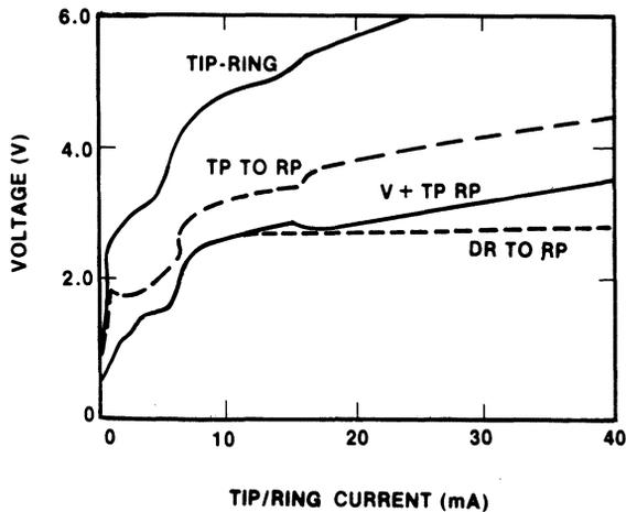
Figure 2. Typical V-I Characteristics (Speech Mode)
