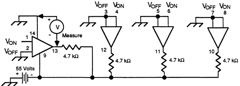
Figure 6. Output-On Voltage Test Circuit
