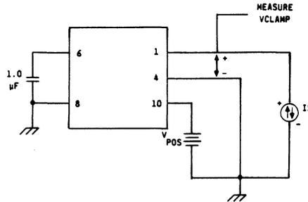
Figure 7. Clamp Voltage
