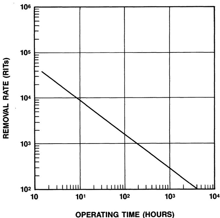
Figure 2. Analog Integrated Circuit Removal Rate (based on experimental data); ( $T_j = 50^\circ\text{C}$ )
