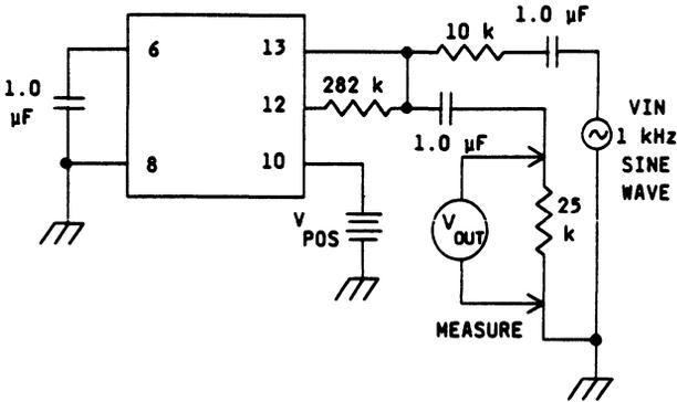
Figure 5. Pre-Amp Output and Gain
