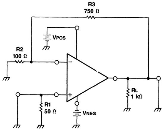
Figure 8. Slew Rate Test Circuit
