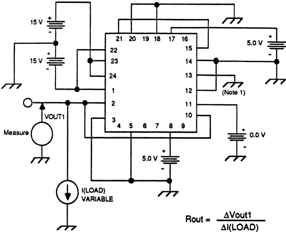
Figure 7. Output Resistance Test Circuit
