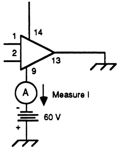
Figure 12. Reverse Leakage Current, Output Diode D2 Test Circuit
