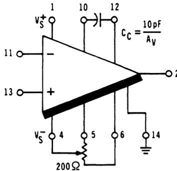
**Figure 14. High Current Output
