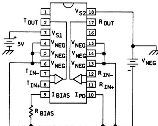
Figure 6. LB1108AD Op-Amp (Ground Return Connections)
