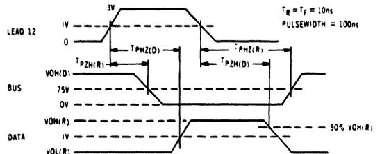
Figure 6.  $\overline{TE}$  to Driver and Receiver Timing Waveform
