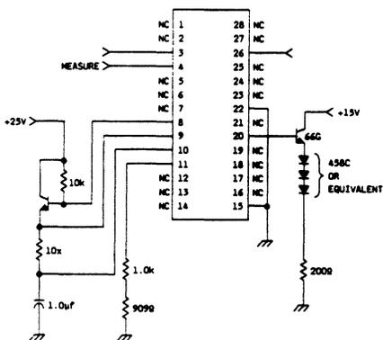
Figure 5. Test Circuit
