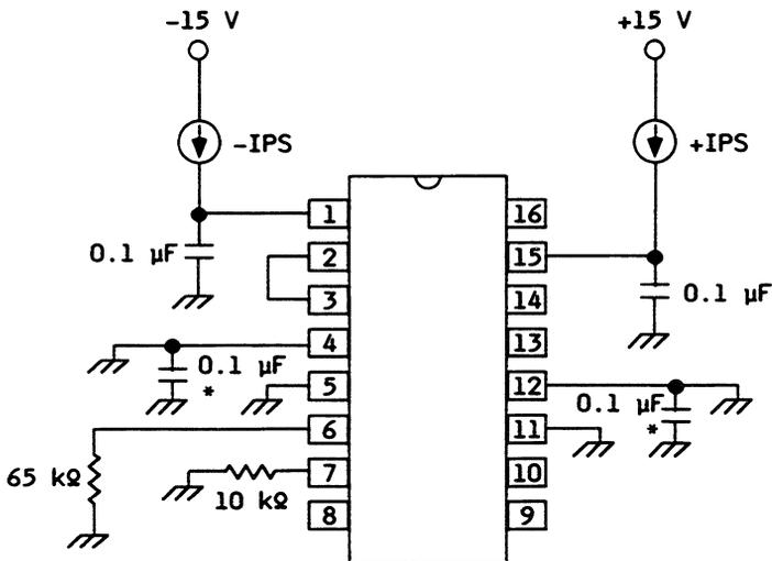
Figure 3. Power-Supply Currents (+ Ips, - Ips) Test Circuit
