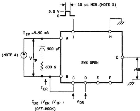
Figure 7. ON Hook dc Test Circuit
