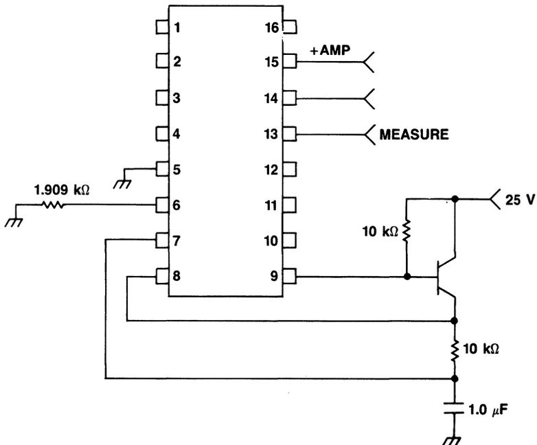
Figure 3. Op Amp Output Voltage Swing
