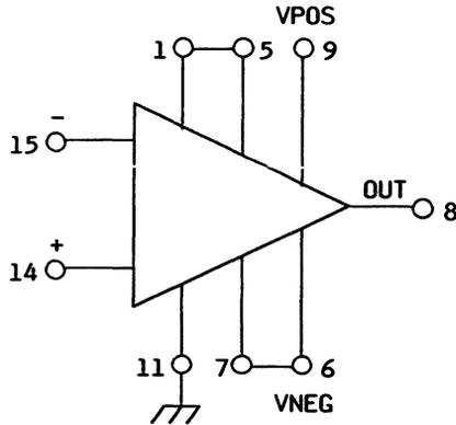
**Figure 3. Internal Bias Setting Internal "T" Compensation**
