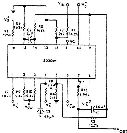
Figure 8. Typical Compressor Connections
