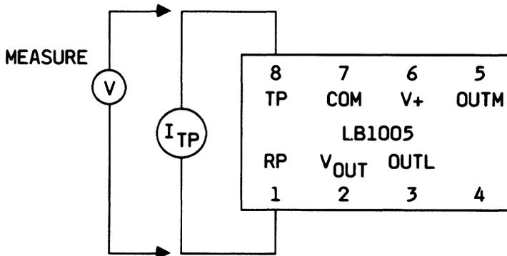
Figure 5. Test Circuit (Clamp Voltage)
