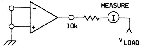
Figure 4. Test Circuit, Output Leakage Current
