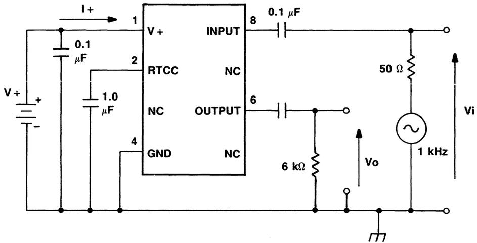
Figure 1. LB1026AB Test Circuit
