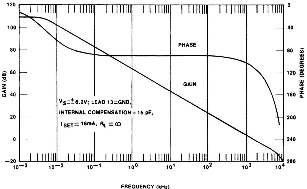
Figure 9. Typical Open-Loop Gain and Phase vs Frequency
