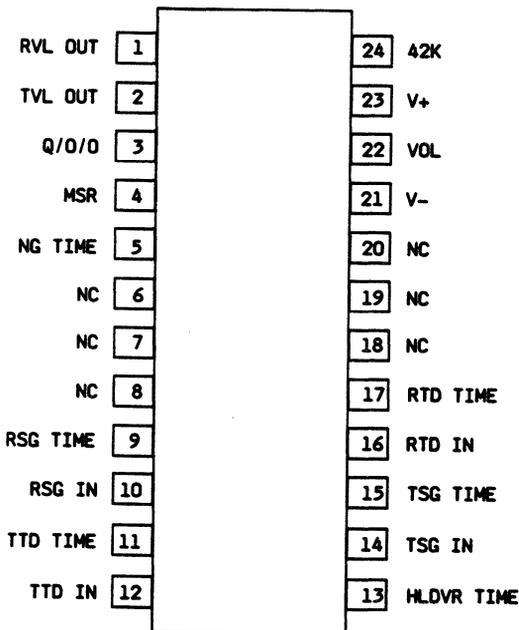
Figure 2. LB1020AF 24-Pin Plastic DIP
