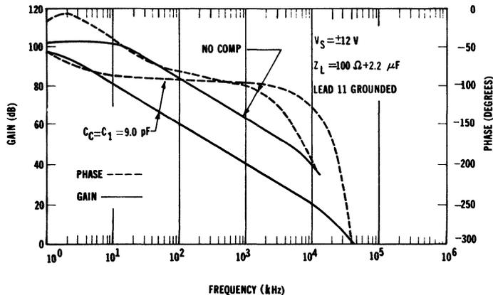
**Figure 10. Open-Loop Gain and Phase vs. Frequency**
