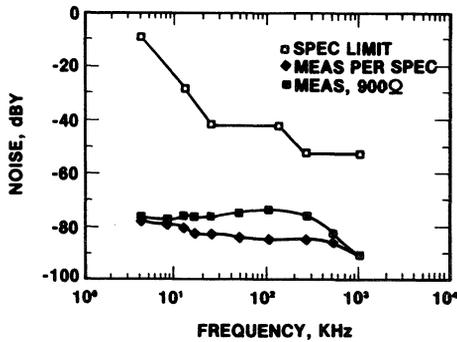
Figure 20(a). Typical. Metallic Out-of-Band Noise
