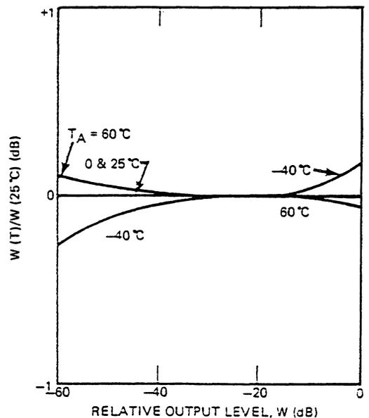
Figure 11. Temperature Stability of the Expander
