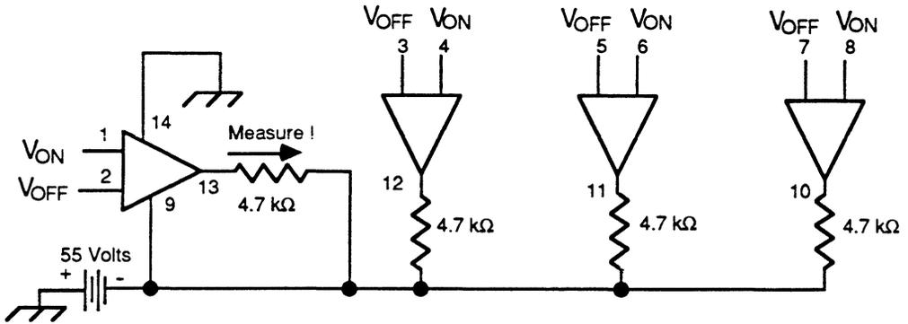
Figure 4. Fail-Safe Output Leakage Current Test Circuit
