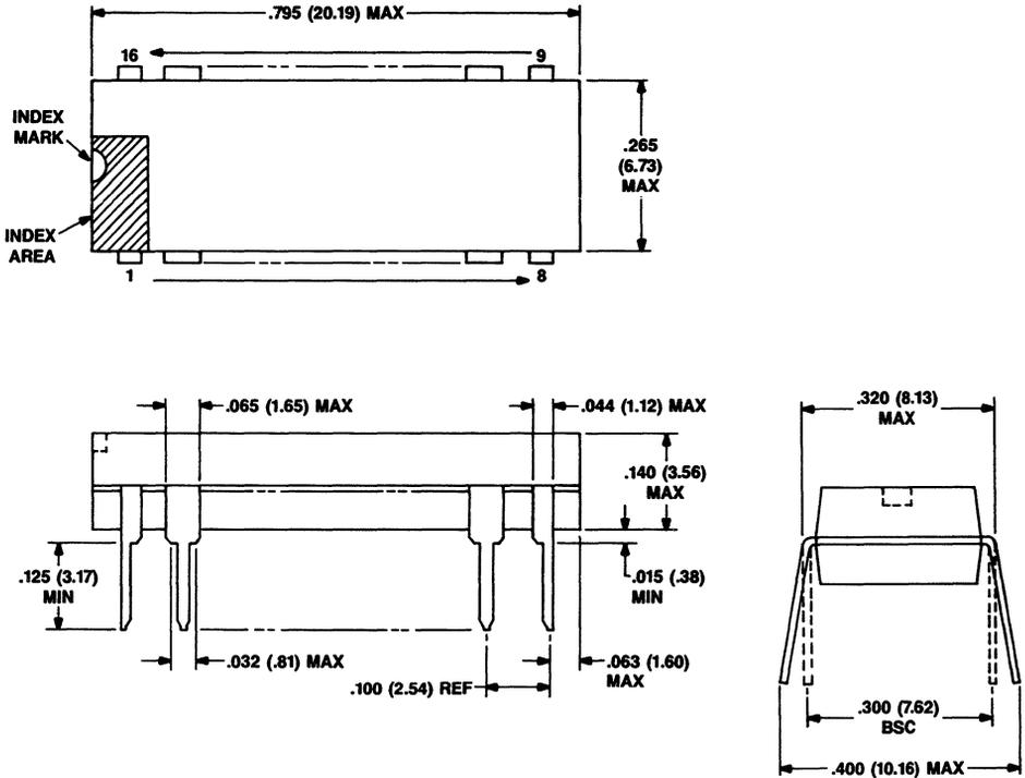
Package D—Standard 18-pin DIP (Dimensions in Inches)
