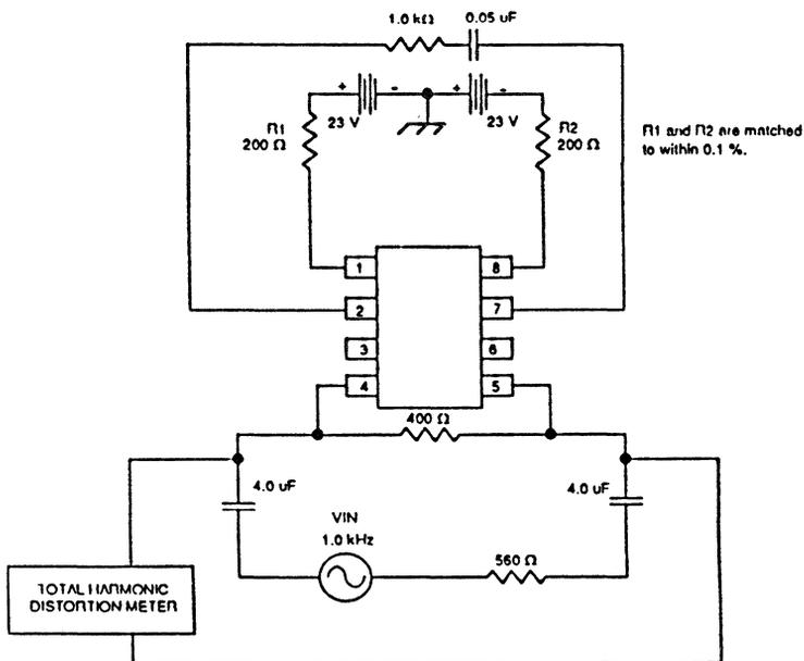
Figure 4. Distortion, Test Circuit
