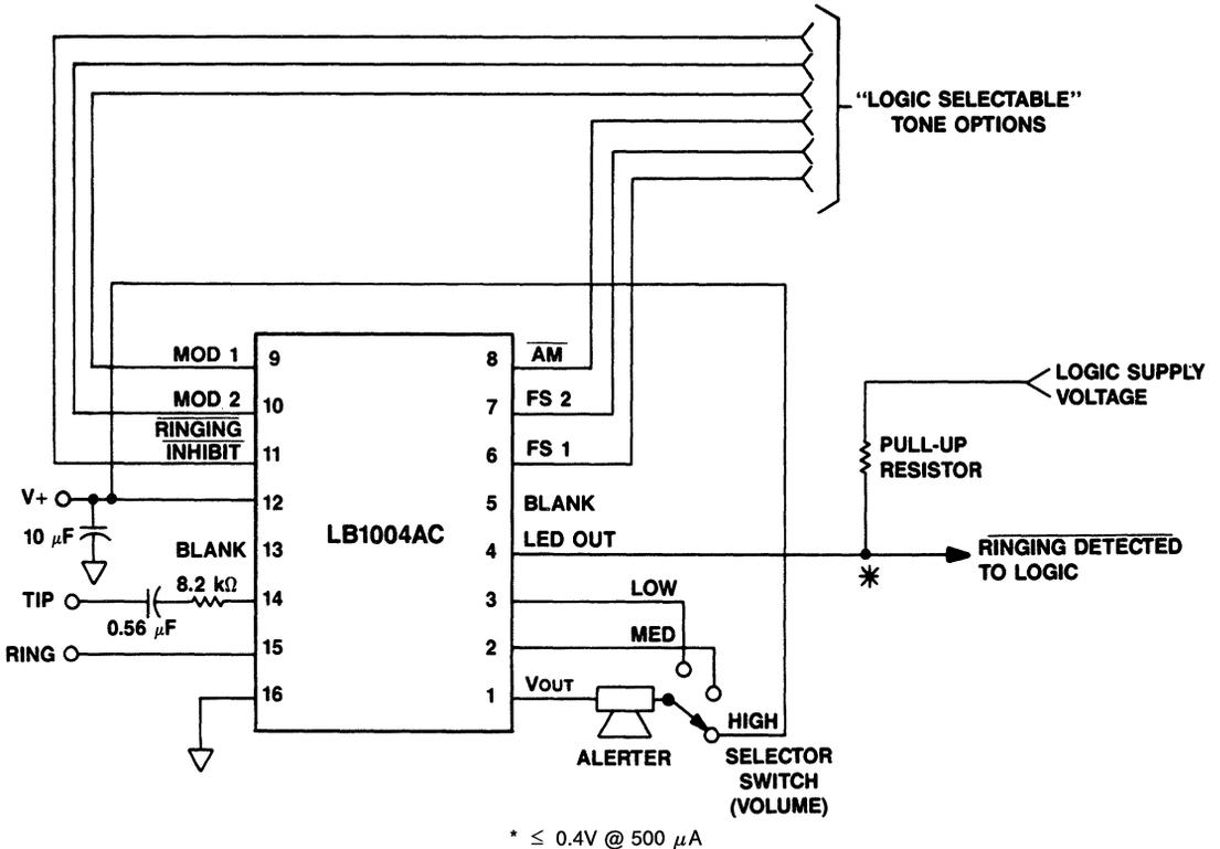
Figure 2. Typical Application for Interface Direct to Logic
