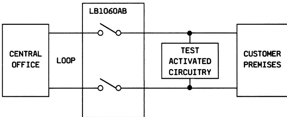
Figure 7. Block Diagram of LB1060AB Device
