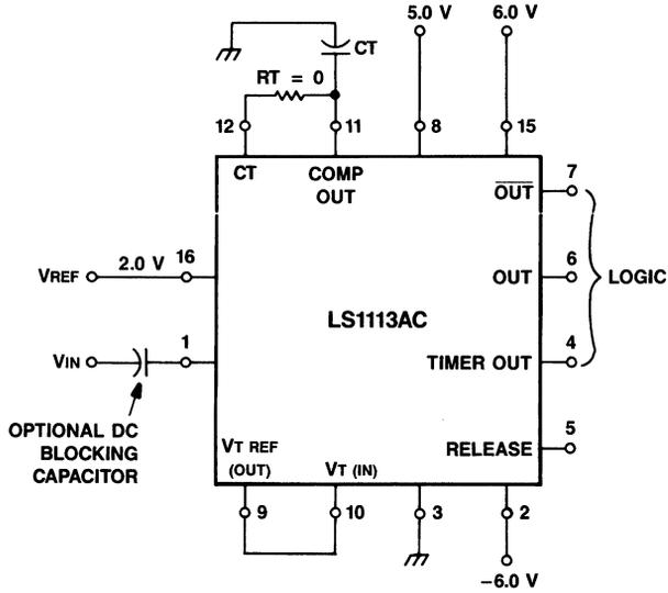
Figure 7. Typical Connections
