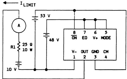
Figure 9. Output Current Limit Test
