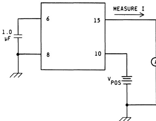
Figure 3. Microphone Bias Current
