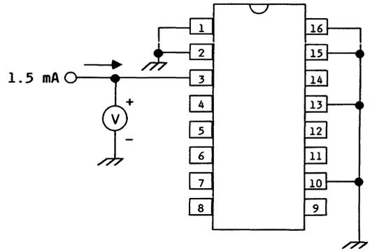
Figure 2. Breakdown Voltage ( $V_{BE0}$ ) Test Circuit
