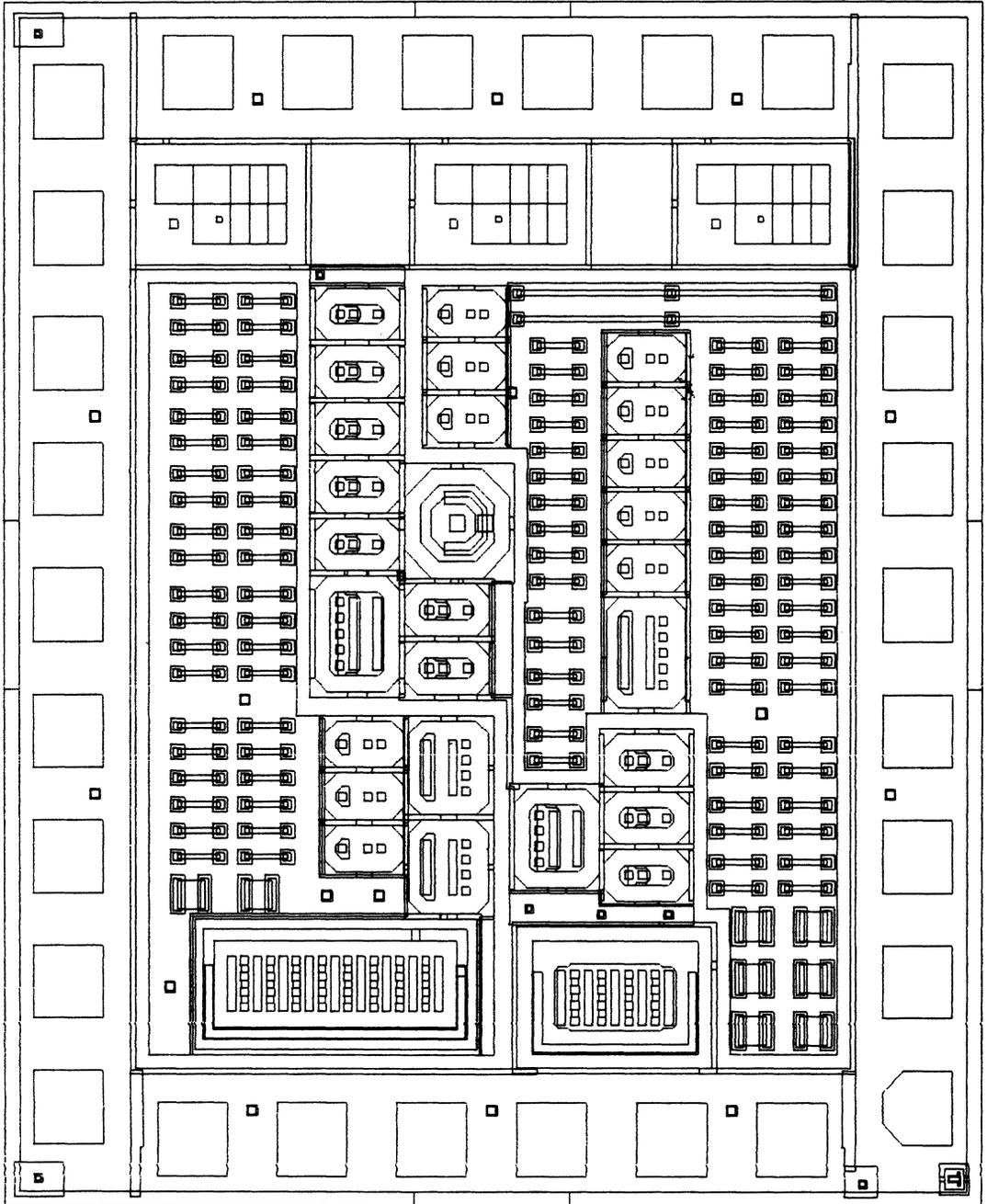
Figure 2. ALA301 High-Voltage Linear Array
