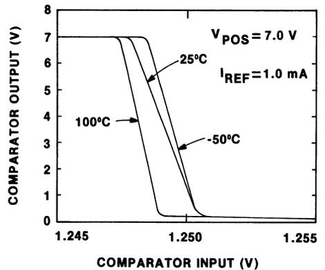
Figure 6. Typical Comparator DC Transfer Characteristics vs Temperature
