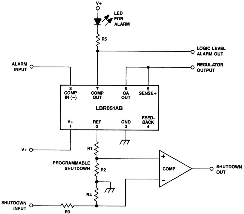
Figure 13. Regulation Control General Application Diagram
