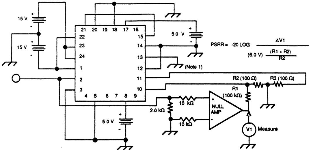
Figure 12. Power Supply Rejection Ratio Test Circuit
