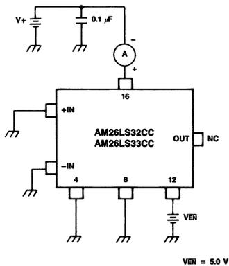
Figure 8. Power Supply Current
