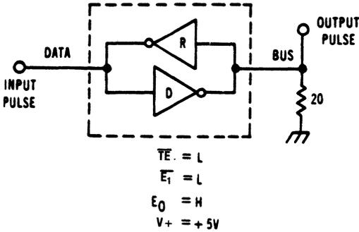
Figure 1. Driver Test Circuit
