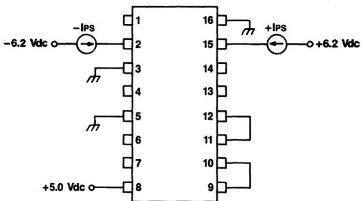
Figure 1. Positive/Negative Power Supply Current, Comparator Section
