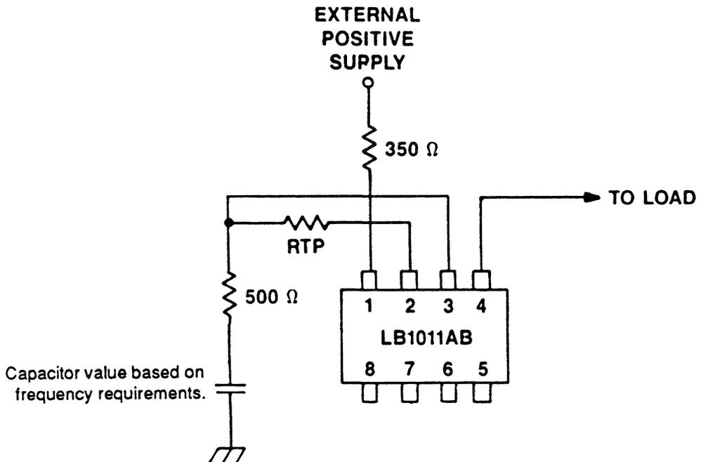
**Figure 14. Battery Feed Application (Unbalanced Configuration)**
