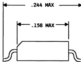
Package T—Standard 6-pin DIP (Dimensions in Inches)
