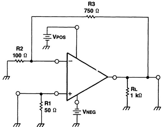
Figure 8. Slew Rate Test Circuit
