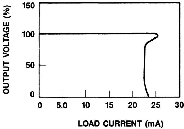
Figure 5. Typical Output Voltage vs. Load Current
