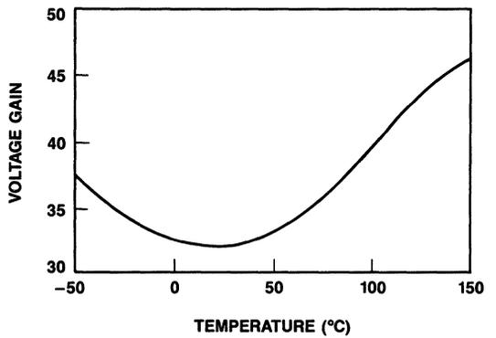
Figure 18. Typical Voltage Gain vs. Temperature
