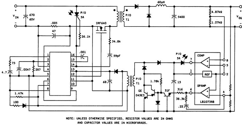
**Figure 9. dc-dc Converter Application**
