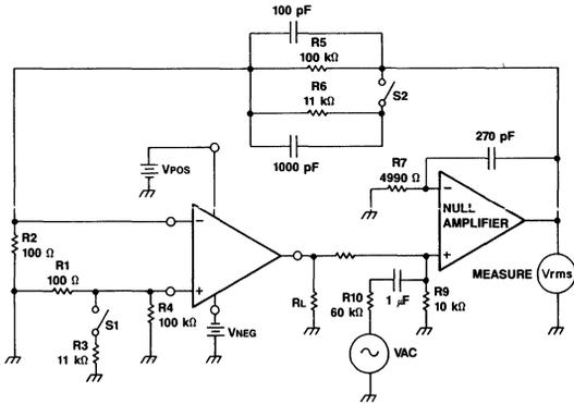
Figure 1. Open Loop Gain Test Circuit
