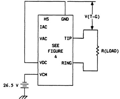
Figure 12. Test Circuit
