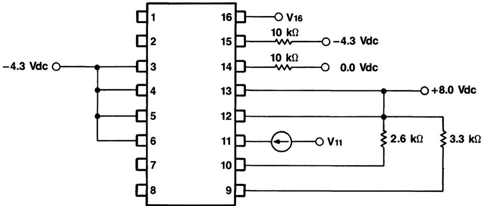
Figure 2. Input Bias Currents ( $I_{IB}$ )
