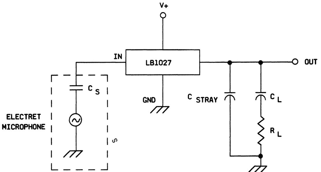
Figure 1. LB1027 Electret Preamplifier Application Diagram
