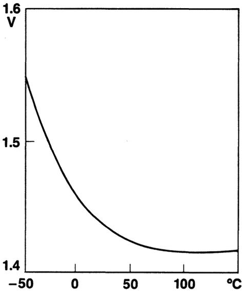
Figure 10. Output Voltage vs. Temperature
