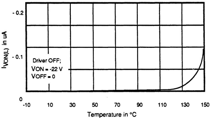
Figure 18. Typical Driver V<sub>ON</sub> Input Current (I<sub>VON(L)</sub>) vs Temperature
