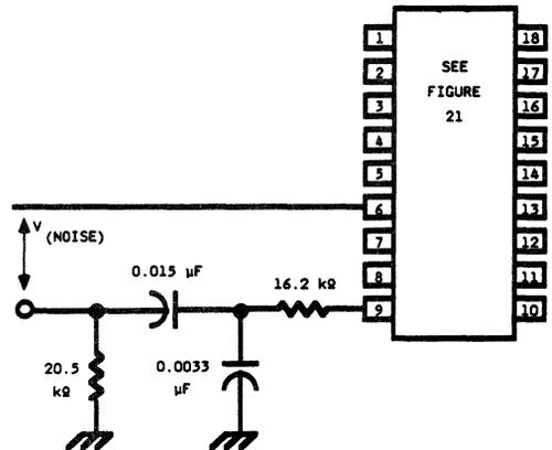
Figure 40. LB1021AD Test Circuit
