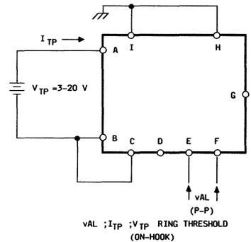
Figure 8. ON Hook ac Test Circuit
