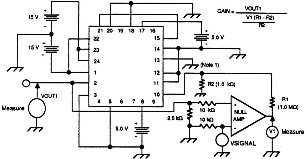
Figure 3. Open Loop Gain Test Circuit
