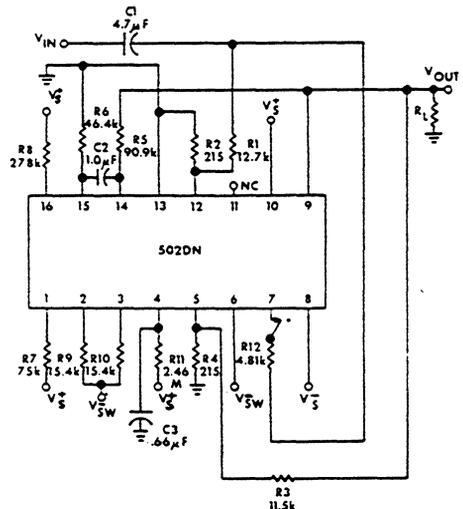
Figure 9. Typical Expander Connections
