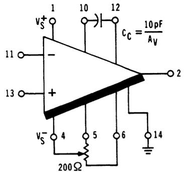
**Figure 13. High Current Output
