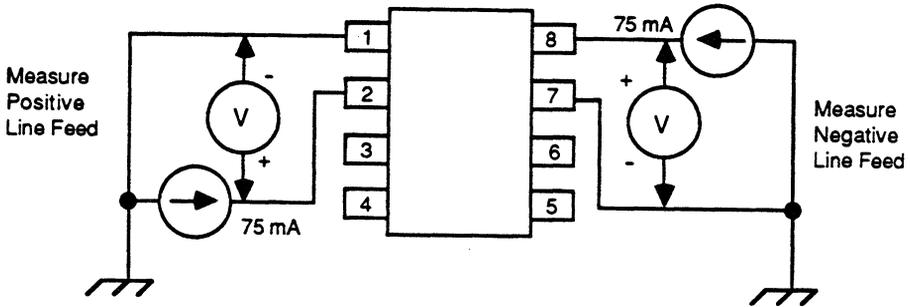
Figure 9. Supply/Cross Coupling Voltage, Test Circuit
