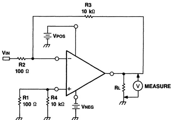
Figure 4. Output Voltage Swing Test Circuit
