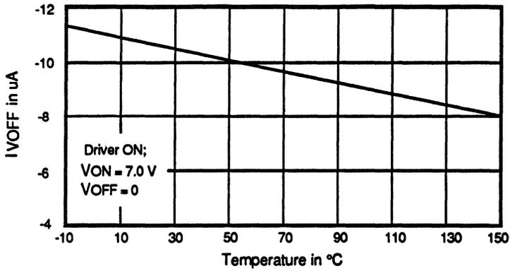
Figure 19. Typical Driver Input Current ( $I_{vOFF}$ ) vs Temperature
