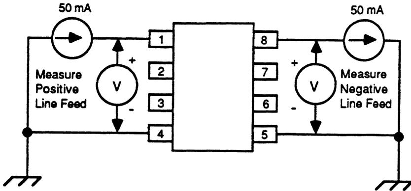
Figure 1. DC Voltage Drop, Test Circuit
