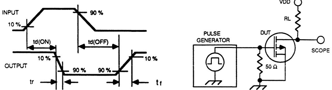
Figure 1. Switching Waveforms and Simplified Test Circuit
