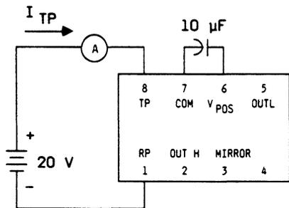
Figure 7. TP Current, No Load
