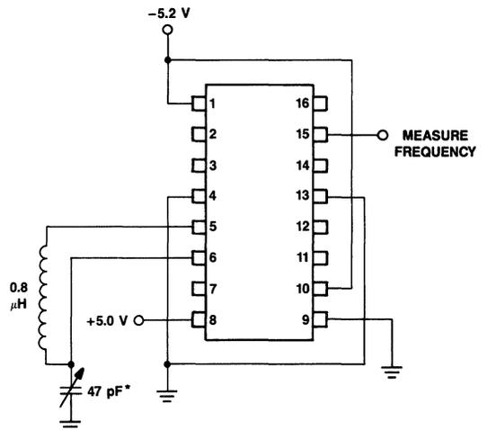
\* Capacitor should be adjusted so the resonant frequency of the tank circuit (including lead length, etc.) is nominally 20 MHz.
