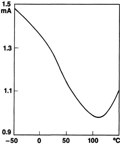
Figure 12. Supply Current vs. Temperature
