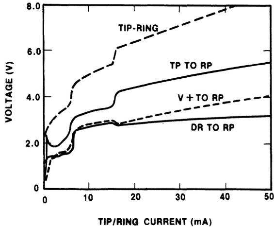
Figure 1. Typical V-I Characteristics (Dial Mode)
