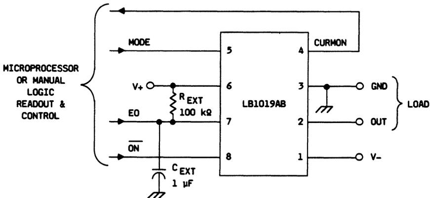
Figure 10. Typical Application Diagram for LB1019AB
