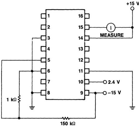
Figure 3. Positive Supply Current ( $I_{15}$ )
