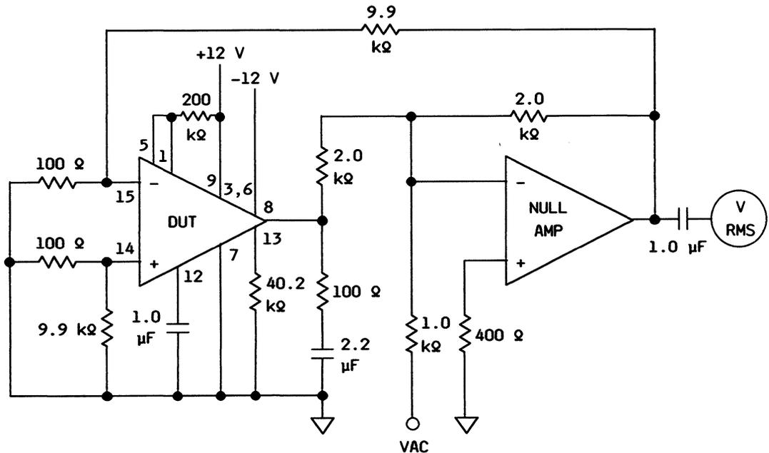
Figure 6. Open-Loop Voltage Gain Test Circuit
