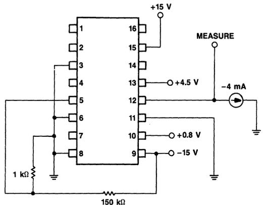
Figure 6. High-Voltage Output ( $V_{OH}$ ), ( $I_{12} = -4 \text{ mA}$ )
