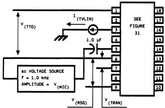
Figure 37. LB1021AD Test Circuit
