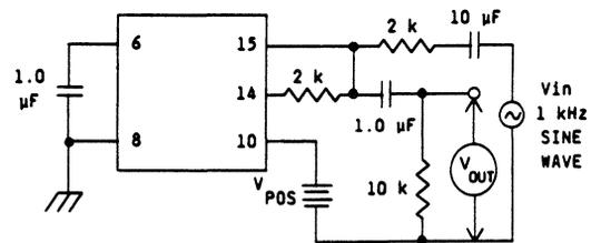
Figure 4. Microphone Bias Output Voltage Swing
