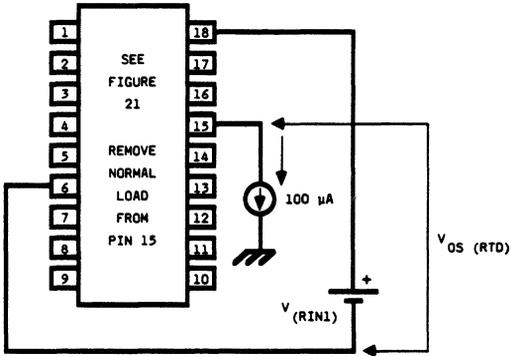
Figure 26. LB1021AD Test Circuit
