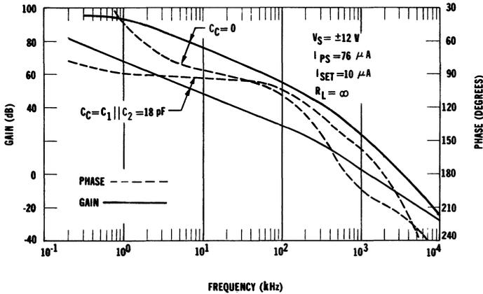
Figure 11. Open-Loop Gain and Phase vs. Frequency
