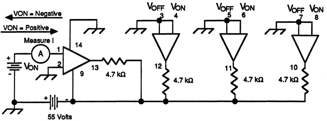
Figure 7. VON Input Current Test Circuit
