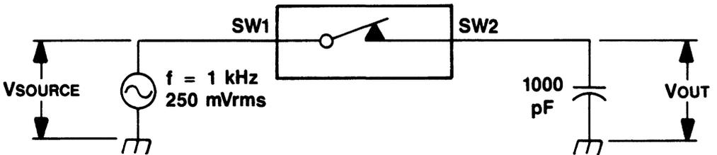
Figure 6. Harmonic Distortion Test Method
