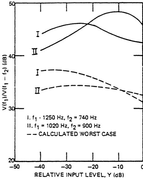
Figure 16. Intermodulation Product ( $f_1 - f_2$ ) of the Compressor
