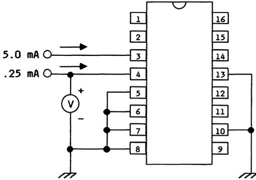
Figure 4. Saturation Voltage ( $V_{BE}$ ) Test Circuit
