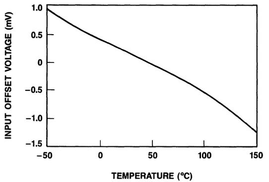
Figure 14. Typical Input Offset Voltage vs. Temperature
