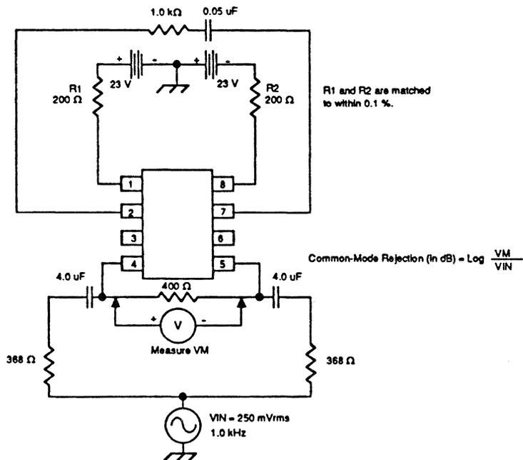
Figure 3. Common-Mode Rejection, Test Circuit
