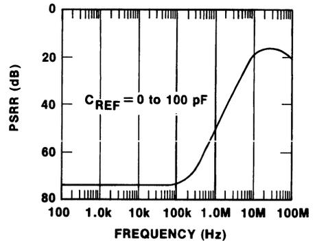
Figure 4. Precision Low-Voltage Reference Power-Supply Rejection Ratio Frequency Characteristics
