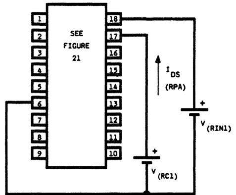
Figure 25. LB1021AD Test Circuit
