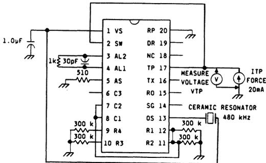
Figure 8. Voltage (TP-to-RP), Dial
