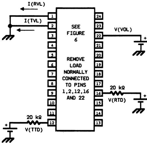
Figure 11. LB1020AF Test Circuit
