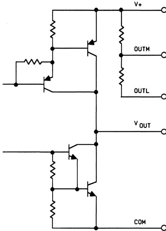
Figure 8. Simplified Tone Ringer Output Diagram
