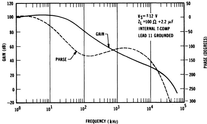
**Figure 9. Open-Loop Gain and Phase vs. Frequency**
