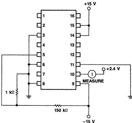
Figure 5. Strobe Leakage Current ( $I_{10}$ )
