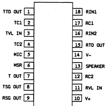
Figure 3. LB1021AD 18-Pin Plastic DIP
