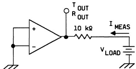
Figure 2. Output Leakage Current, (The current through  $V_{LOAD}$  is the leakage current)
