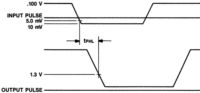
Figure 2. Negative Input and Output Waveforms
