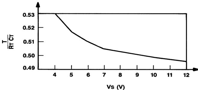
**Figure 6. Ratio of Ramp Generator Period (T) to  $R_T C_T$  Time Constant vs. Supply Voltage**
