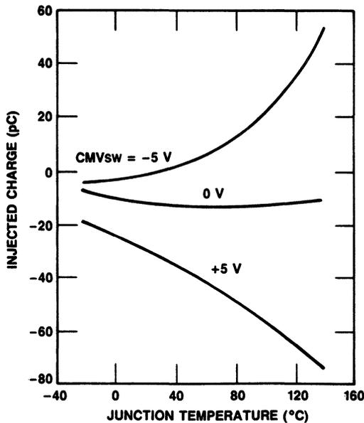
Figure 17. Typical Injected Charge vs. Temperature
