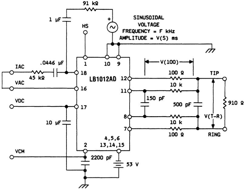
Figure 18(b). Frequency Response Test Circuit
