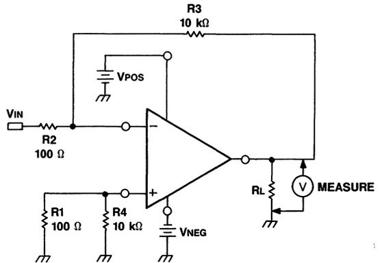
Figure 4. Output Voltage Swing Test Circuit
