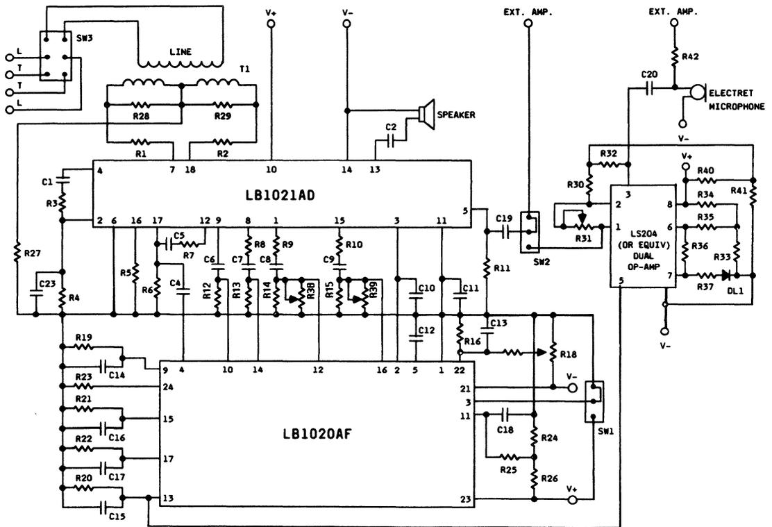
**Figure 42. Typical Speakerphone Line-Coupled Application**
