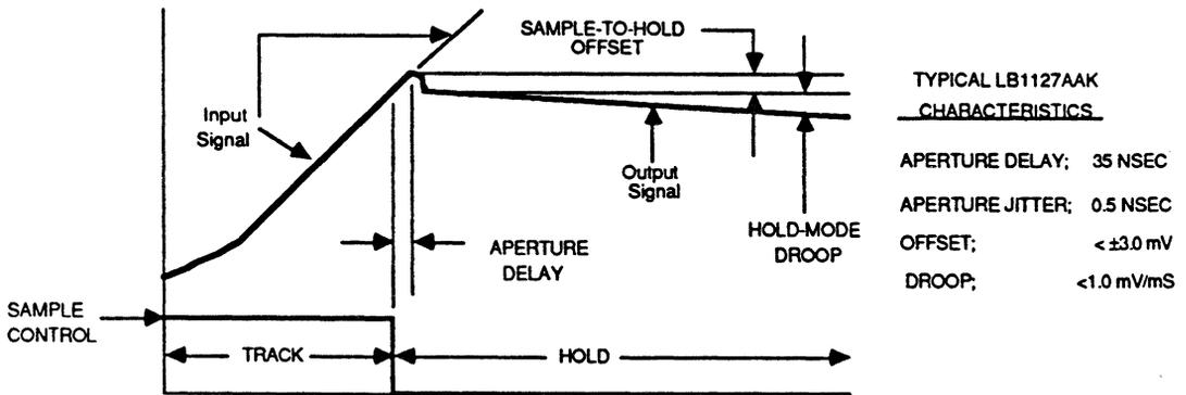
Figure 15. Several Sample-Hold Characteristics
