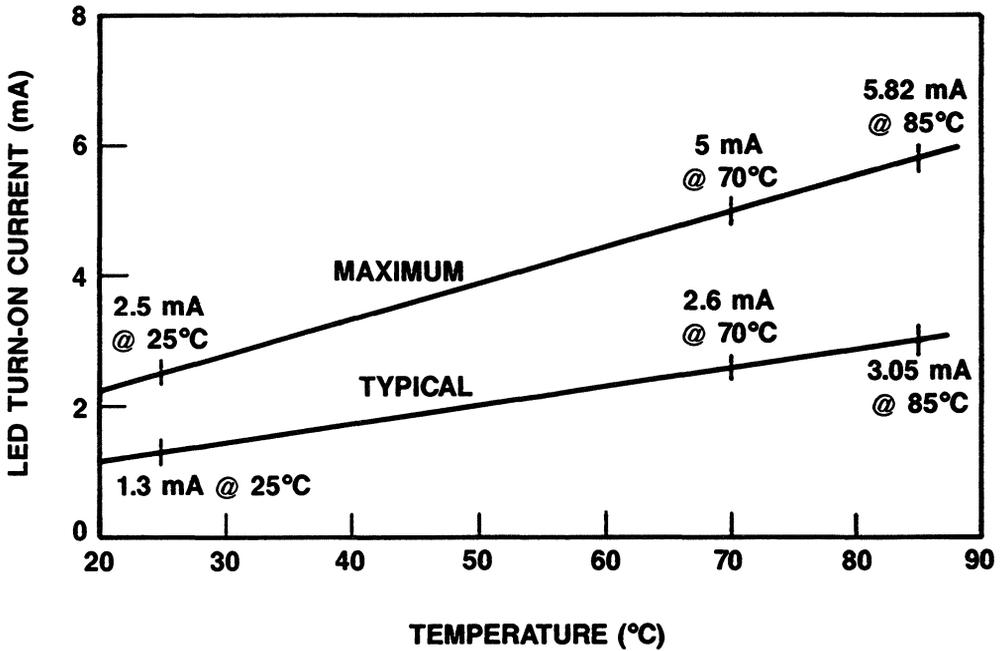
Figure 2. LED Turn-On Current vs. Temperature (°C)
