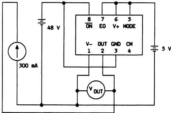
Figure 6. Output Voltage Test
