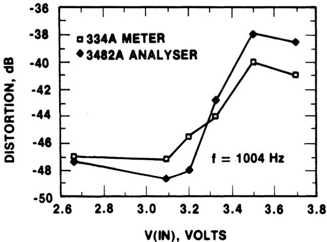
Figure 21(a). Typical Distortion vs Input Characteristics
