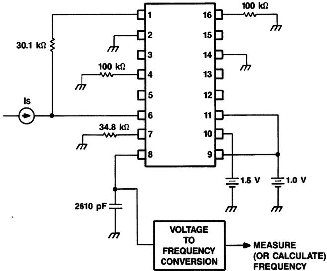
**Figure 5. Ramp Generator Frequency Test Circuit**
