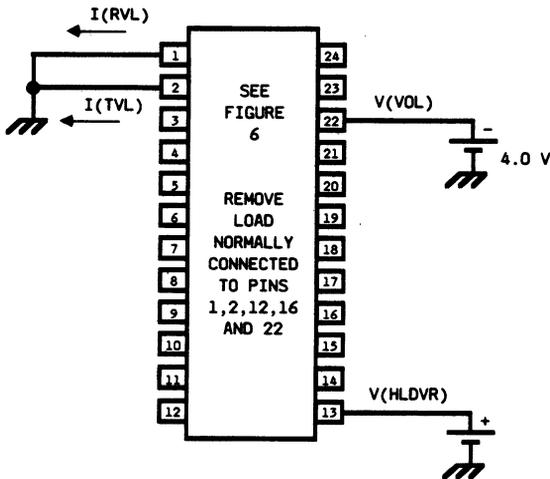
Figure 13. LB1020AF Test Circuit
