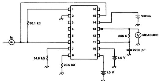
Figure 3. Sense Amplifier Output Voltage Test Circuit
