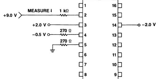
Figure 6. Output Leakage Current (+Vs = +2 V and -Vs = -2 V)
