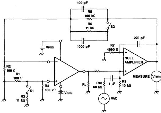
Figure 1. Open Loop Gain Test Circuit
