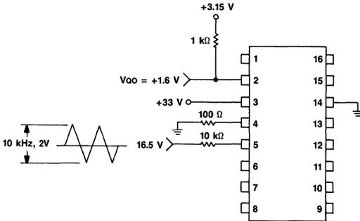
Figure 1. Input Offset Voltage; Input Bias Current; Input Offset Current (+Vs = 33 V and -Vs = 0 V)
