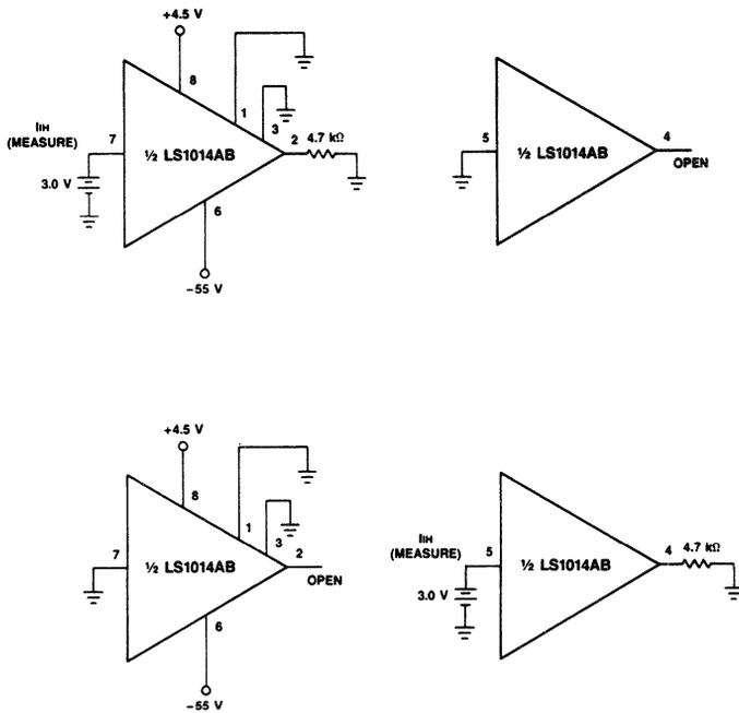
Figure 6. Logic Input Current, On
