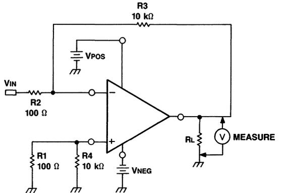
Figure 4. Output Voltage Swing Test Circuit
