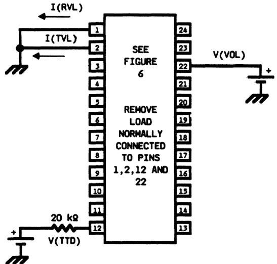
Figure 10. LB1020AF Test Circuit
