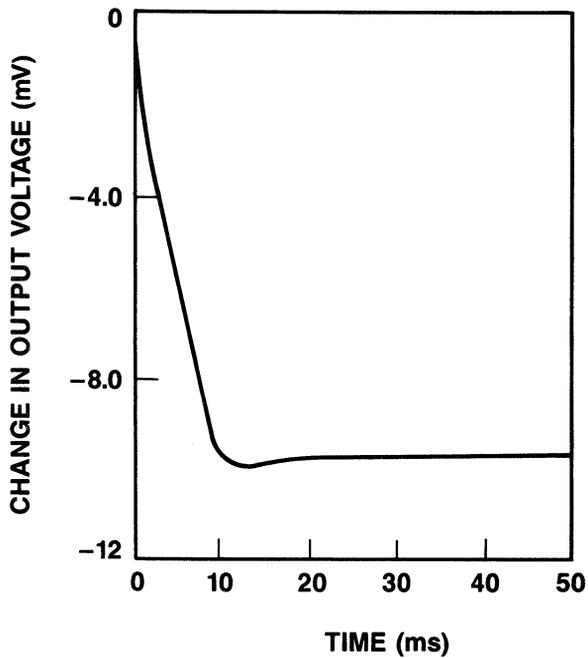
Figure 4. Typical Output Step Response
