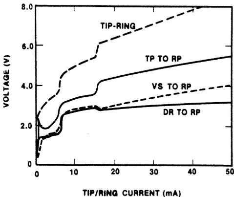
Figure 1. Typical V-1 Characteristics (Dial Mode)
