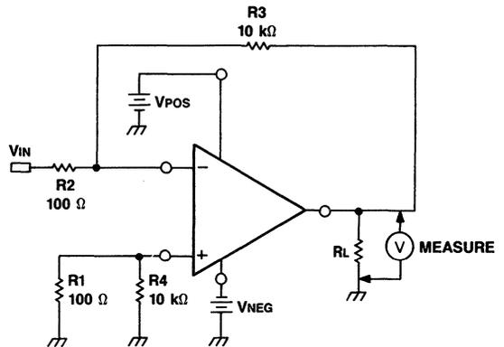
Figure 4. Output Voltage Swing Test Circuit
