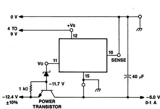
**Figure 10. Negative 6.0 V Application Using the LB1081CC 6 V Reference**
