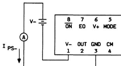
**Figure 4. Power-Supply Current**
