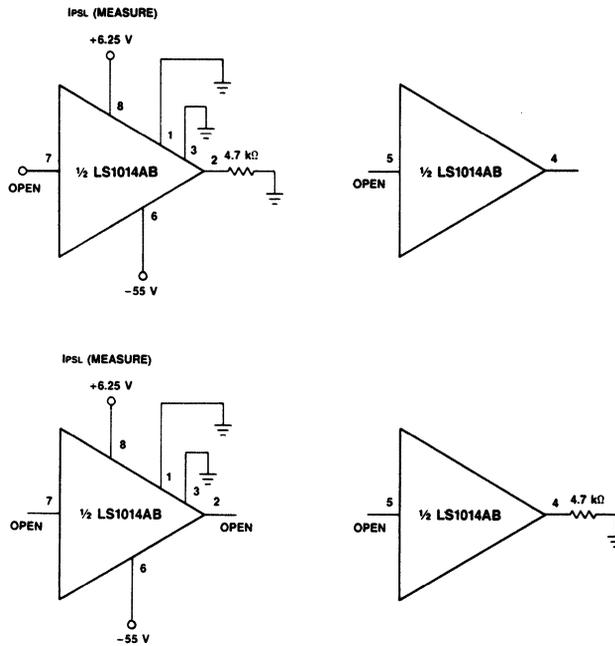
Figure 4. Logic Supply, Current On
