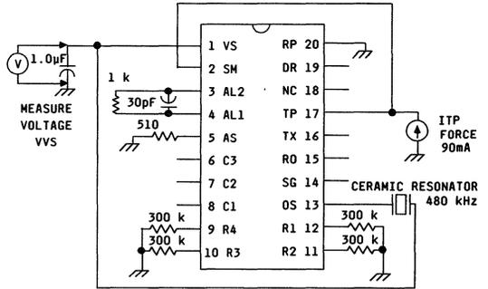
Figure 7. Voltage (VS-to-RP), Speech
