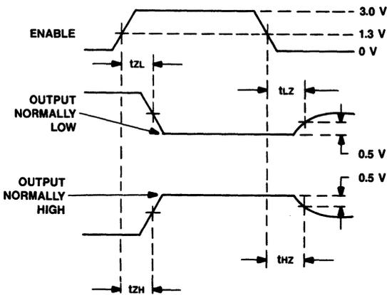
Figure 11. ENABLE and Output Waveforms
