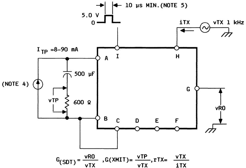
**Figure 4. OFF Hook ac Test Circuit 1**
