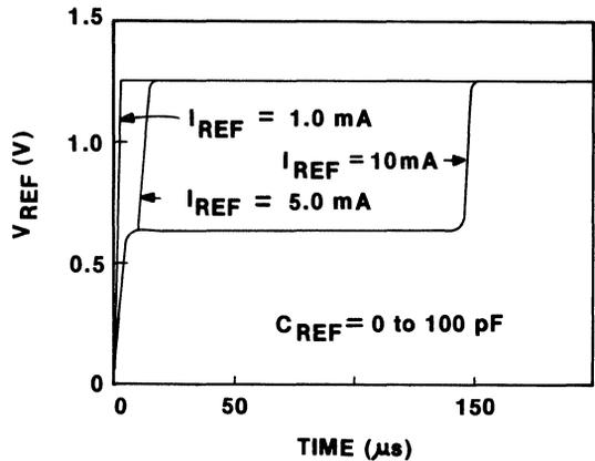
Figure 2. Precision Low-Voltage Reference Transient Start-Up Time
