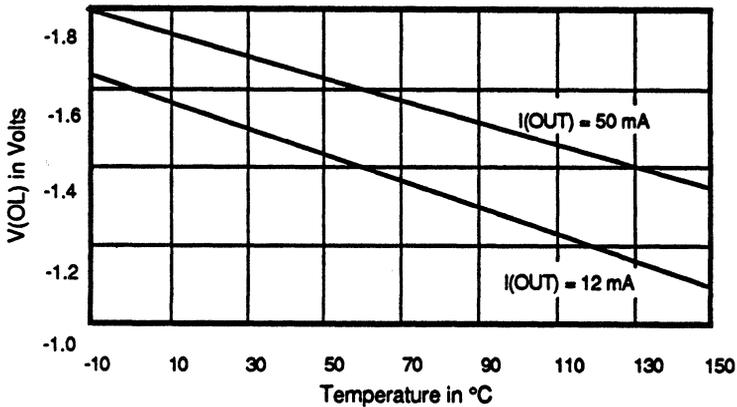
Figure 21. Typical Driver Output ON Voltage ( $V(OL)$ ) vs Temperature
