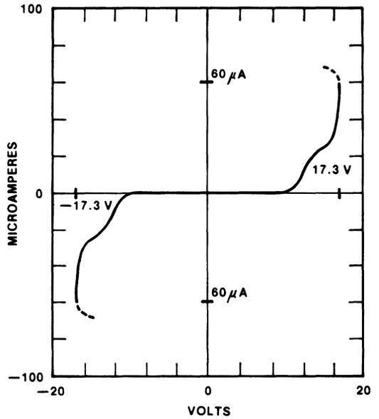
Figure 6. Low Current Characteristics
