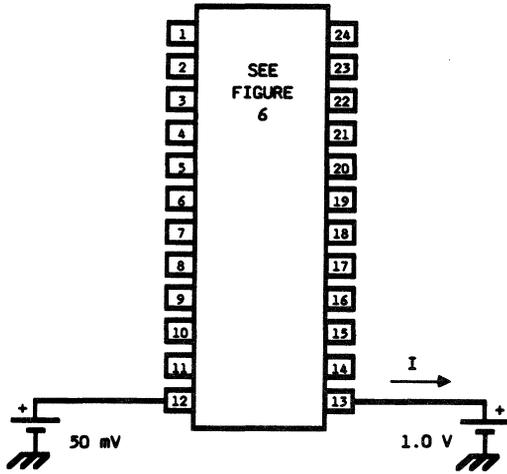
Figure 15. LB1020AF Test Circuit
