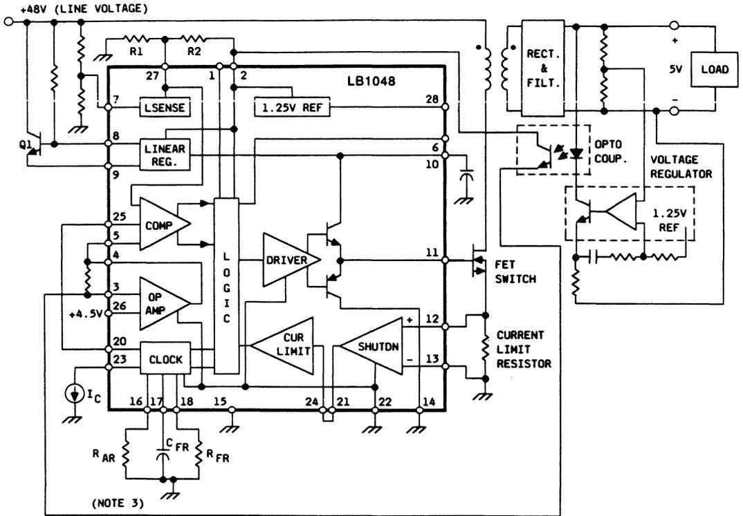
Figure 9. Application Diagram
