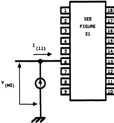
Figure 24. LB1021AD Test Circuit
