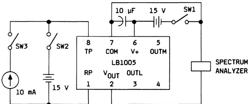
Figure 6. Test Circuit (Output Frequency and Modulation Rate)
