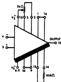
**Figure 12. 1031AC Offset Null Feedback Compensation**
