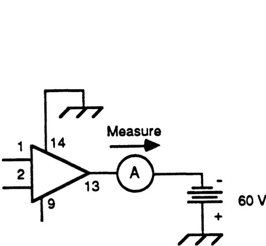
Figure 11. Reverse Leakage Current, Output Diode D1 Test Circuit
