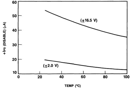
Figure 10. Temperature vs. Power Supply Current (Disabled) at Various Supply Voltages
