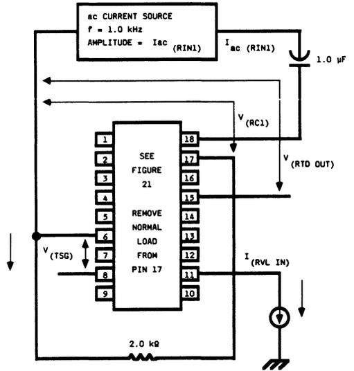
Figure 31. LB1021AD Test Circuit
