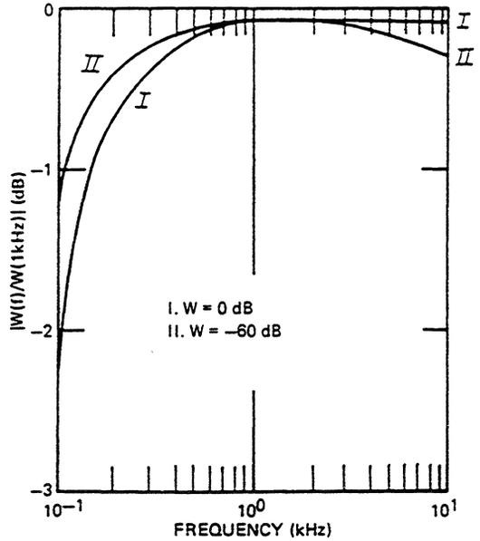
Figure 13. Frequency Response of the Expander
