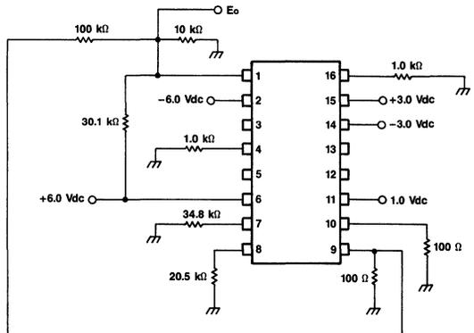
Figure 4. Input Offset Voltage Test Circuit
