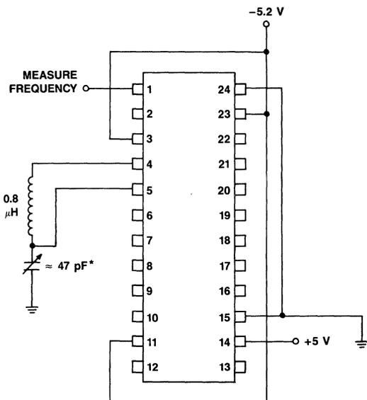
\* Capacitor should be adjusted so the resonant frequency of the tank circuit (including Lead length, etc.) is nominally 20 MHz.
