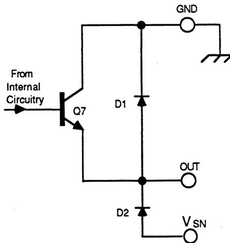
Figure 2. LS1098AAF Simplified Output Diagram
