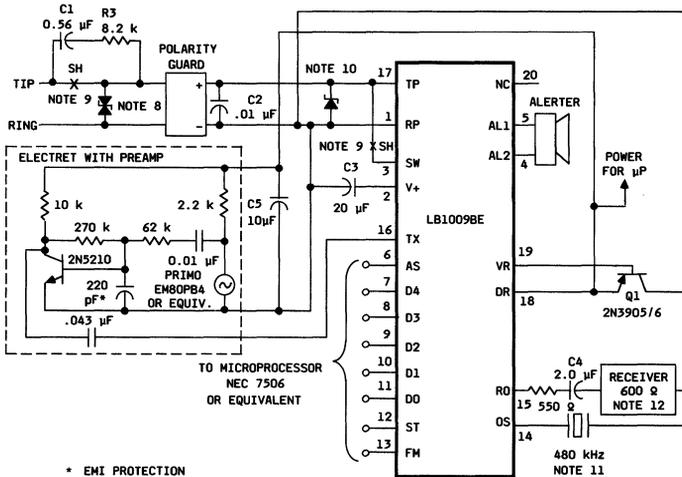
Figure 10b. Typical Application Diagram
