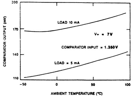
Figure 12. Typical Temperature Characteristics
