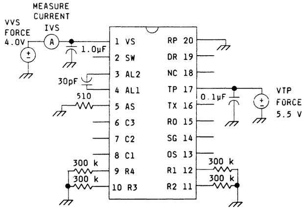
Figure 3. VS Current (Ring Detect)
