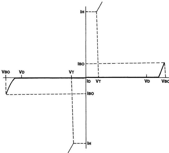
Figure 1. Typical Electrical Characteristics
