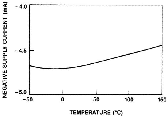
Figure 9. Typical Negative Supply Current vs. Temperature
