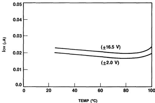
Figure 11. Temperature vs. Output Current (High) at Various Supply Voltages
