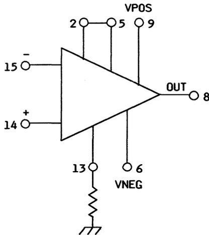
**Figure 4. External Bias Setting Internal Feedback Compensation**
