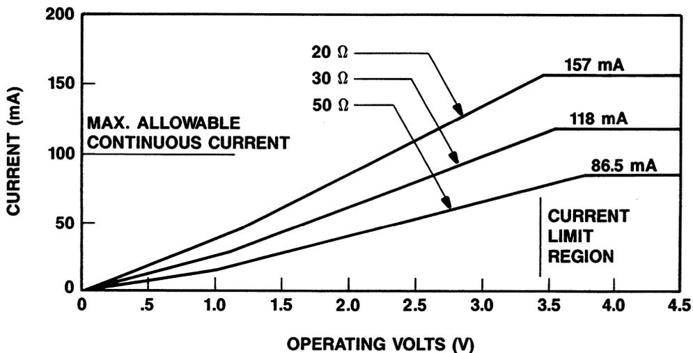
Figure 5. Output I/V Characteristics for Various Ron @ 70°C
