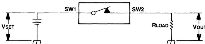
**Figure 3. Test Method for Switching Time and Switch Offset Voltage**
