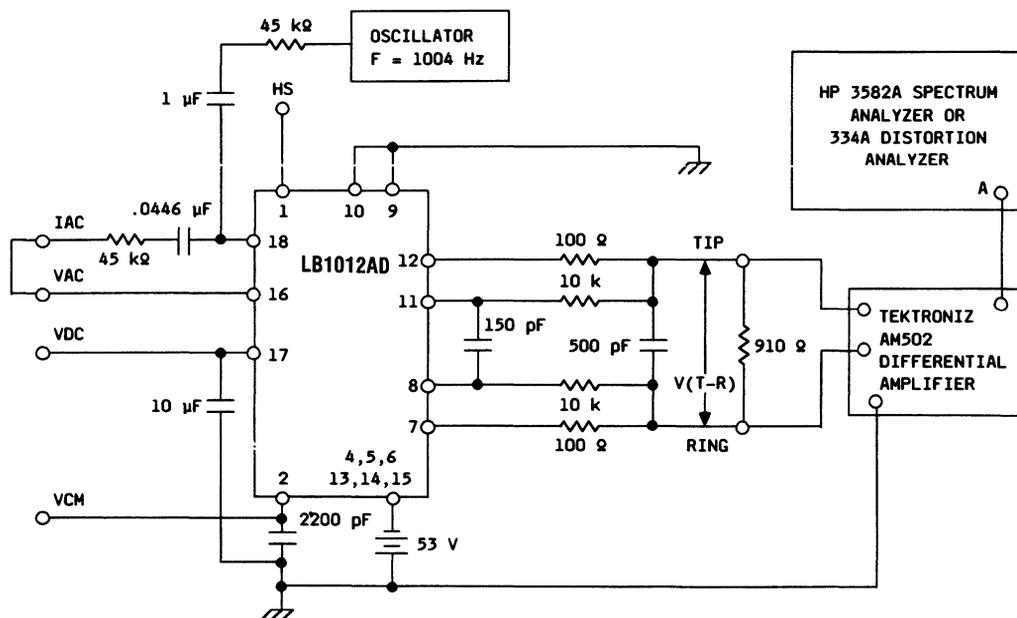
Figure 21(b). LB1012AD Distortion Test Circuit
