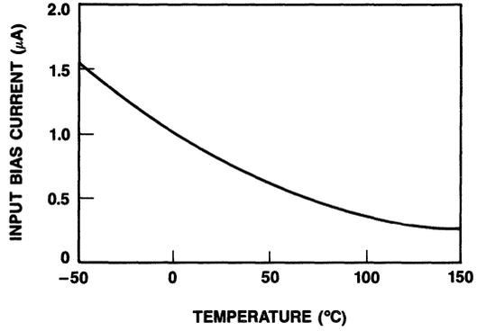
Figure 16. Typical Darlington Input Bias Current vs. Temperature
