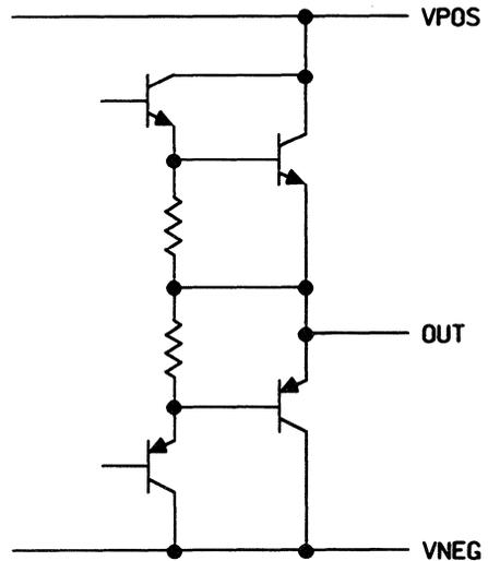
Figure 2. Simplified Output Diagram
