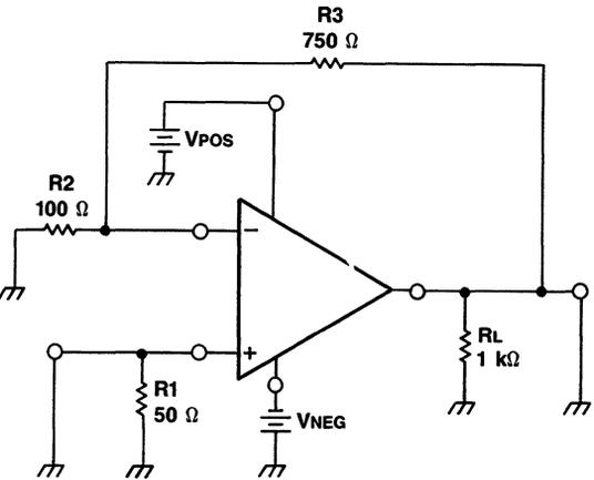
Figure 8. Slew Rate Test Circuit
