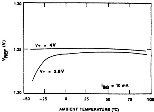
Figure 5. Precision Low-Voltage Reference Start-Up Characteristics
