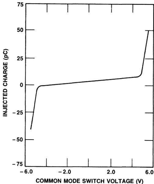
Figure 9. Typical Injected Charge vs. Common-mode Voltage
