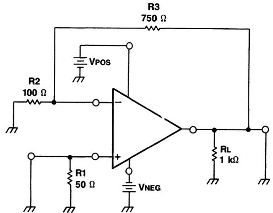
Figure 8. Slew Rate Test Circuit
