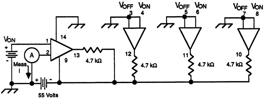
Figure 8. VOFF Input Current Test Circuit
