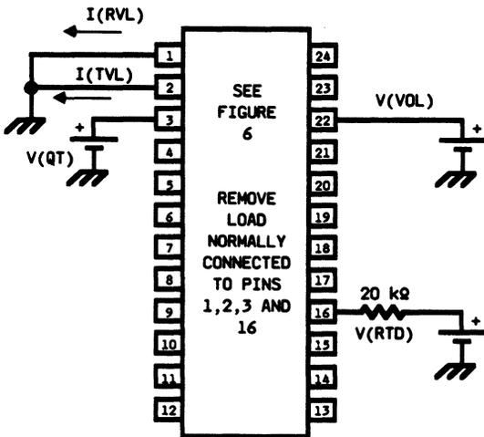
Figure 9. LB1020AF Test Circuit
