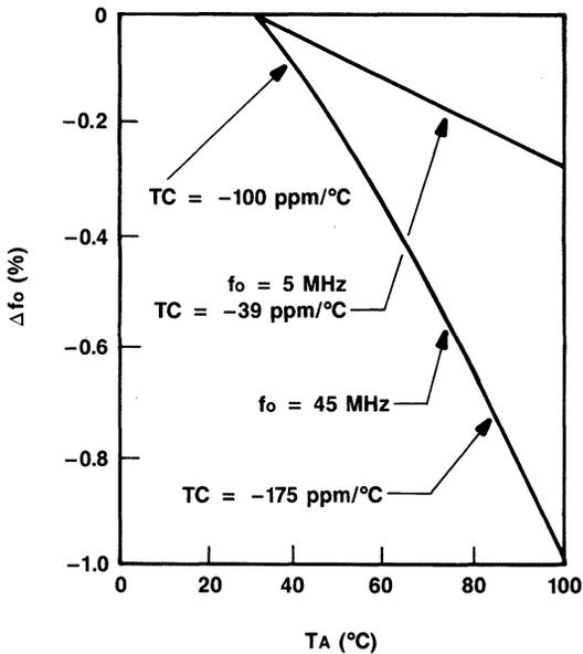
Figure 4. Typical Temperature Coefficient
