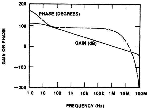
Figure 5. Gain/Frequency Response Curve
