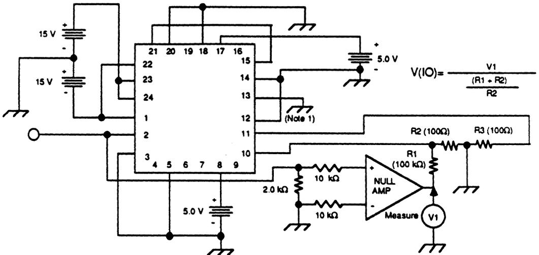
Figure 8. Input Offset Voltage Test Circuit
