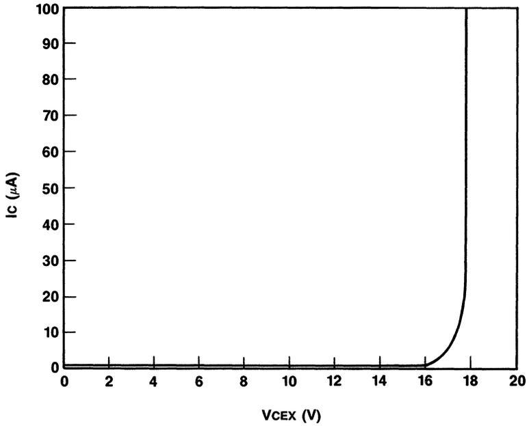
Current vs. Breakdown Voltage (PNP 1X)
