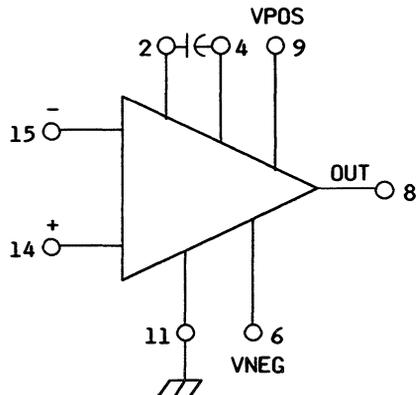
**Figure 5. Internal Bias Setting External Feedback Compensation**
