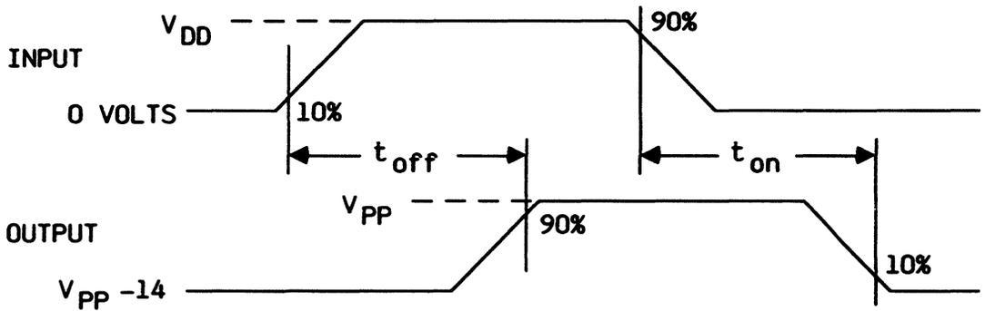
Figure 1. Switching Waveforms
