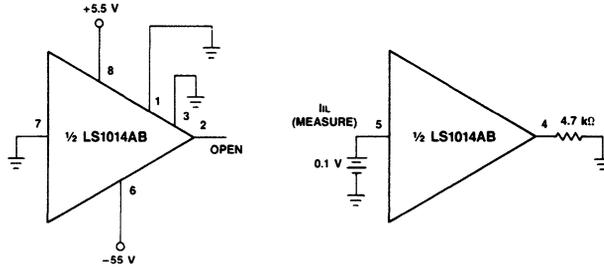
Figure 7. Logic Input Current, Off
