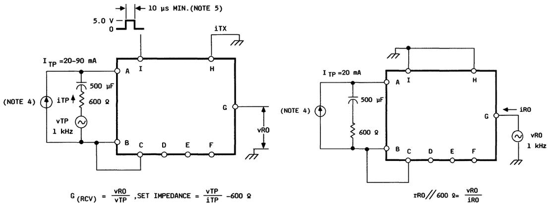
**Figure 5. OFF Hook ac Test Circuit 2**
