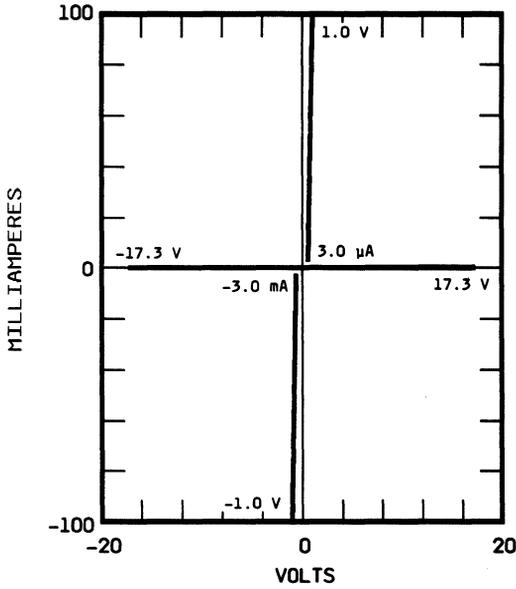
Figure 5. High Current Characteristics
