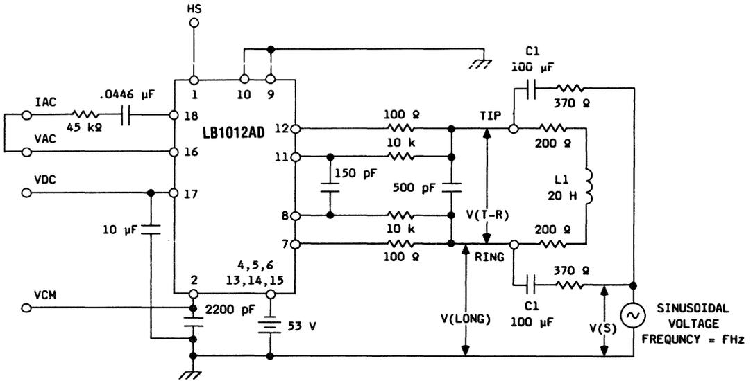
Figure 19(b). Longitudinal Balance Test Circuit
