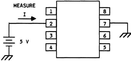
Figure 3. Leakage Tests
