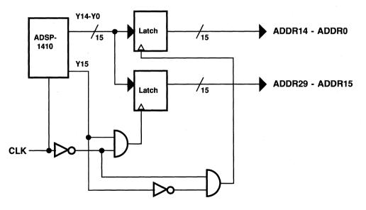
Figure 9.1 Single-Chip Connections to 30-Bit Address Bus
