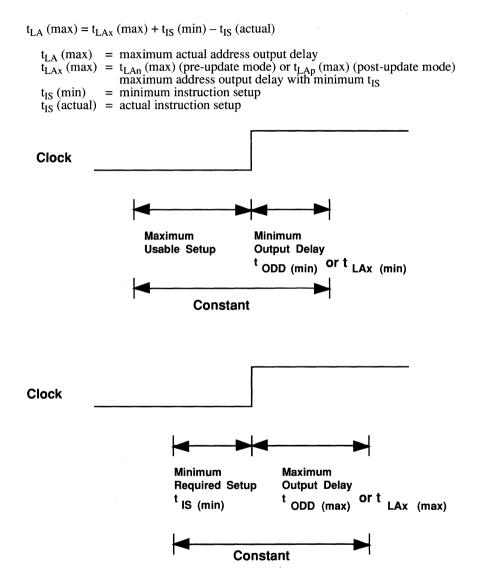
Figure 10.2 Sliding Window Timing
