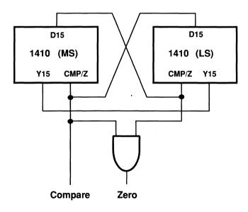
Figure 9.2 Two-Chip Cascade Connections
