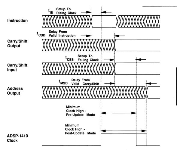
Figure 9.3 Minimum Clock Period For Two-Chip/Double-Precision Mode
