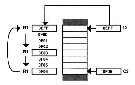
Figure 8.2 Reinitialization to Form Circular Buffer
