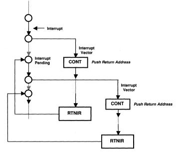
Figure 4.4 Pending Interrupt on Return From Service Routine
