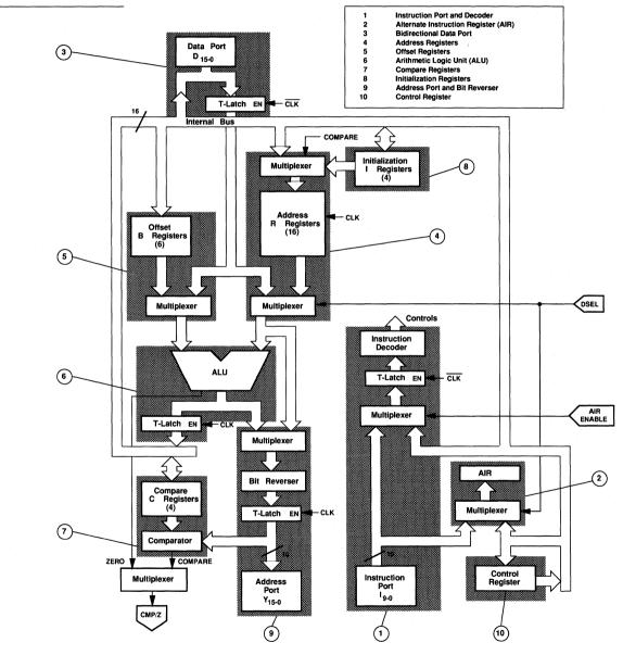
Figure 7.1 ADSP-1410 Block Diagram
