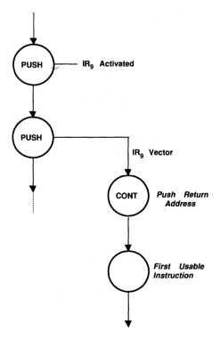
Figure 4.7 Three Pushes On Stack Overflow
