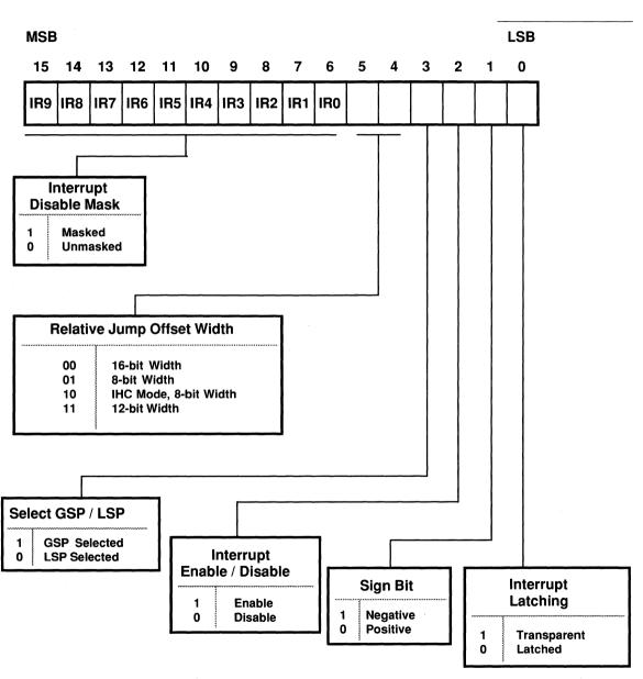
and clear all bits at once or individually, using dedicated instructions. The ADSP-1401 also writes the  $SR_1$  bit during the execution of instructions that decrement counters. You can load or read the entire status register from the data port. You can also save and restore the status register to and from the subroutine stack. The reset operation clears the entire status register.
