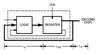
f<sub>max</sub> External Feedback; 1/(t<sub>s</sub> + t<sub>co</sub>)
