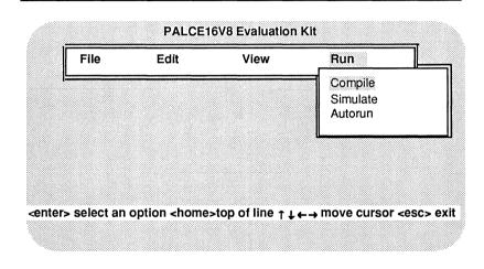
PALASM software offers you a time saving autorun feature that combines the compile and Simulation processes into one keystroke. The autorun procedure follows.
