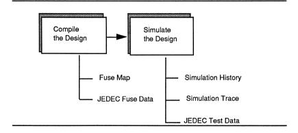
Now that you have an overview of the procedure, you can begin processing the decoder design. Proceed to Autorun Compile and Simulate.
