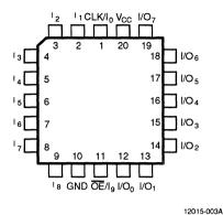
Note: Pin 1 is marked for orientation
