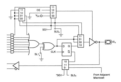
\*In macrocells MC<sub>0</sub> and MC<sub>7</sub>, SG1 is replaced by SGO on the feedback multiplexer.
