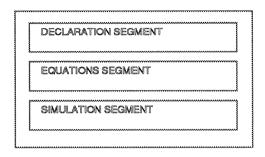
The PALASM design file is also known as the PDS (PAL device Design Specification) file.
