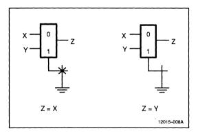
Figure 5. PAL Device Multiplexer
