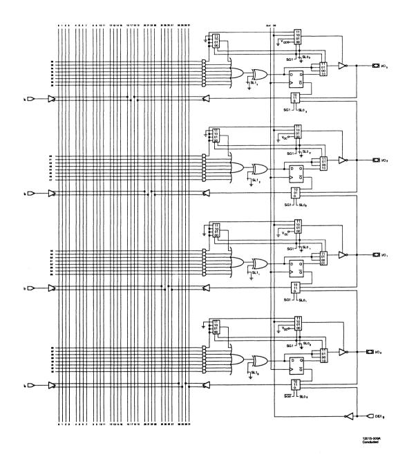
Figure 6. PALCE16V8 Logic Diagram
