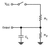
**Switching Test Circuit**
