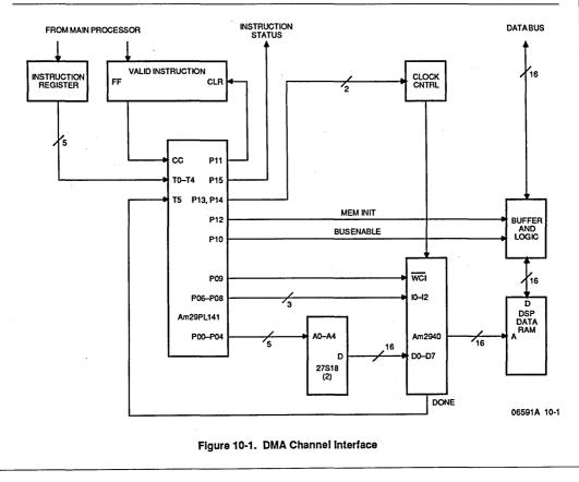
data buses. Finally, two bits (P[13], P[14]) are used to control the clock source to the Am2940 address generator. P[15] signals the main CPU when the execution of a command is complete.
