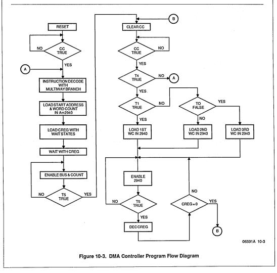
into the Am2940s. This parallel operation allows the data transfers to take place with a minimum of overhead. By the time the instruction is decoded, the Am2940 data and control registers are loaded and ready to start the transfer operation.
