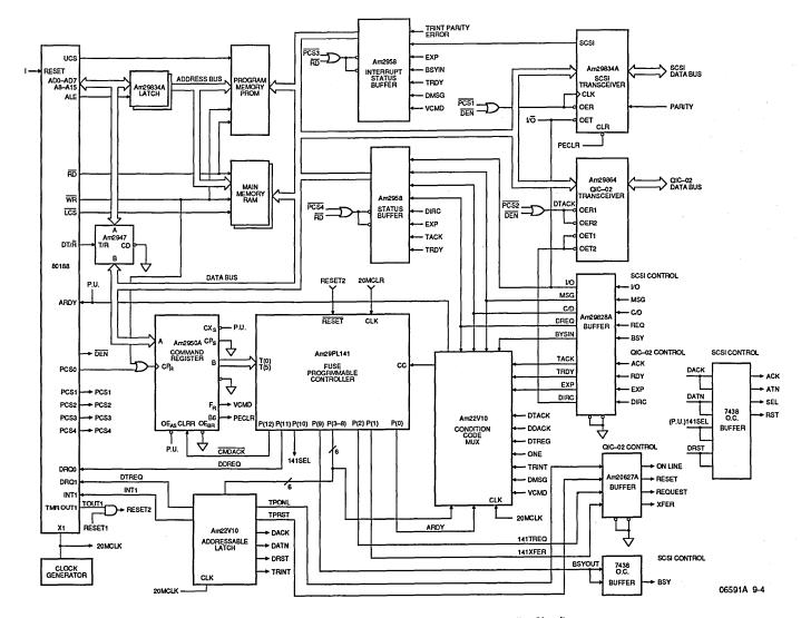
Figure 9-4. Am29PL141 QIC-02 and SCSI Controller Circuitry
