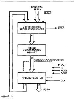
Figure 1-1. Am29PL141 Block Diagram
