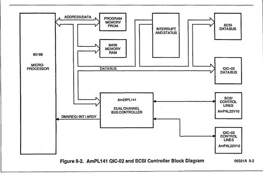
interface and as an "Initiator" to a SCSI system. This design is composed of three main functional blocks: Microprocessing Unit, Dual Channel Bus Controller, I/O Bus Interface.
