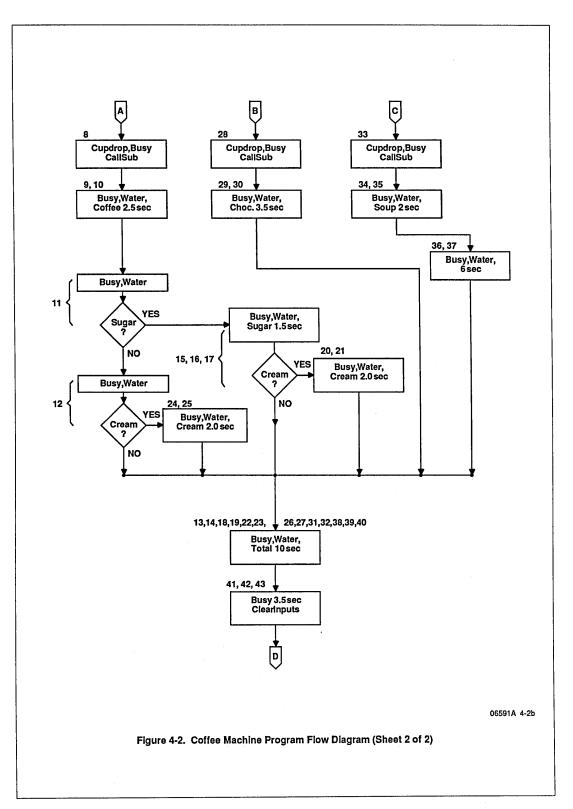
Special care needs to be taken to ensure that water is on continuously for 10 seconds. Six possible paths lead to the microcode line labeled "last". At the end of each of these paths, the CREG is loaded with a value equal to 10 seconds minus the time in seconds for which water has already been on. Note that the value loaded into the CREG is one less than the expected value. This is because the value 0 in the CREG needs to be accounted for as the Am29PL141 checks the CREG and then decrements.
