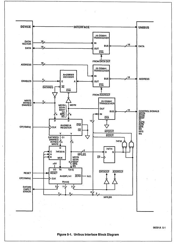
implement the Unibus request/grant handshaking. Because the clock period must be at least 64.5 ns, a clock frequency of 15 MHz is appropriate (66.6 ns). A detailed control logic timing analysis is shown in Figure 5-2.
