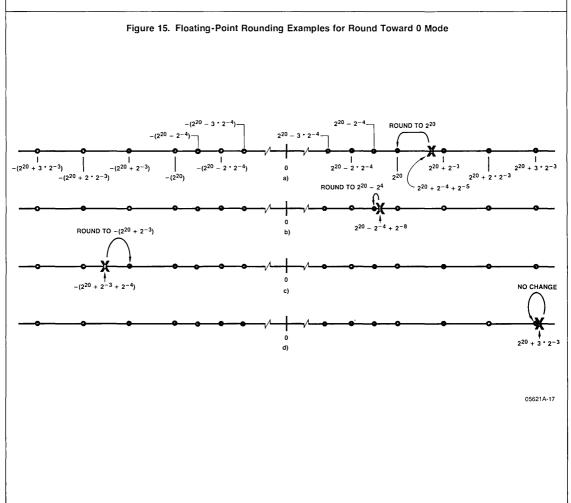
Figure 16 illustrates four examples of the round toward 0 process for operations having an integer destination format. The infinitely precise result of an operation is represented by an X on the number line; the black dots on the number line indicate those values that can be exactly represented in the integer format.
