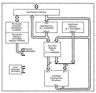
Figure 3: Am29300-based array processor.
