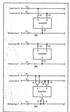
4. Three programmable I/O bus modes permit the floating-point processor to operate with dual 32-bit input buses (a), a single, shared 32-bit input bus (b), or even two 16-bit buses (c) so that it can easily connect to most 16-bit microprocessor systems.
