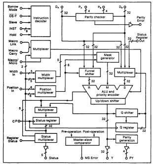
2. To connect its various internal functional blocks, the Am29332 ALU employs a 32-bit bus. Among the chip's major features are a 64-bit funnel shifter, parity checking and generation, and a basic 32-bit ALU that has three input ports. The processor also has three 32-bit ports through which it transfers data into and out of the chip.
