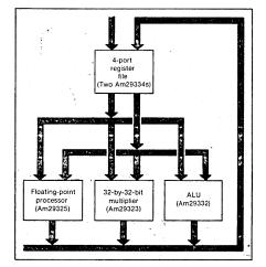
The 32-bit multiplier and the 32-bit floating-point processor can be used together in a system. Either chip also functions without the other if just one of the capabilities is needed.
