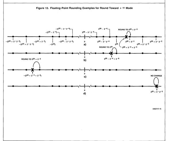
Figure 14 illustrates four examples of the round toward  $+\infty$  process for operations having an integer destination format. The infinitely precise result of an operation is represented by an X on the number line; the black dots on the number line indicate those values that can be exactly represented in the integer format.
