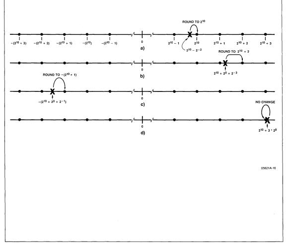
**Round Toward 0** – In this rounding mode the result of an operation is rounded to the closest representation whose magnitude is less than or equal to the infinitely precise result, and which fits the destination format. Rounding is performed both for floating-point and integer destination formats.
