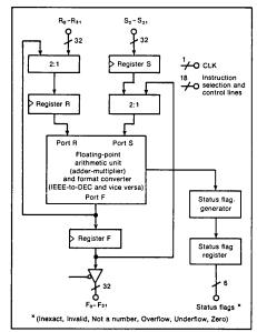
3. Also using separate 32-bit buses for the inputs and output, the AM29325 floating-point processor handles either IEEE or DEC formatted data and can translate between formats, if necessary.
