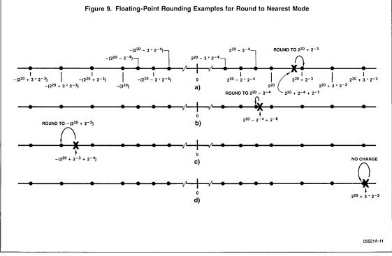
Figure 10 illustrates four examples of the round to nearest process for operations having an integer destination format. The infinitely precise result of an operation is represented by an X on the number line; the black dots on the number line indicate those values that can be represented exactly in the integer format.
