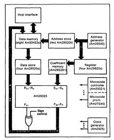
5. To build a fast-Fourier transform processor that uses the floating-point processor as its heart requires only a few control chips and some memories. Use of the Am29540 and Am29332 LSI building blocks helps keep the circuitry simple.
