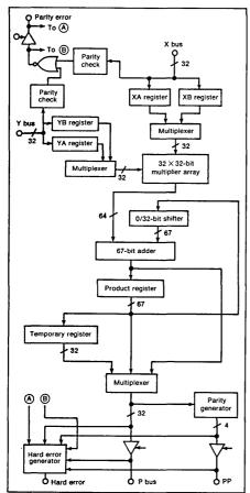
Surrounding the 32-by-32-bit multiplier array on the Am29323 are multipliers for the two 32-bit input buses, which permit 64-bit multiplications to be done in just four cycles. The multiplier checks parity on the input data and generates parity bits for the output result.
