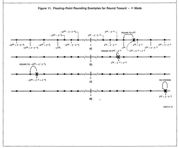
Figure 12 illustrates four examples of the round toward  $-\infty$  process for operations having an integer destination format. The infinitely precise result of an operation is represented by an X on the number line; the black dots on the number line indicate those values that can be exactly represented in the integer format.
