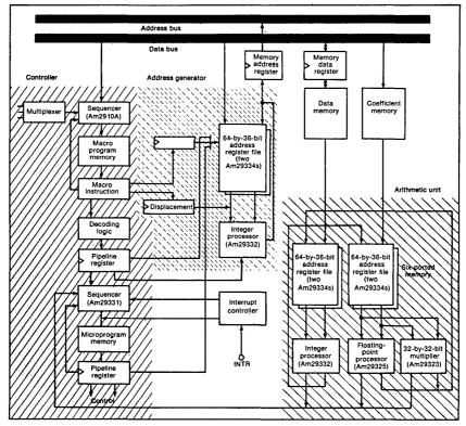
6. A versatule, yet high-performance microprogrammable system can be built by including both the floating-point processor and the 32-bit multiplier into a system that uses the other Am29300 building blocks to form the control and address generation sections.
