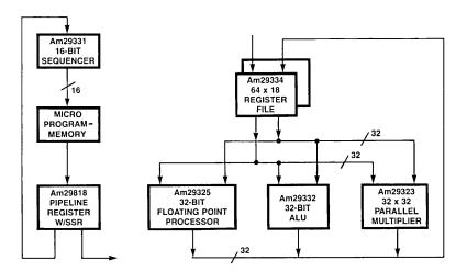
Figure 1. Am29300 Family High Performance System Block Diagram
