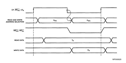
Figure 2. Read through  $Y_A$  and Write through  $D_A$  in a Single Cycle (Two Bytes)
