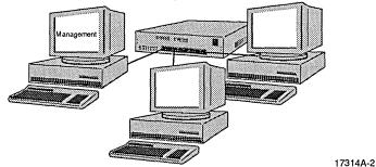
The term "management" means that the repeater supports access to information regarding its operation. Managed 10BASE-T repeaters differ in exactly what information is available, and how that information can be accessed. The recently completed IEEE 802.3 Repeater Management standard defines common sets of information required in managed IEEE 802.3 repeaters.
