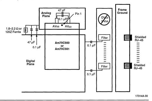
Shielded RJ-45 connectors are recommended. The shield pins should be tied to the frame ground. Depending on the characteristics of the 10BASE-T filters, either the frame ground or a void in the planes should be extended under the filters. Consult the filter manufacturer to determine if the frame ground is needed to minimize the effects of crosstalk within the filters.
