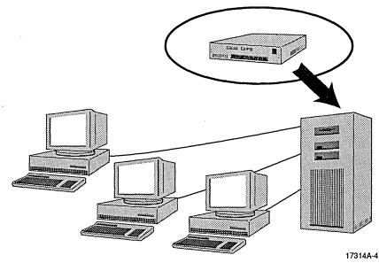
Initially server based repeaters provided only unmanaged capabilities. These products are the equivalent of a fixed configuration dumb repeater. Newer server based repeaters use the capabilities of the server processor to add management support for these products. Novell, Inc. recently introduced the Hub Management Interface (HMI) specification. This specification provides a hardware independent interface between the Novell Netware server management software and the repeater (hub) card.
