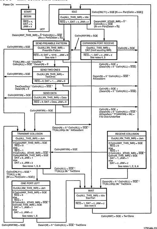
Referring to Figure 3-8, the upper box in each block contains the name of the state. The center box refers to the output at the AUI and TP ports. The lower box describes the state of the REQ, DAT, and JAM output pins for the IMR+ device with this state machine embedded.
