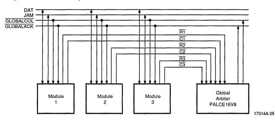
Figure 5-10 Repeater Module with Three IMR+ Devices
