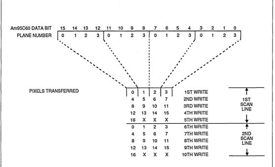
Figure 14-12 Input Block by Pixel for BIS=4 As Seen by Each Am95C60
