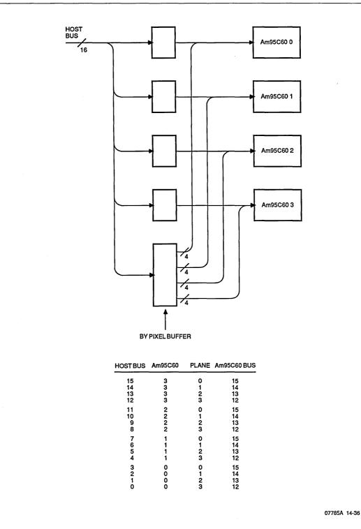
Figure 14-10B Input Block by Pixel for BIS=1 Connections
