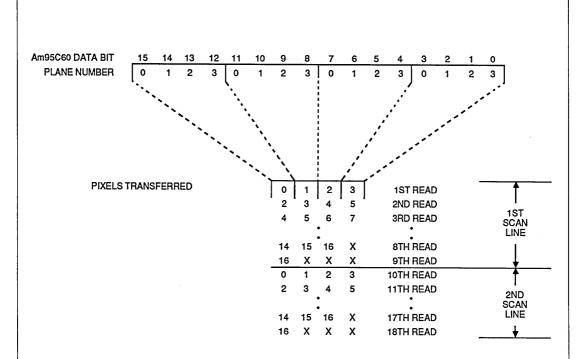
Figure 14-16A Output Block by Pixel for BOS=2 As Seen by Each Am95C60
