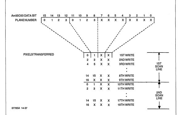
Figure 14-11A Input Block by Pixel for BIS=2 As Seen by Each Am95C60
