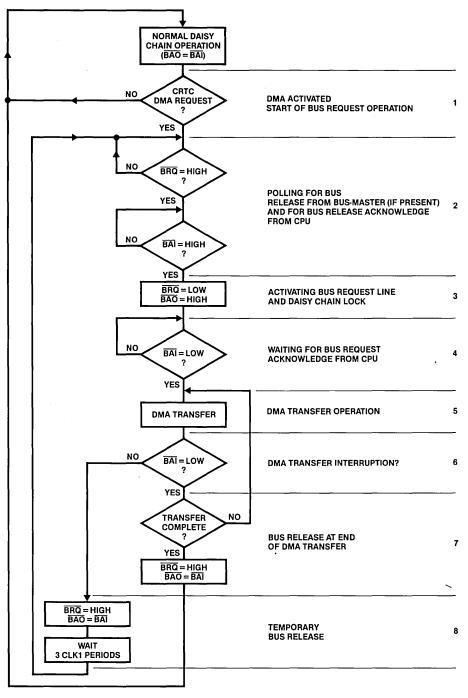
Figure 2.26. DMA Bus Request Flow Chart
