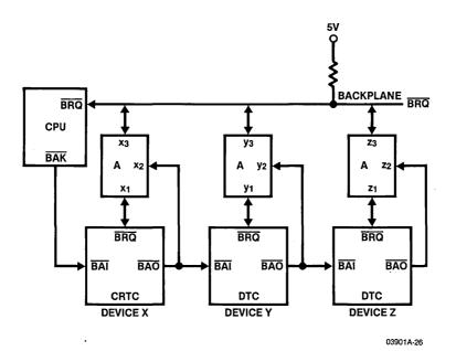
Figure 2.27. System with Multiple DMA Devices
