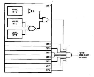
Figure 2.43. Attribute Flag Detect Mechanism
