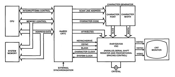
Figure 2.1. CRT Controller System Diagram
