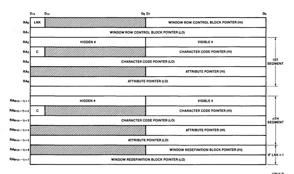
Figure 2.40. Window Row Control Block ( $L/\overline{S} = 1$ )
