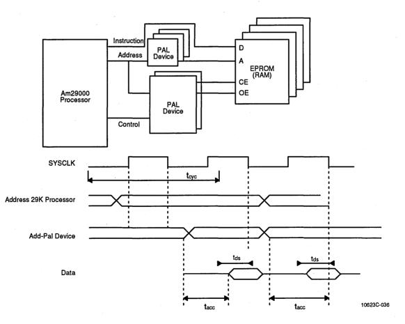
Using memory devices with standard access times, the maximum frequency at which the Am29000 processor can be clocked is:
