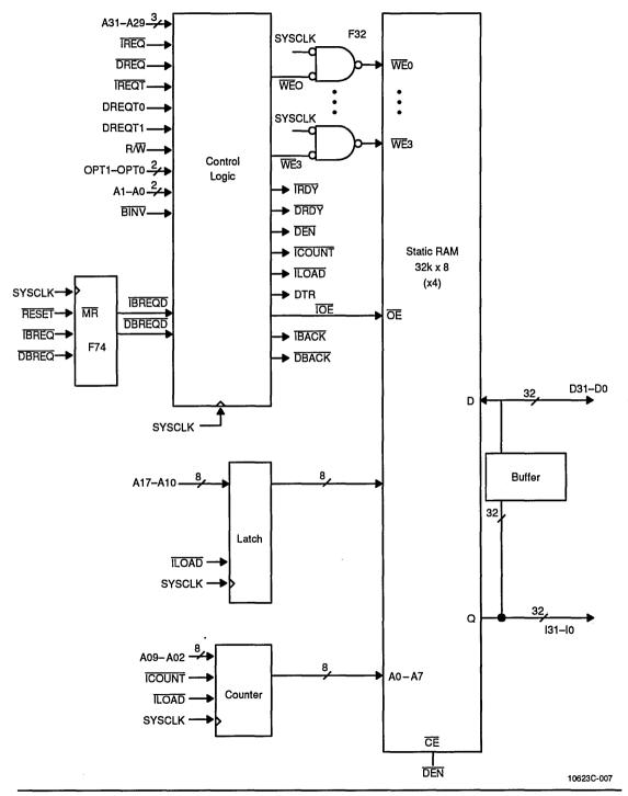
Figure 3-5 Single-Bank SRAM Block Diagram
