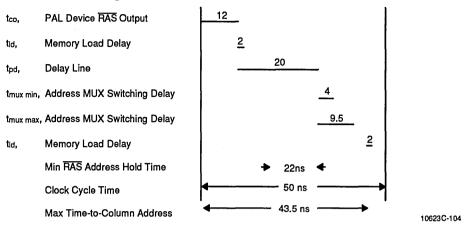
added to the 12-ns delay of the RAS line (standard 50 pF load) for a worst-case total of 14 ns.
