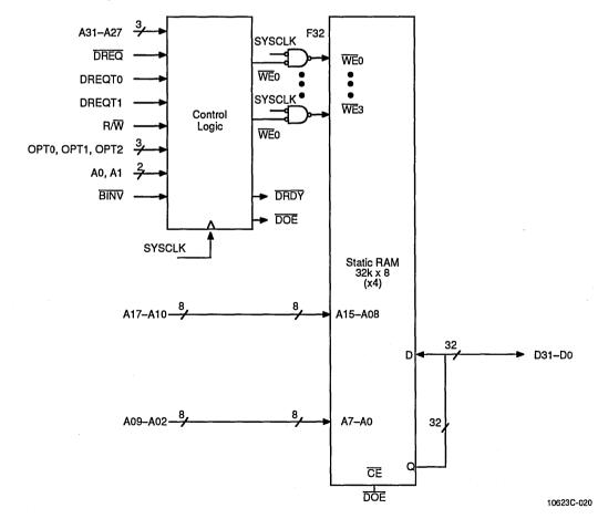
Figure 3-18 Simple Data Access Block Diagram
