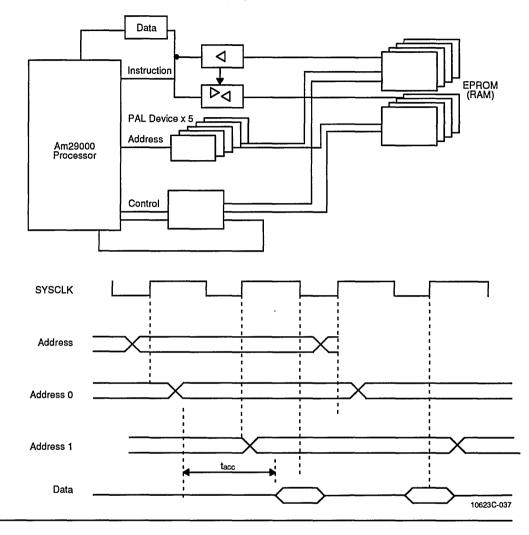
Figure 5-3 Dual-Bank Interleaved Memory System
