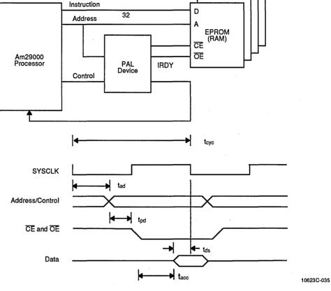
Using memory devices with standard access times, the maximum frequency at which the Am29000 microprocessor can be clocked is:
