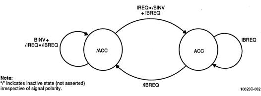
The address counter for the lower eight bits is loaded whenever a valid instruction address is issued by the Am29000 processor. Since single-cycle burst is supported, it is incremented on every clock while ACC is active.
