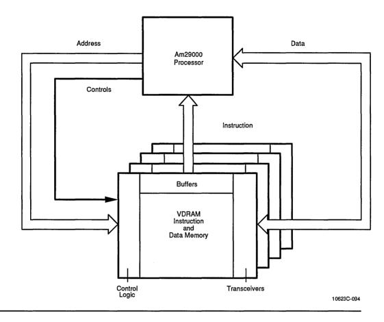
Figure 10-1 Am29000 Processor with VDRAM Memory
