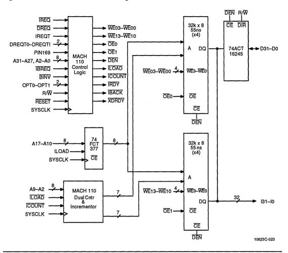
Figure 3-21 Interleaved SRAM Block Diagram
