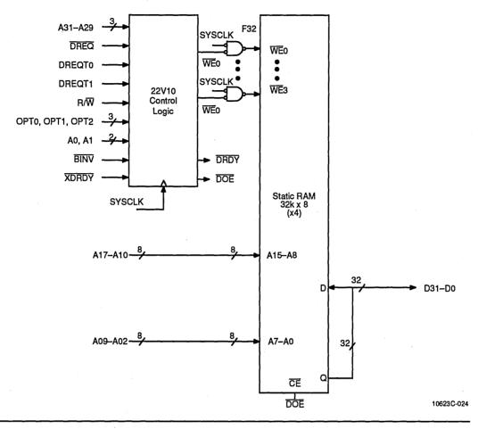
Figure 3-22 Simple Data Access Block Diagram
