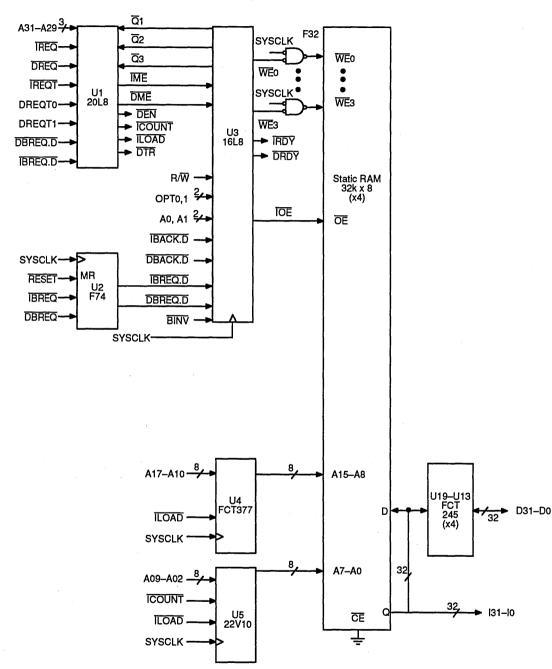
Figure 3-23 Single-Bank SRAM Block Diagram
