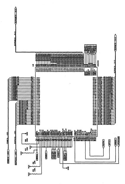
Figure 6-6 Low-Cost Am29000 Processor Design (continued)
