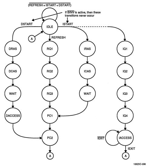
The active states can be thought of as two tokens, labeled SD and DQ, being moved around a game board. The DQ token is never allowed to follow the dotted line to the virtual states. The SD token is always in one of the virtual states or the IDLE state; it never enters any of the other states. When the SD token enters the IDLE state, it cannot leave until the DQ token is also in IDLE and the ISTART condition is true.
