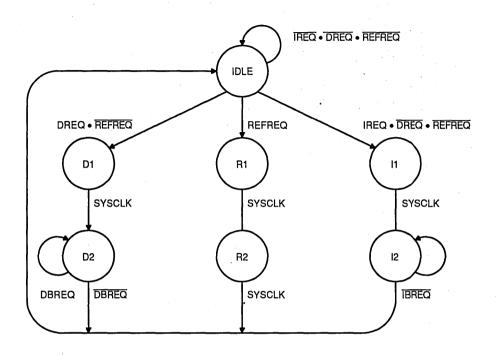
then it is a two-cycle access.  $\overrightarrow{DREQ}$  with OPT2 = 1 is for the ADAPT29K to access PROM as data. PIN169 will be High for this type of load, but for other ADAPT29K loads and stores, PIN169 will be Low. Pin 169 is then used by the state machine to hold in the IDLE state.
