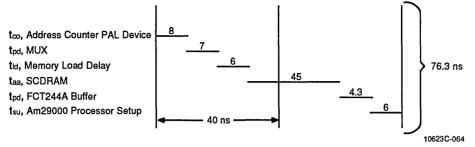
This works out to satisfy the 15 ns of required hold time of address after RAS goes active. Also, the column address is settled by 40 ns into the cycle.
