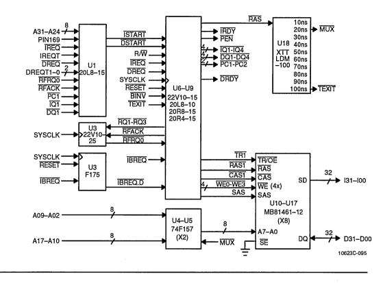
Figure 10-2 Single-Bank VDRAM Memory Block Diagram
