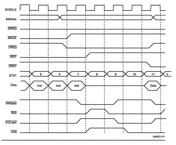
Figure 8-7 Instruction Burst Pre-empted by a Data Access
