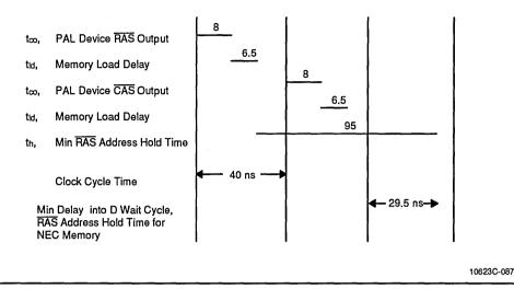
Assuming minimum delays in the TR and SAS signals and maximum delays in the RAS signals, the hold time for TR will just be met for either the NEC or Fujitsu memories. For the Fujitsu memory, the TR setup time before SAS will also just be met as shown in Figure 9-16. For the NEC memory there is 5 ns of margin as shown in Figure 9-17.
