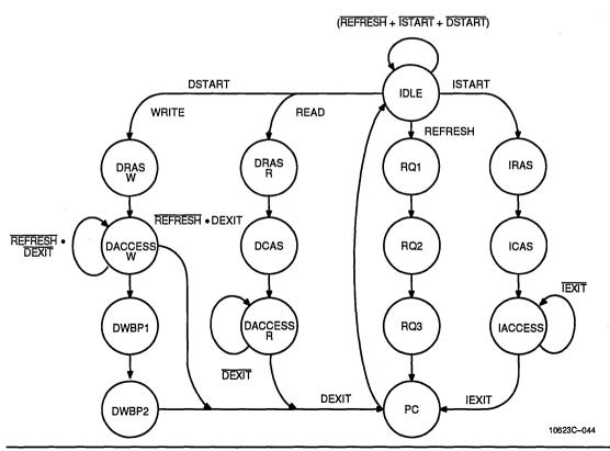
used as the input to a delay line whose output will switch the address mux to the column address after the row address hold time is satisfied. The transition to the Instruction Column Address Strobe (ICAS) state is unconditional.
