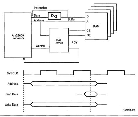
commencement of the next. For example, to fill half the contents of the register file (i.e., perform 64 LOADs) 191 clocks would be required rather than 128 as first thought. This is a loss of 30% (worst case) of the available data bus bandwidth. This performance impact would only be seen on programs performing many multiple LOADs and STOREs.
