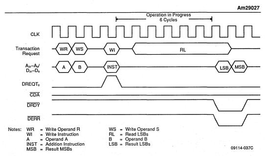
Signals A<sub>31</sub>-A<sub>9</sub> and D<sub>31</sub>-D<sub>9</sub> are the Am29000 address and data buses, respectively.
