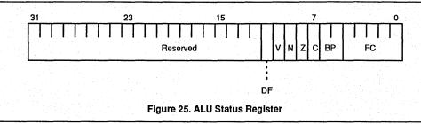
Bit 10: Overflow (V)—The V bit indicates that the result of a signed, twos-complement ALU operation required more than 32 bits to represent the result correctly. The value of this bit is determined by exclusive ORing the ALU carry-out with the carry-in to the most-significant bit for signed, twos-complement operations. This bit is not used for any special purpose in the processor, and is provided for information only.
