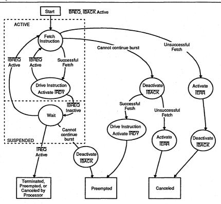
Note: A similar state transition may be used to support suspended burst-mode data accesses or a channel master other than the processor.
