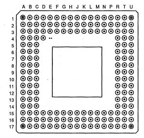
\* Pinout observed from pin side of package. \*\*Alignment pin (not connected internally).
