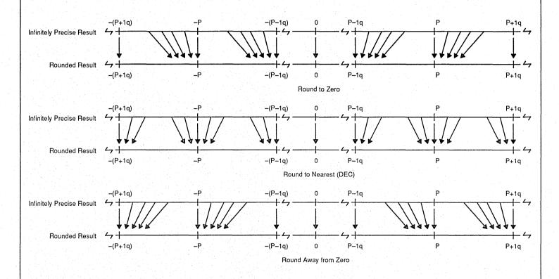
Figure B2. Graphical Interpretation of Round-to-Zero, Round-to-Nearest (DEC), and Round-Away-from-Zero Rounding Modes
