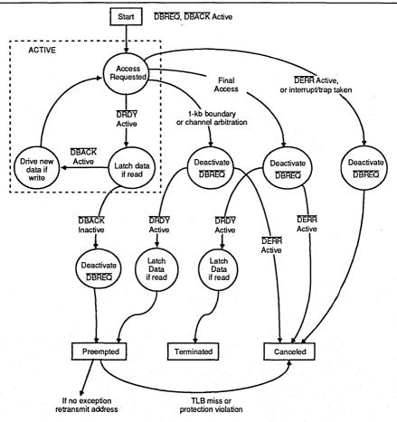
Note: The Am29000 does not suspend burst-mode data accesses.
