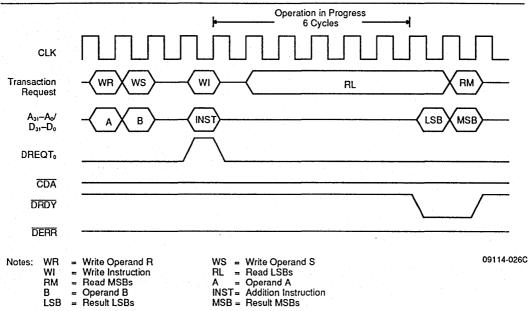
Signals A<sub>31</sub>-A<sub>0</sub> and D<sub>31</sub>-D<sub>0</sub> are the Am29000 address and data buses, respectively.
