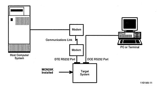
Figure 11. MON29K System Connections
