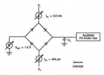
$\rm C_L$  is guaranteed to 80 pF. For capacitive loading greater than 80 pF, refer to the Capacitive Output Delay table.
