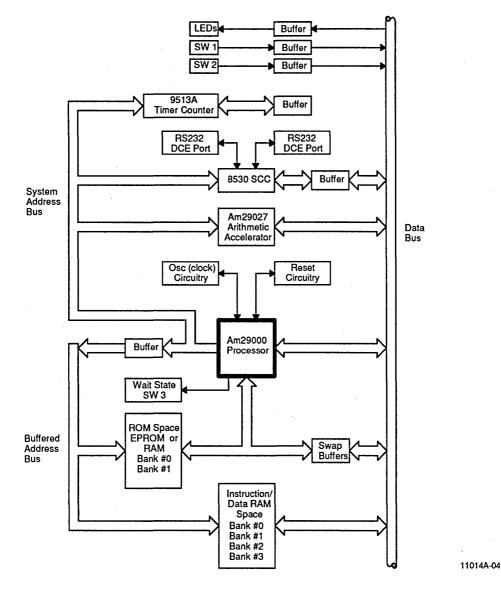
Figure 4. Block Diagram of the STEB
