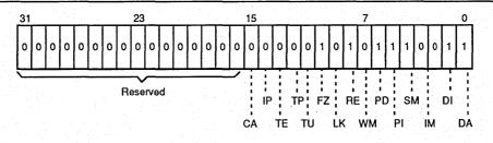
Figure 67. Current Processor Status Register In Reset Mode
