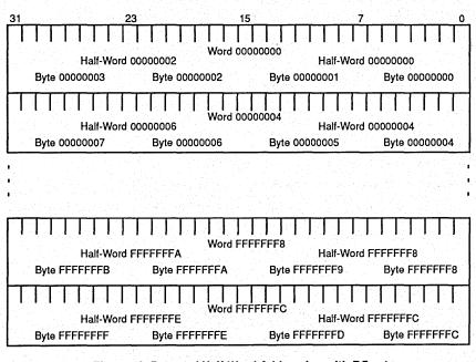
Figure 52. Byte and Half-Word Addressing with BO = 1
