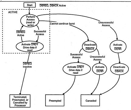
Figure 66. Slave Burst-Mode Data Accesses: Control Flow
