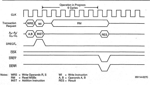
Signals A31-A0 and D31-D0 are the Am29000 address and data buses, respectively.
