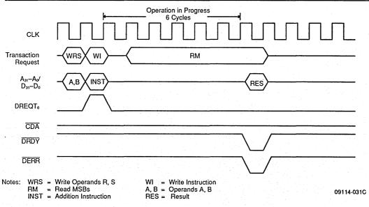
Signals A<sub>31</sub>-A<sub>0</sub> and D<sub>31</sub>-D<sub>0</sub> are the Am29000 address and data buses, respectively.
