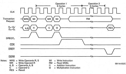
Signals  $A_{31}\text{-}A_0$  and  $D_{31}\text{-}D_0$  are the Am29000 address and data buses, respectively.
