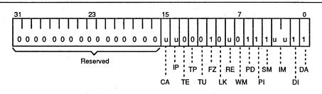
Figure 55. Current Processor Status after an Interrupt or Trap
