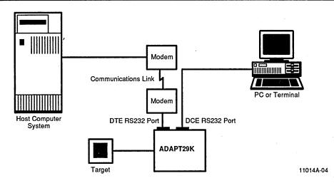
Figure 4. Connections to the ADAPT29K
