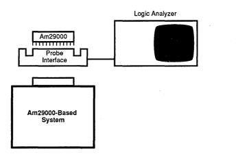
Figure 16. Connection of the Probe Interface
