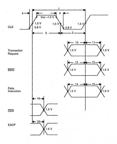
Input Signal Timing; CDA, EXCP Timing
