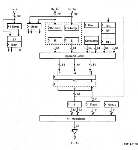
Figure 16. Programmer's Model for Pipeline Mode
