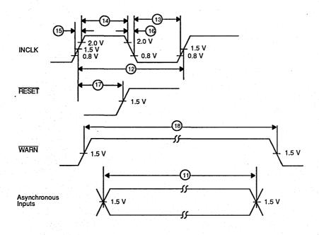
**INCLK and Asynchronous Inputs**
