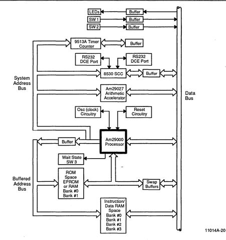
Figure 20. Block Diagram of the STEB
