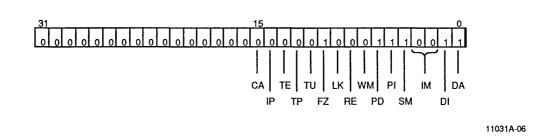
Figure 6. Current Processor Status Register After an Interrupt or Trap
