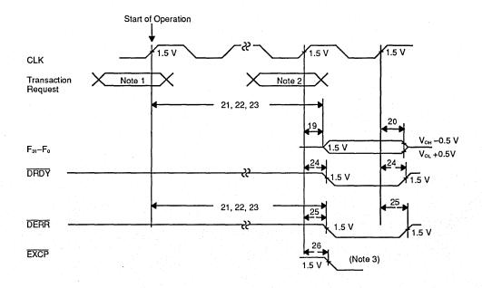
Operation Timing for Flow-Through Mode, DRDY, DERR Advanced (Mode Register Bit AD=1)
