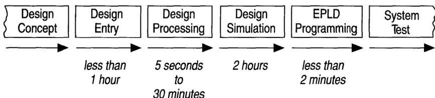
design entry to device programming in a matter of hours. Design processing is typically completed in minutes, allowing several design iterations to be completed in a single day.
