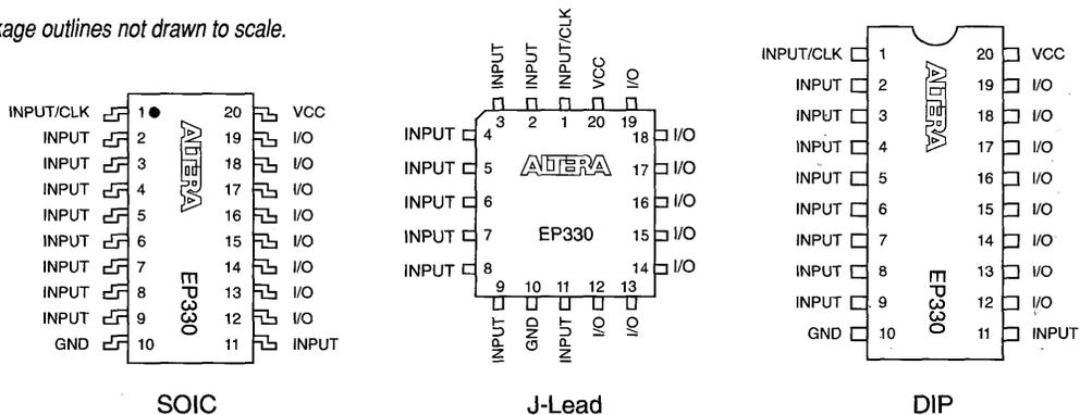
The EP330 EPLD can accommodate up to 18 inputs and 8 outputs. Each of the 8 macrocells contains a programmable-AND/fixed-OR structure that implements logic with up to 8 product terms. An additional product term in each macrocell controls Output Enable.
