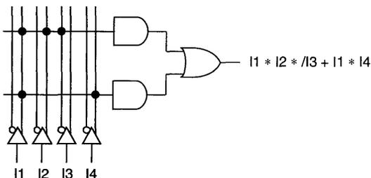
The  $2 \times 8$  AND-array of Circuit C can produce any Boolean function of four variables (provided only two product terms are required) when expressed in sum-of-products form. Any Boolean expression—no matter how complex—can be written in sum-of-products form. Outputs of the two AND gates in Figure 5 are called product terms (or p-terms).
