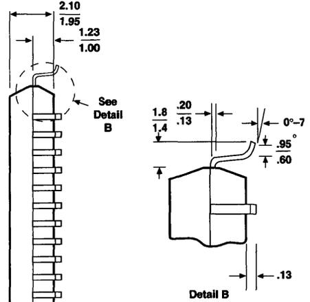
68-Pin Ceramic J-Lead Chip Carrier (JLCC)
