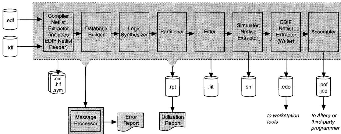
Compiler options simplify design processing and analysis. The user can specify up to two LMFs for the Compiler to use in processing EDIF Input Files (.edf), and can choose to create an EDIF Output File (.edo) for use with Valid Logic, Viewlogic, or other third-party simulation tools. Other options specify the degree of detail of the Report File (.rpt) that shows how EPLDs have been utilized and the target EPLD for the design.
