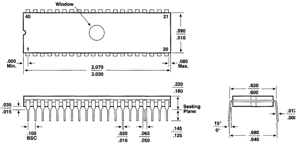
**40-Pin Plastic Dual In-Line Package (PDIP)**
