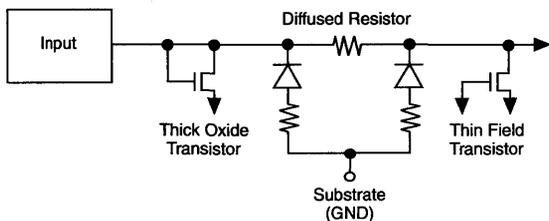
Altera components include special structures that reduce the effects of ESD at the pins. Figure 15 shows a typical input structure. Diode structures as well as specialized field-effect transistors shunt harmful voltages to ground before destructive currents will flow. Altera EPLDs typically withstand ESD voltages >2 kV, and are thus safe under normal handling conditions.
