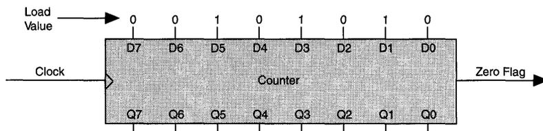
The CREG is loaded or decremented on the leading edge of the clock. It will not decrement once it reaches zero, thereby preventing roll-over. A zero flag indicates when the counter has reached zero. This flag is used with the LOOPNZ command to control program flow. (See "Instruction Set" later in this data sheet.) Single-instruction delay loops are easily constructed, and nested loops or delays of arbitrary length may be generated in combination with the stack.
