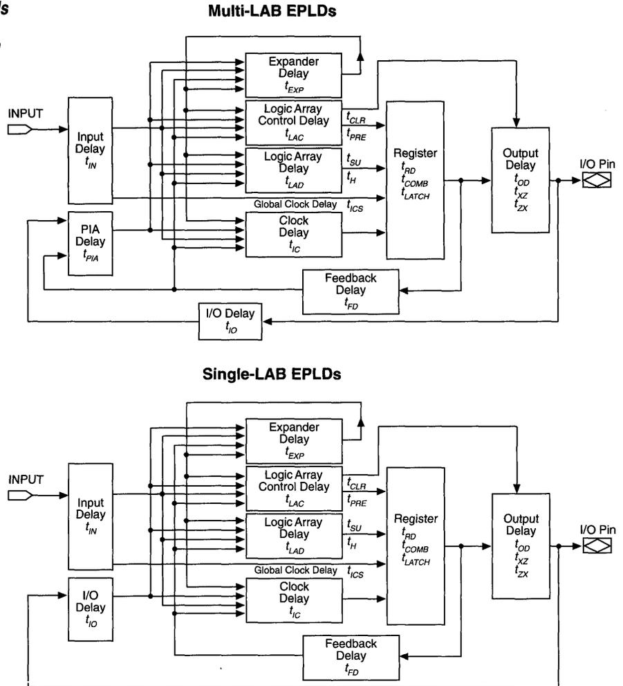
The timing models shown in Figure 6 can be used together with the internal timing parameters for a particular EPLD to derive timing information. External timing parameters are derived from a sum of internal parameters and represent pin-to-pin timing delays. Figure 7 shows the internal timing waveforms for these devices. Refer to *Application Brief 75* for further information on MAX 5000 EPLD timing.
