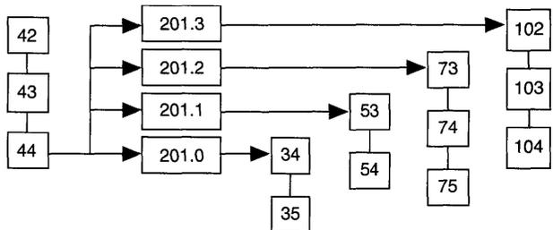
Any of the 13 available commands can be enhanced with multiway branching. For example, location 44 in Figure 10 can be a `CALL` to a subroutine, and address 201 can contain the starting instruction for 4 unique subroutines. The routine that is actually executed depends on the user-defined condition of the inputs. The following ASM code can be used to implement this example:
