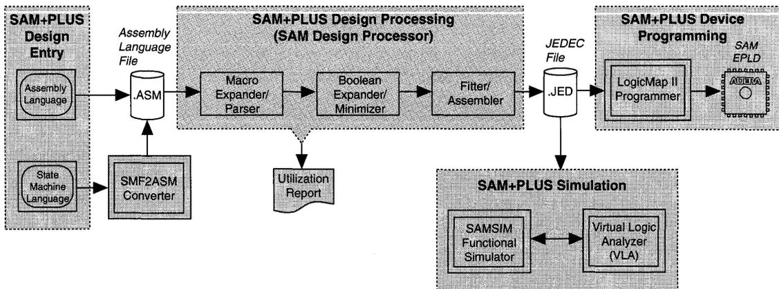
Horizontal cascading (i.e., using multiple EPS448 EPLDs to increase the number of outputs) is fully supported in design entry, processing, simulation, and programming. Multiple EPS448 EPLDs are listed in a single source file, but separate report and JEDEC Files are created for each device.
