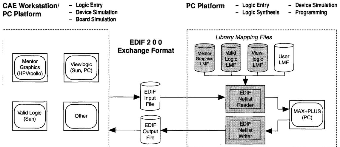
PLS-EDIF (Bidirectional EDIF Netlist Interface to MAX+PLUS Software) allows designers to enter and verify logic designs for Altera MAX 5000 EPLDs with third-party CAE tools. The EDIF 2 0 0 netlist exchange format provides a two-way bridge between MAX+PLUS and third-party schematic capture and simulation tools. PLS-EDIF runs on an IBM PS/2, PC-AT, or compatible computer.
