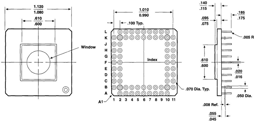
84-Pin Ceramic J-Lead Chip Carrier (JLCC)
