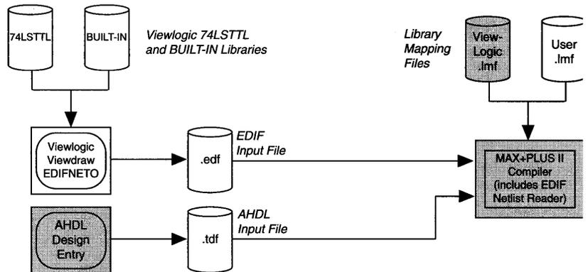
compiled. Symbols from the Valid Logic LSTTL library can be mapped to corresponding primitive and TTL functions in the MAX+PLUS II TTL MacroFunction Library with the Altera-provided Library Mapping File (.lmf) for Valid Logic users. Table 1 shows the primitive mappings and Table 3 shows the macrofunction mappings provided in this LMF.
