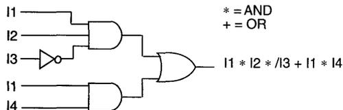
Circuit B: Circuit A drawn with complementary output buffers
