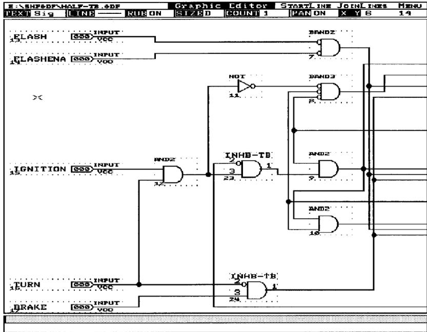
Figure 9. Schematic Converted and Annotated with SNF2GDF
