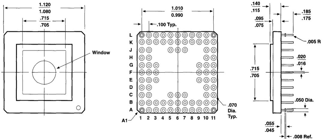
100-Pin Ceramic Pin-Grid Array (PGA)
