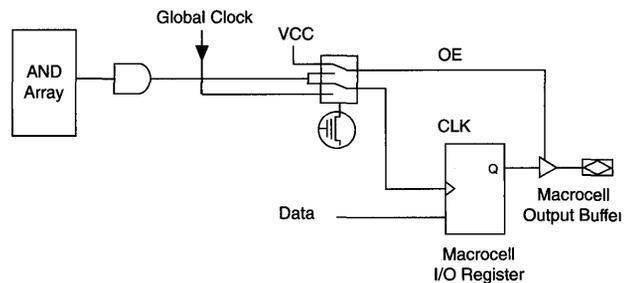
In Mode 0, the tri-state output buffer is controlled by a single product term. If the output of the AND gate is high, the output buffer is enabled. If the output is low, the output buffer has a high-impedance value. In this mode the macrocell flip-flop is clocked by its global Clock input signal (CLK1 or CLK2). In the erased state, the OE/CLK Select multiplexer is configured to Mode 0.
