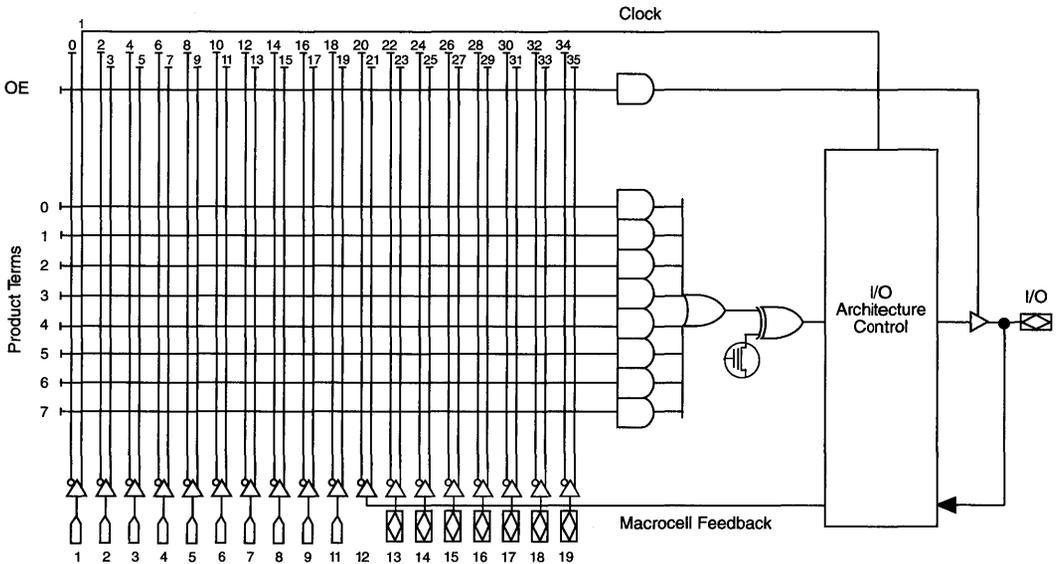
The EP330 block diagram is shown in Figure 4. The internal architecture of this device has a sum-of-products (AND/OR) structure. Inputs to the programmable-AND array come from the true and complement signals of the 10 dedicated input pins, and the true and complement forms of the 8 feedback signals from the I/O architecture control blocks. The 36-input AND array has 72 product terms distributed equally among the 8 macrocells. Each product term represents a 36-input AND gate.
