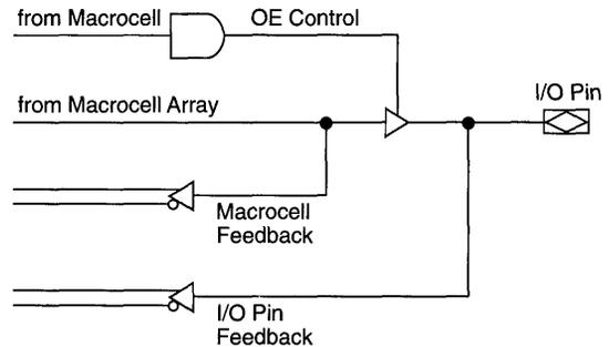
Each MAX 5000 EPLD has dual feedback—a feedback path both before and after the tri-state buffer—for every I/O pin. The tri-state buffer decouples the I/O pins from the macrocells so that all registers within the LAB can be “buried.” Thus, I/O pins can be configured as dedicated input, output, or bidirectional pins. In multi-LAB devices, I/O pins feed the PIA.
