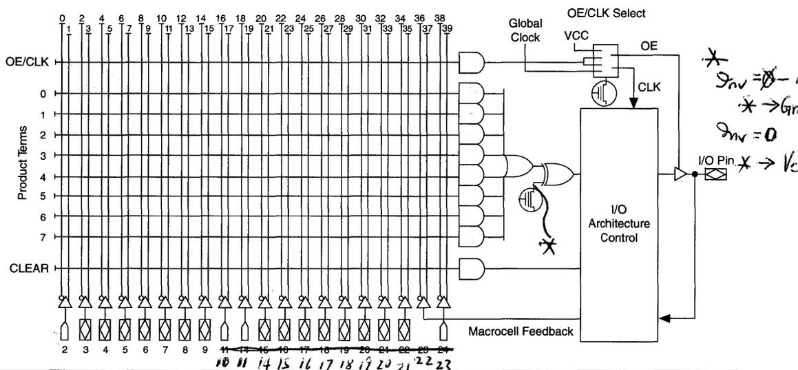
Figure 2 shows the complete block diagram of an EP610 EPLD. The internal device architecture has a sum-of-products (AND/OR) structure. Inputs to the programmable-AND array come from the true and complement signals of the 4 dedicated data inputs and 16 I/O feedback signals. The 40-input AND array has 160 product terms distributed among the 16 macrocells. Each product term represents a 40-input AND gate.
