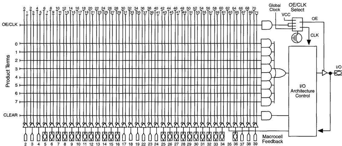
Figure 2 shows the block diagram of an EP910 EPLD. The internal device architecture has a sum-of-products (AND-OR) structure. Inputs to the programmable-AND array come from the true and complement signals of the 12 dedicated data inputs and the 24 I/O feedback signals. The 72-input AND array has 240 product terms that are distributed equally among the 24 macrocells. Each EP910 product term represents a 72-input AND gate.
