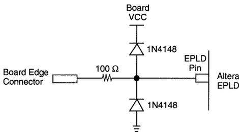
In some applications, boards are “hot-socketed” in the field. The circuitry shown in Figure 14 is recommended to ensure that latch-up-inducing levels are not applied to the EPLD under these conditions. Normally, this circuitry is required only if the EPLD has inputs tied directly to the edge connector. The diodes clamp the inputs at acceptable levels and the series resistor further limits the injection of current into the EPLD input and clamp diodes. This interface provides maximum protection.
