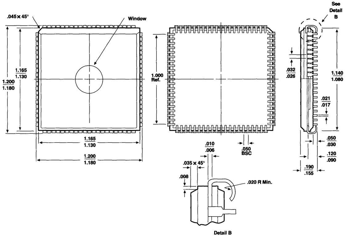
34-Pin Plastic J-Lead Chip Carrier (PLCC)
