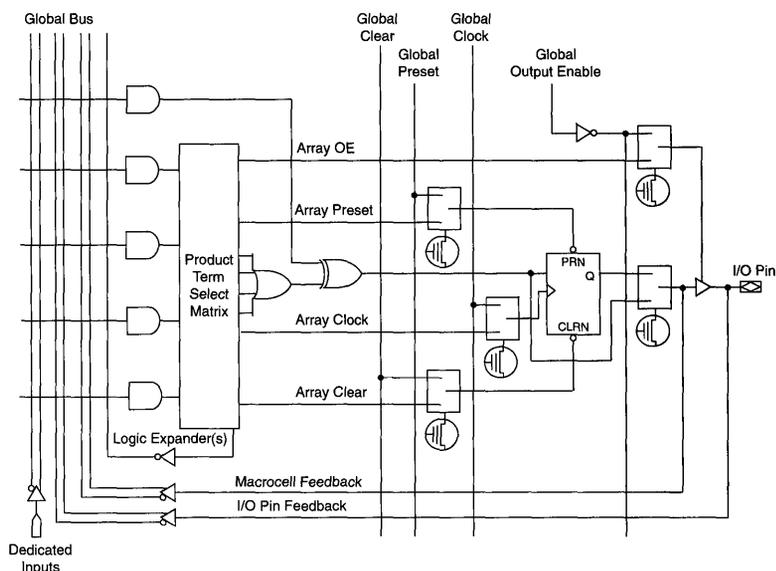
Combinatorial logic is implemented in the product-term array, which consists of five product terms. Four product terms feed the product-term select matrix, and the fifth feeds one input of an XOR gate, making it possible to implement active-high or active-low logic. The XOR gate is also used to build complex arithmetic logic functions and for De Morgan's inversion to reduce the number of product terms required for a design.
