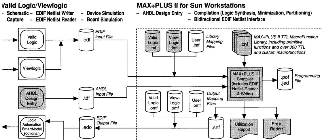
support, advanced logic synthesis, and design fitting in the Sun computer environment. Together, MAX+PLUS II and Valid Logic or Viewlogic software provide the tools to quickly and efficiently create, compile, and verify logic designs for Classic, MAX 5000, MAX 7000, and STG EPLDs.
