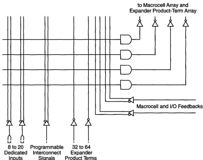
Expanders are fed by all signals in the LAB. One expander may feed all macrocells in the LAB or multiple product terms in the same macrocell. Since expanders also feed the secondary product terms of each macrocell, complex logic functions can be implemented without using additional macrocells. Expanders can also be cross-coupled to build additional flip-flops or latches.
