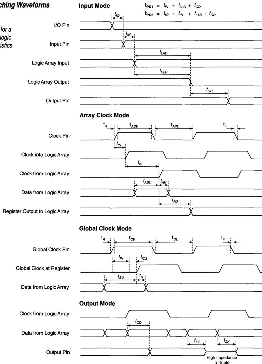
Figure 5. EP1810 Timing Model
