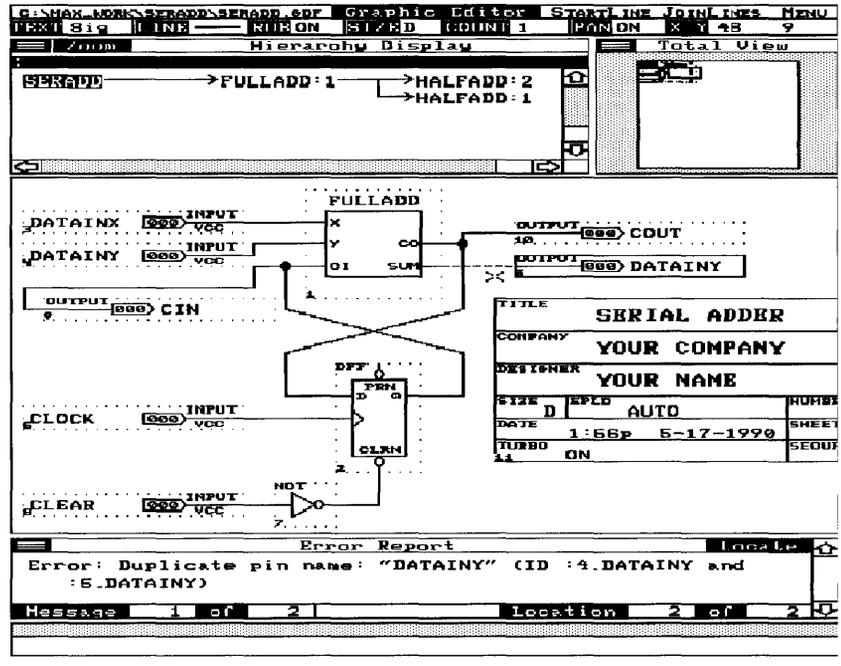
View window shows the entire design. By clicking inside this window, the main work window is moved to the corresponding area of the schematic. The Error Report window lists all warnings and errors in the compiled design; selecting an error with the mouse highlights the problem node and symbol. A design is entered in the main work window, which can be enlarged by closing the auxiliary windows.
