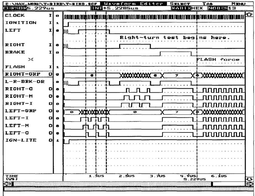
up to 32 signals that are represented in binary, octal, decimal, or hexadecimal format. Logical operators can also be used on pairs of waveforms, so that waveforms can be inverted, ORed, ANDed, or XORed.
