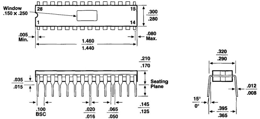
28-Pin Plastic Dual In-Line Package (PDIP)
