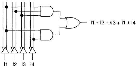
Circuit C: Circuit B with 8-input AND gates in AND-array notation
