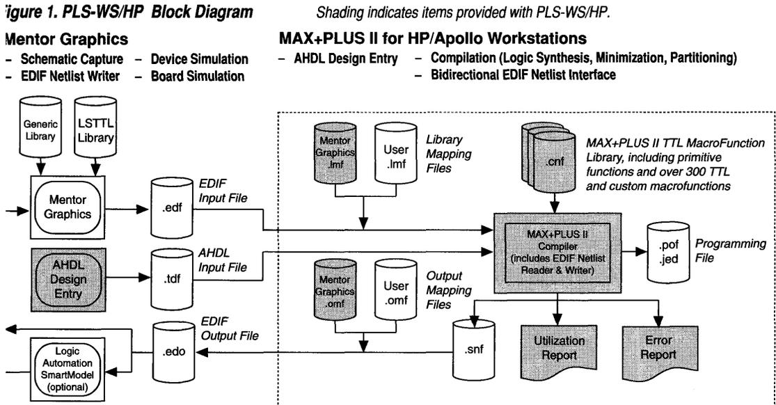
Description Language (AHDL) design entry, bidirectional EDIF netlist interface, Mentor Graphics library support, advanced logic synthesis, automatic partitioning, and design fitting in the HP/Apollo computer environment. Together, MAX+PLUS II and Mentor Graphics software provide the tools to quickly and efficiently create, compile, and verify logic designs for Classic, MAX 5000, MAX 7000, and STG EPLDs.
