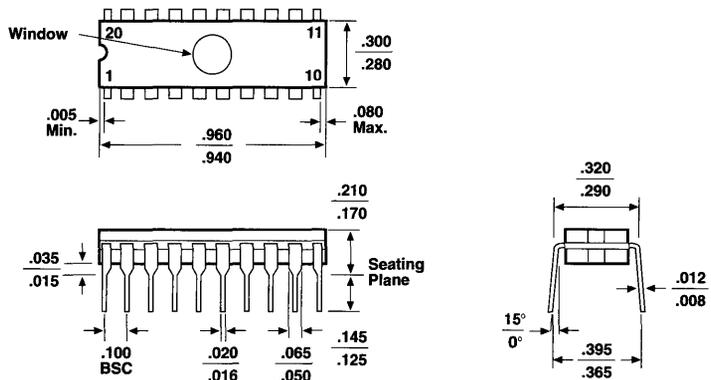
20-Pin Plastic Dual In-Line Package (PDIP)
