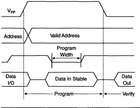
1. The programming pin ( $V_{PP}$ ) is raised to the super-high-input level (nominally 12.5 V).
