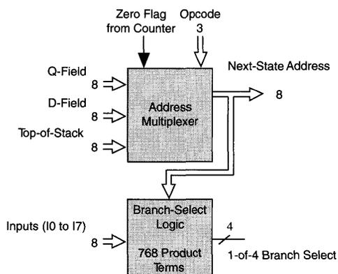
The address multiplexer provides the next-state address to the microcode memory. The next-state address can come from the Q-field, the D-field, or the top-of-stack. The selection is based on the instruction in the pipeline register and the condition of the zero flag from the counter.
