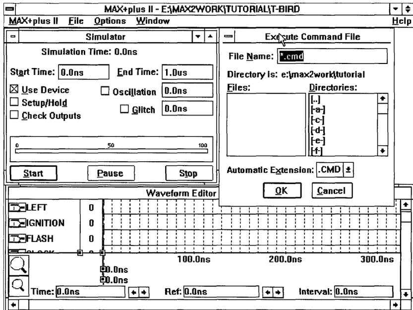
during simulation, the Message Processor can locate the offending node in the original design file, and display the time at which the problem took place in the Waveform Editor.
