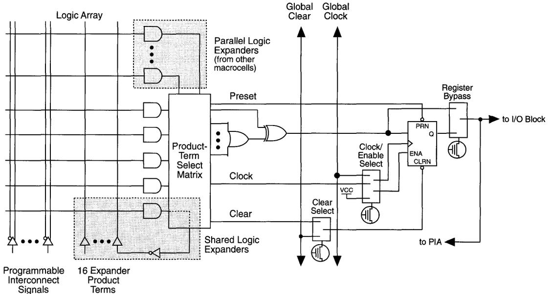
secondary inputs for either an additional XOR input or individual Clear, Preset, Clock, and Clock Enable logic functions for the flip-flops; or as logic expanders to assist the generation of complex logic functions.
