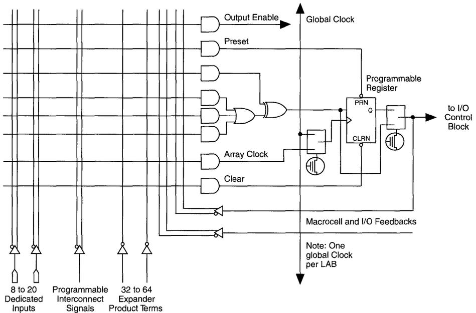
eliminating inefficient, unused product terms. Also, expanders can be allocated to enhance the capability of the logic array.
