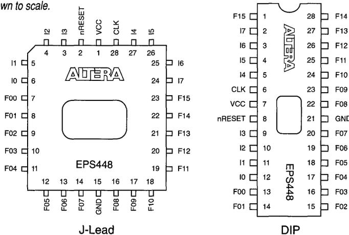
The on-chip EPROM of each EPS448 device (up to 448 words) is integrated with branch-control logic, a pipeline register, a stack, and a loop counter. This generic microcoded architecture can efficiently implement a broad range of high-performance controllers, from state machines to waveform-generation applications.
