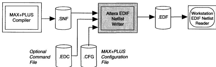
The EDIF output file may have one of two formats. The first format expresses all delays with special EDIF property constructs. The second expresses combinatorial delays with port-delay constructs and registered delays with path-delay constructs—a format that is especially useful for behavioral simulators. Figure 5 shows an example in both formats.
