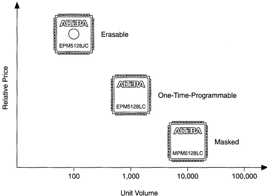
The EPLD-to-MPLD conversion is handled by Altera so that no redesign effort is required. Altera guarantees that the MPLD meets the worst-case AC and DC parameters of the original EPLD design. In addition, Altera automatically generates test vectors with over 95% fault coverage.
