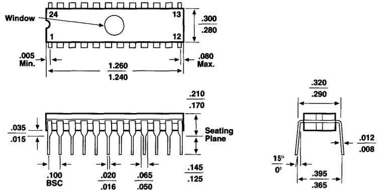
**24-Pin Plastic Dual In-Line Package (PDIP)**
