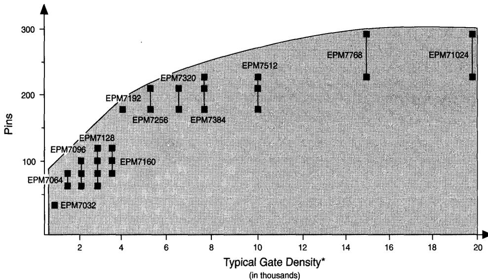
\* Typical gate density is 50% of maximum gate density.
