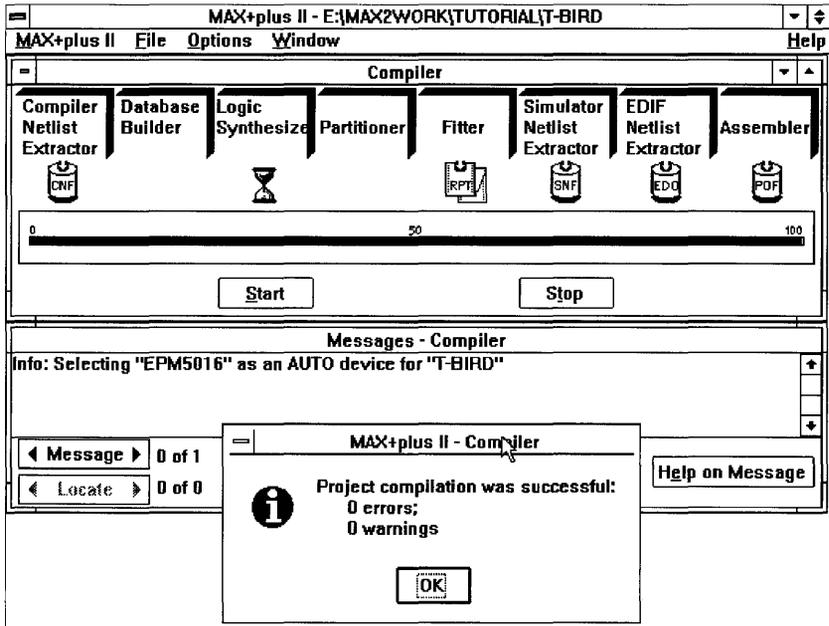
factor and map logic within the chosen EPLD structure. It then uses advanced synthesis algorithms that ensure the most efficient use of silicon resources.
