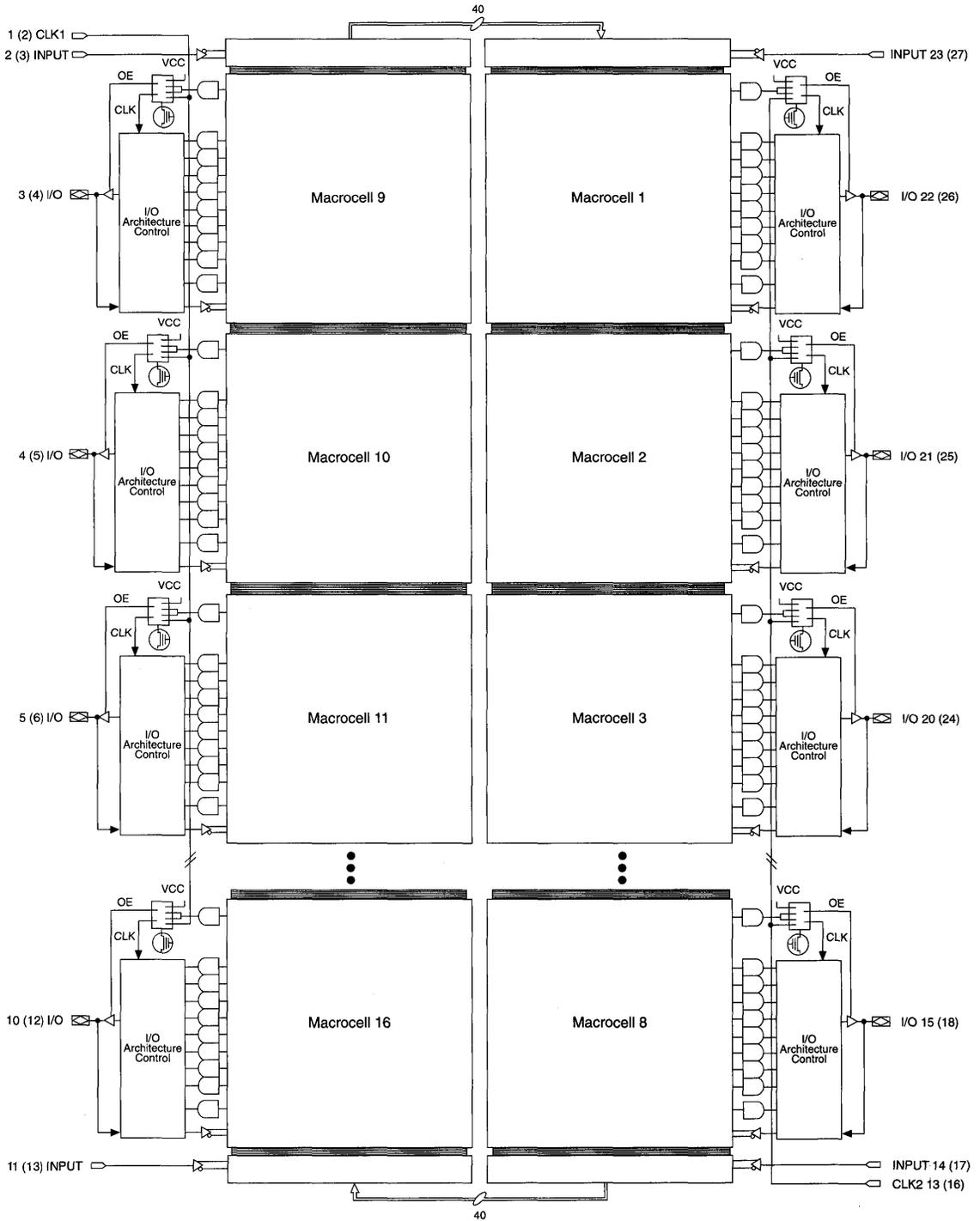
In the erased state, the true and complement of the AND-array inputs are connected to the product terms. An EPROM control cell is located at each intersection of an AND-array input and a product term. During programming, selected connections are opened, allowing any product term to be connected to a true or complement array input signal with the following results:
