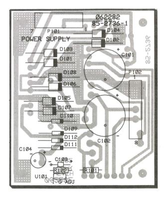
**POWER SUPPLY CIRCUIT BOARD** (Assembled part number HE 181-3887)
