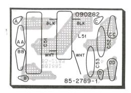
**RF TRAP CIRCUIT BOARD** (Assembled part number HE 181-4325)
