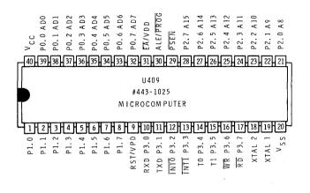
The clear to send (CTS) and data terminal ready (DTR) control signals (handshaking) on the computer port (DTE) are taken directly from the microcomputer and passed to the line drivers. On the auxiliary port the clear to send (CTS), data terminal ready (DTR), data set ready (DSR), and the received line signal detect (RLSD) signals are all tied together.
