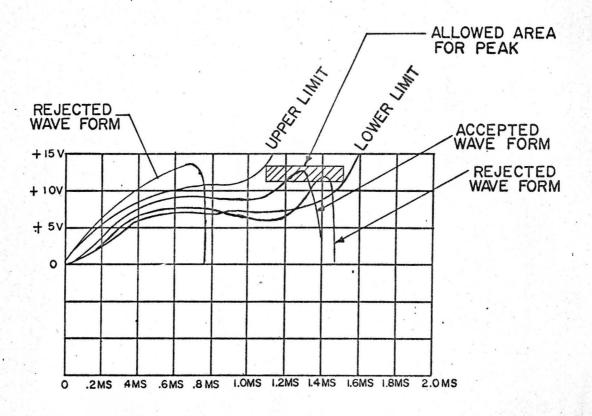
(OSCILLOSCOPE GRID) HORIZ = .2 MS/CM VERT = 5 V/CM
