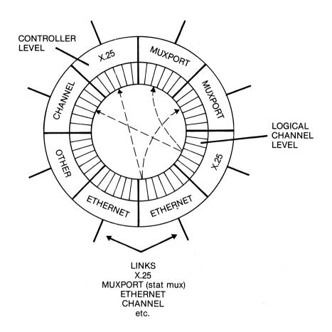
The diagram below illustrates how the onion skin structure in the TelePAC model maps on to the OSI reference model, when a cross section of the onion skin layers is taken. The diagram also shows how the proposed extensions to the TelePAC interfaces map on to the TelePAC and OSI model.
