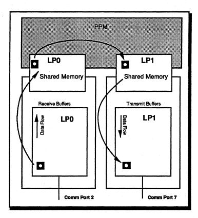
Figure 2-2 Typical LP Data Flow
