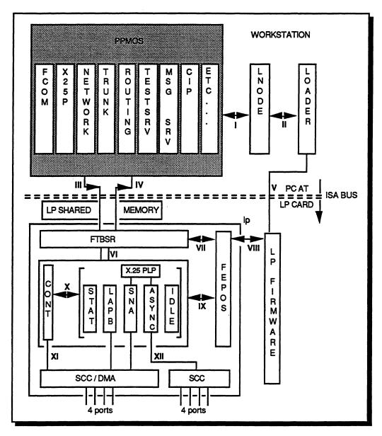
Figure D-1 Standard LP Port Interface
