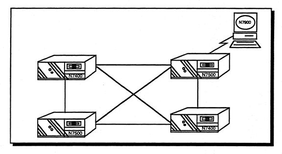
Figure 1-5 Typical Backbone Network
