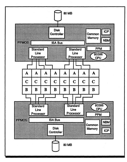
Figure 6-1 Hot Standby Switch
