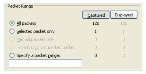
If the **Captured** button is set (default), all packets from the selected rule will be processed. If the **Displayed** button is set, only the currently displayed packets are taken into account to the selected rule.
